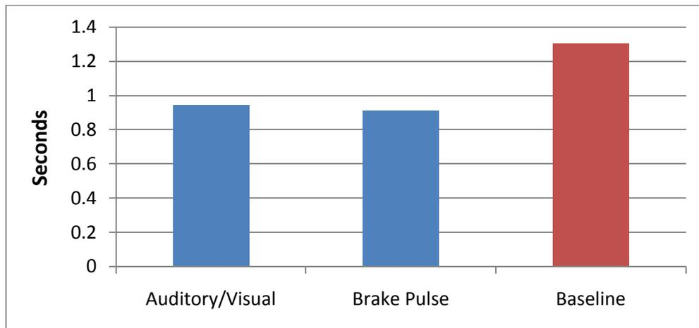
**Figure 13. Brake response times for FCW systems**
