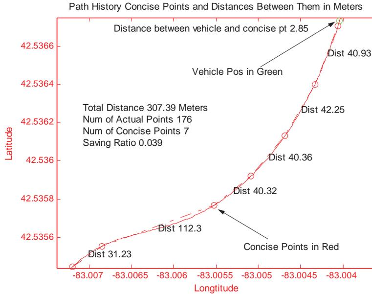
Figure 15: Method One – PH Representation of Curved Road
