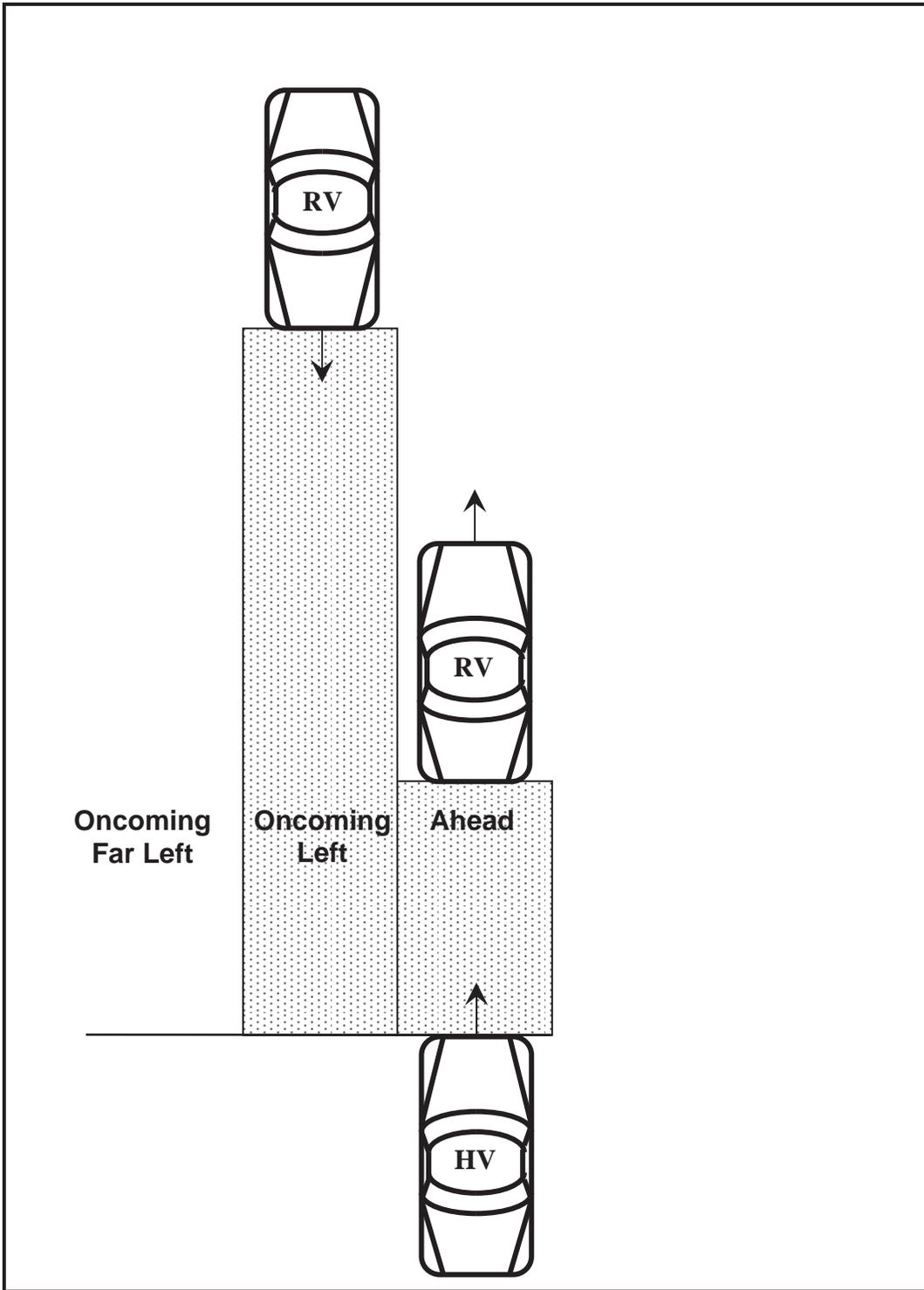
Figure 7: DNPW Target Classification Zones
