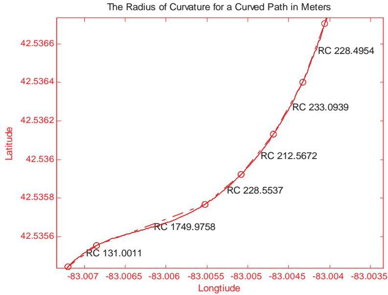
Figure 11: Method One and Three – Radii of Curvature for Curved Road
