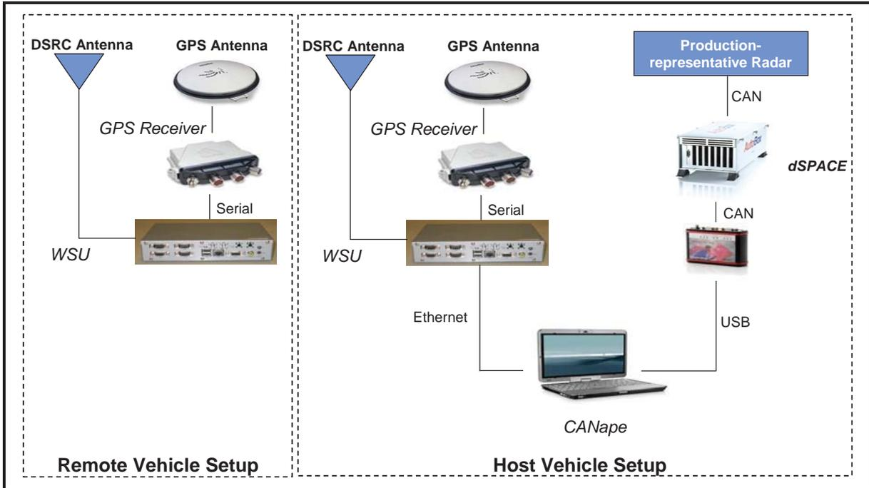
Figure 1: DSRC and Autonomous Sensing Safety System Analysis Setup
