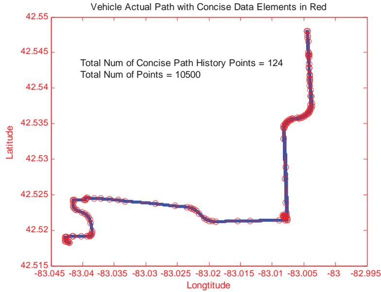
**Figure 10: Method Three – Representation of Vehicle Path**
