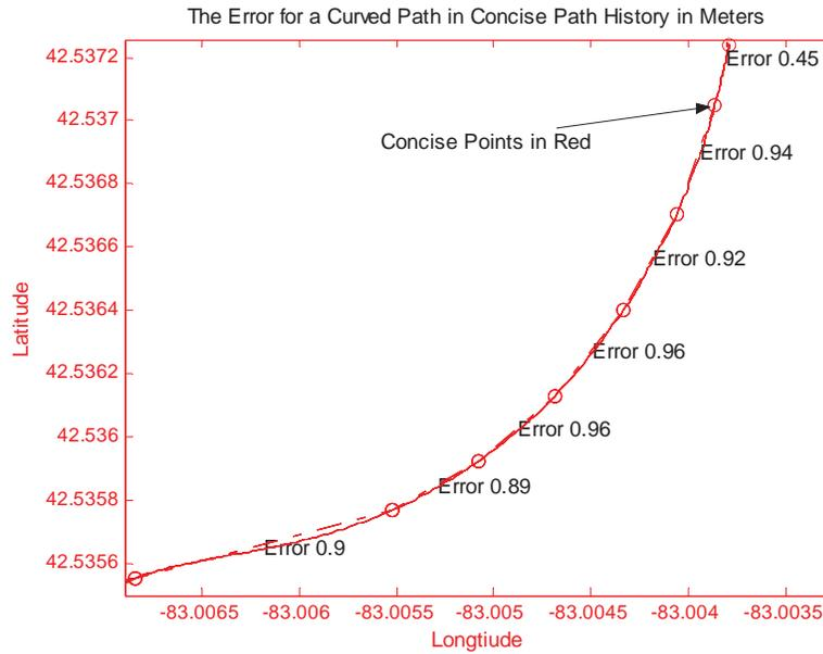
Figure 21: Method One – PH Error Analysis
