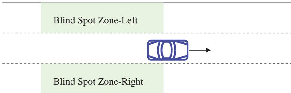
**Figure 3: Vehicle Blind Spot Zone Definition**
