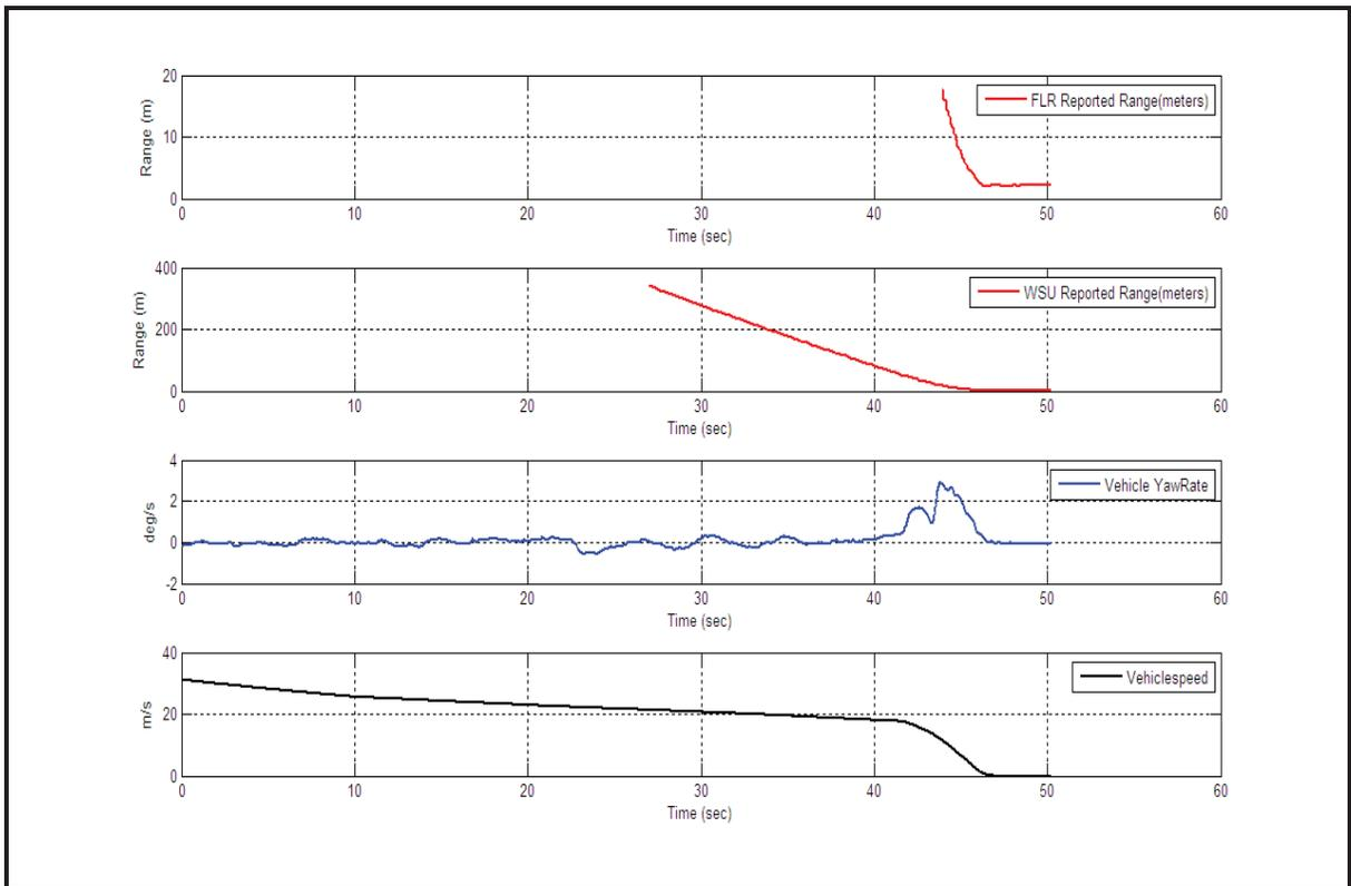
Figure 6: Sensor Performance During Detection of a Stationary Vehicle in a Curve
