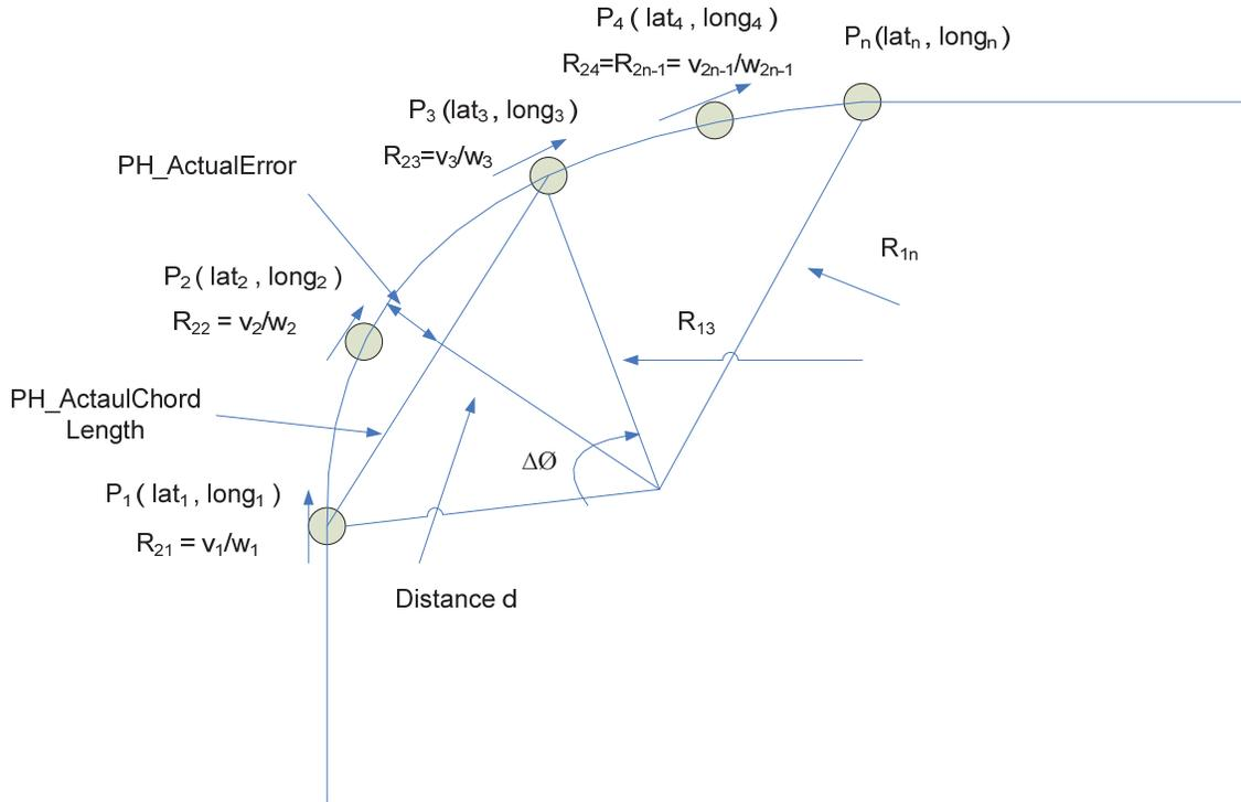
**Figure 4: Representation of Estimated Radius Calculation**
