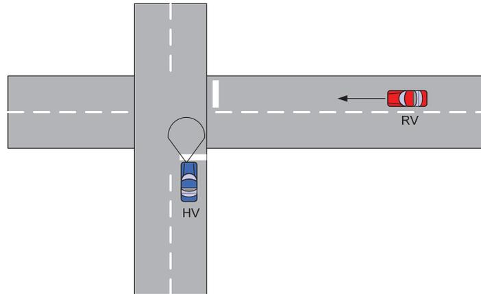
Figure 13: Detecting and Tracking Intersecting Vehicles
