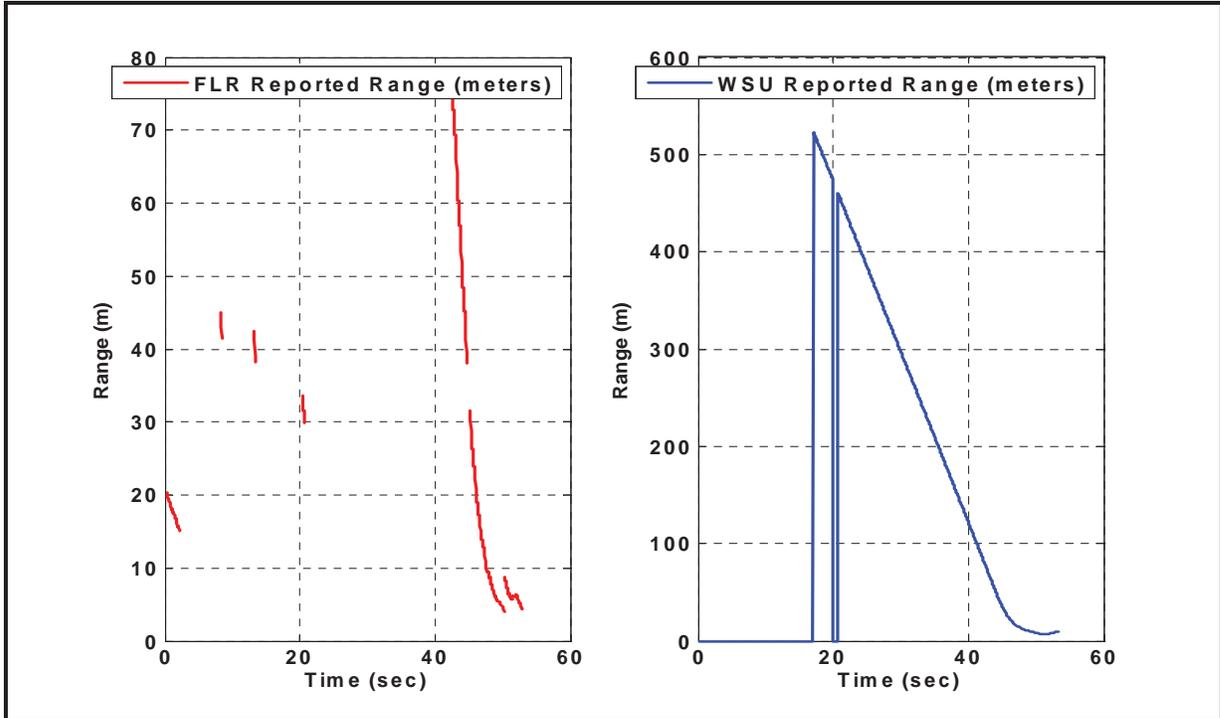
Figure 4: Sensor Performance on Detecting a Vehicle as an In-path Stationary Target
