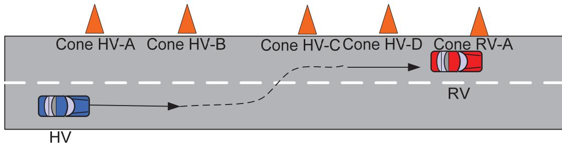
**Figure 5-8: HV Change Lanes behind Stopped RV**
