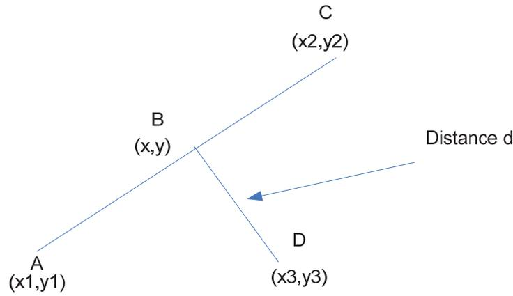
**Figure 6: Shortest Distance from a Point to a Line Segment**
