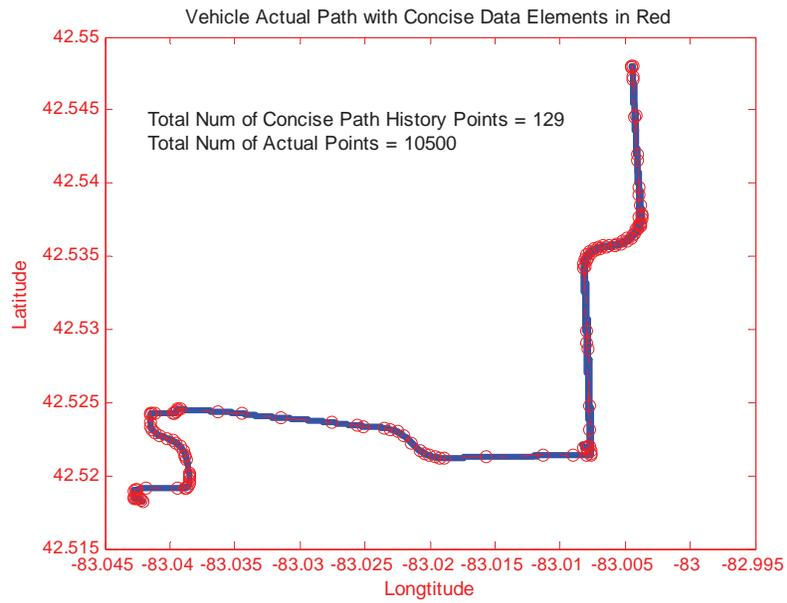
Figure 9: Method Two – Representation of Vehicle Path
