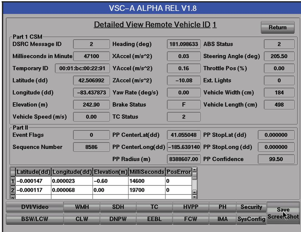
Figure 20: WMH – Remote Vehicle Detailed View EGUI Screen
