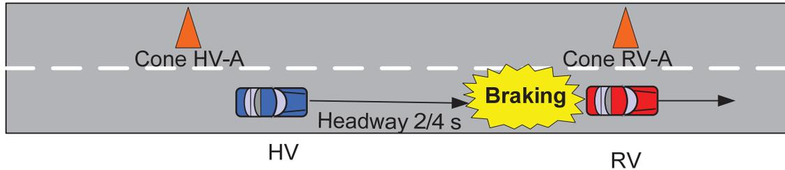
**Figure 5-5: HV Follows RV/ RV Brakes Hard**
