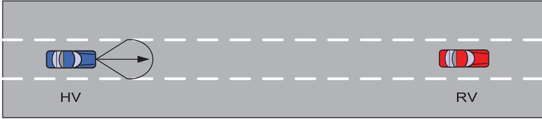
Figure 3: Confirmation of Stopped Vehicle as In-path Stationary Target
