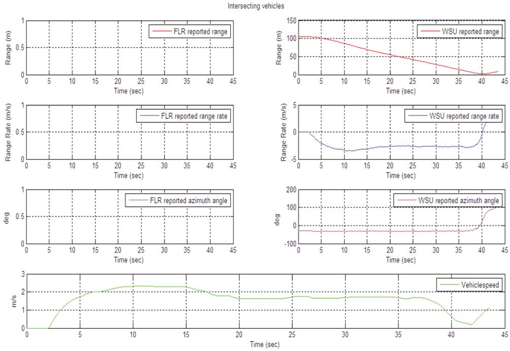
**Figure 14: Sensor Performance During Detection and Tracking of Intersecting Vehicles**
