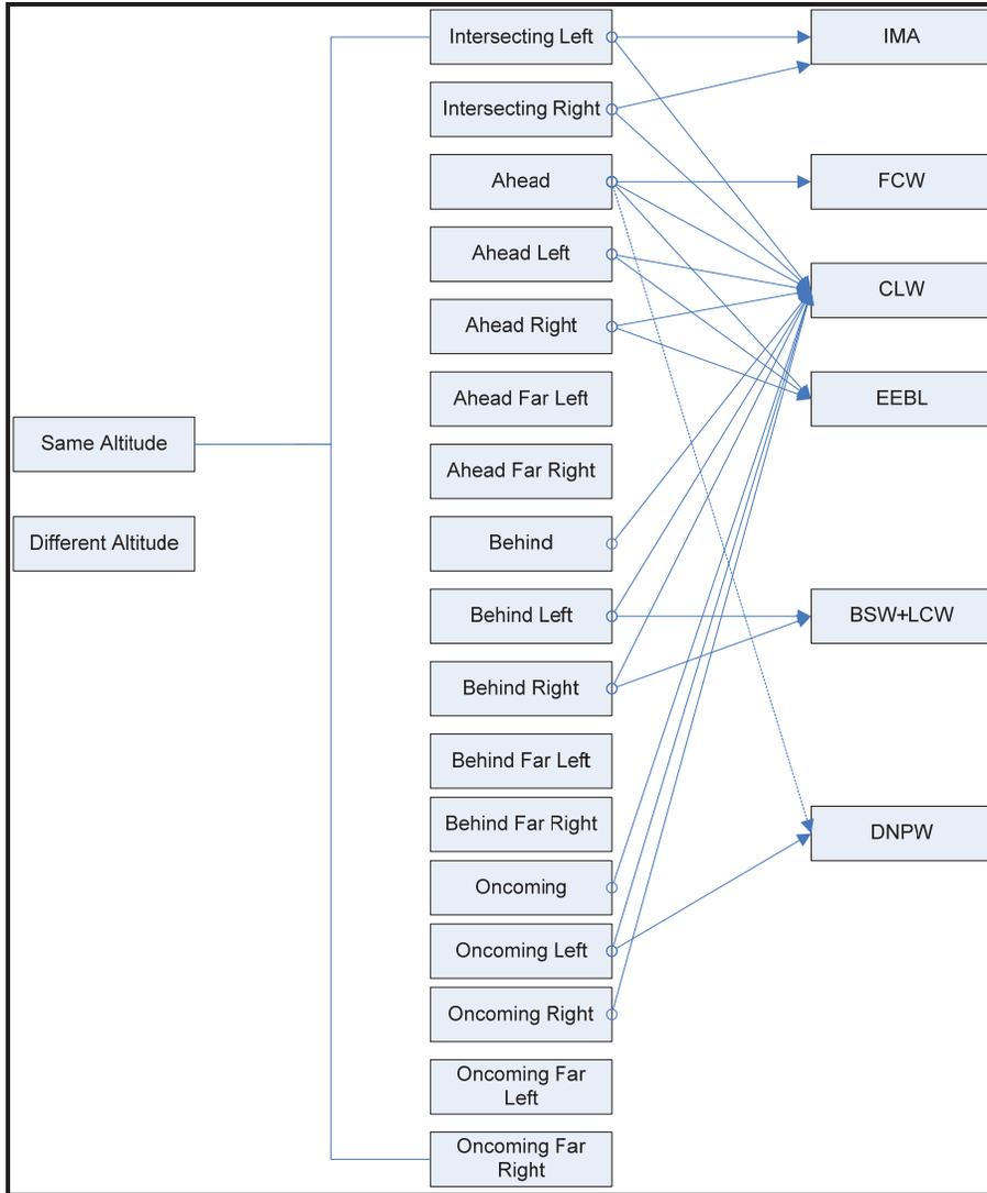
Figure 3: Target Classifications used by VSC-Applications
