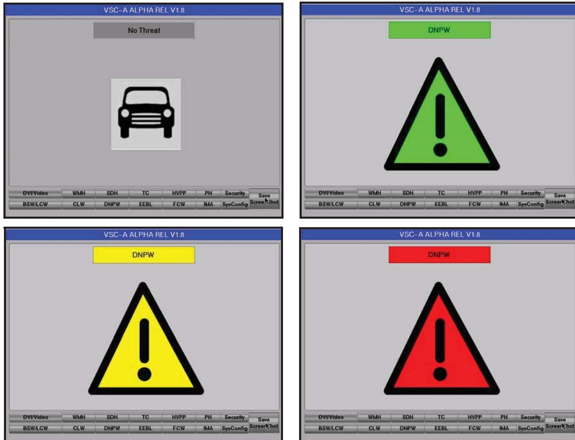
**Figure 12: DVIN Stages: (left → right, top → bottom) No Threat, Threat Detected, Inform Driver, Warn Driver**
