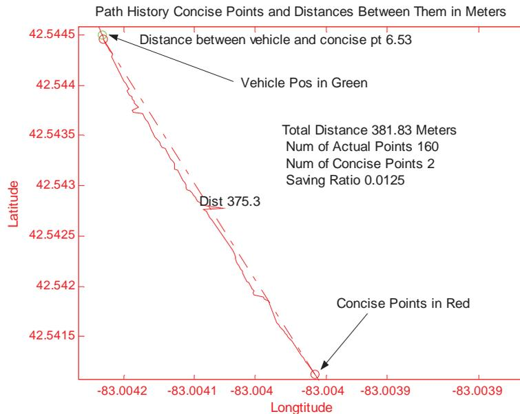
Figure 18: Method One – PH Representation of Straight Road
