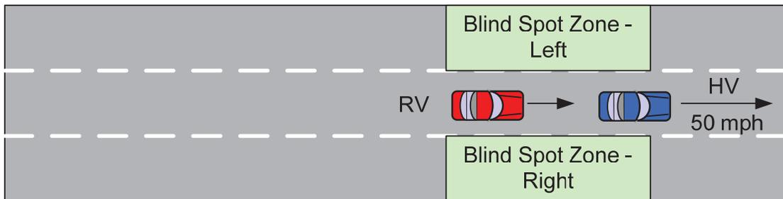
**Figure 6-6: RV Behind HV Test 6**
