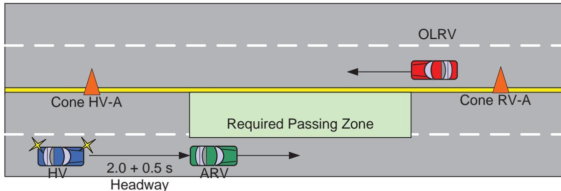
**Figure 7-3: Attempt to Pass when RV Does Not Occupy Adjacent Lane**
