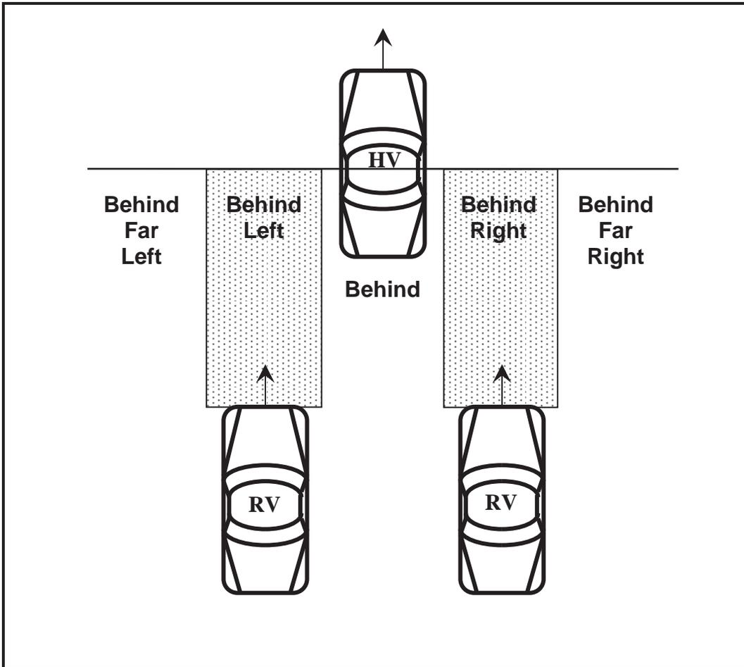
**Figure 6: BSW + LCW Target Classification Zones**
