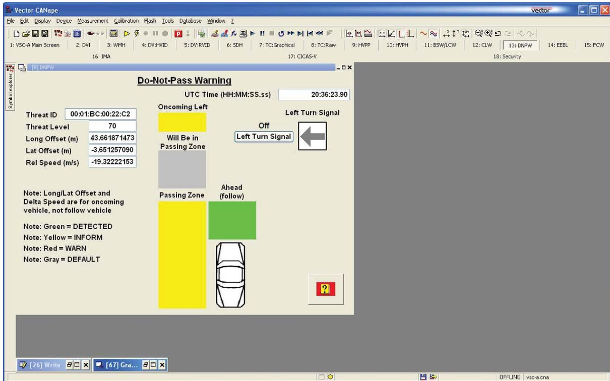
**Figure 4: Example Layout for the DNPW EGUI in the Visualization Tool**
