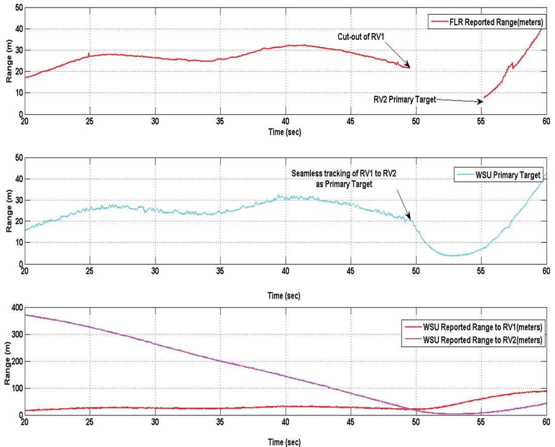
Figure 12: Sensor Performance during Vehicle Cut-Outs
