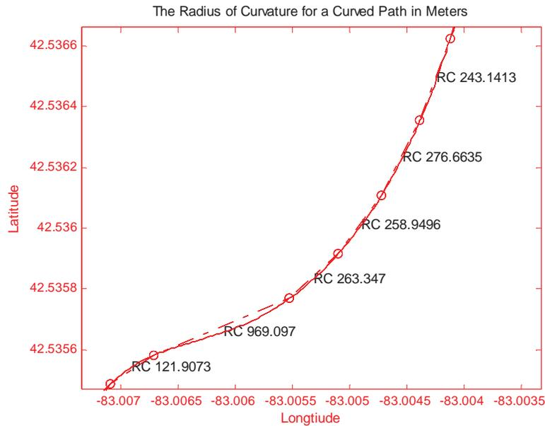
Figure 12: Method Two – Radii of Curvature for Curved Road
