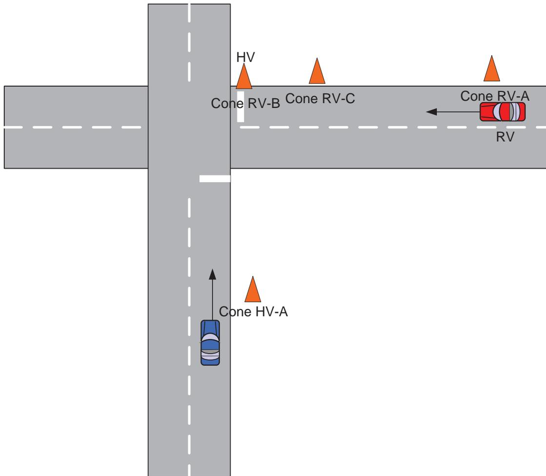
**Figure 8-4: Test Setup for Intersection Approach False Positive Tests, Two Vehicles Moving**
