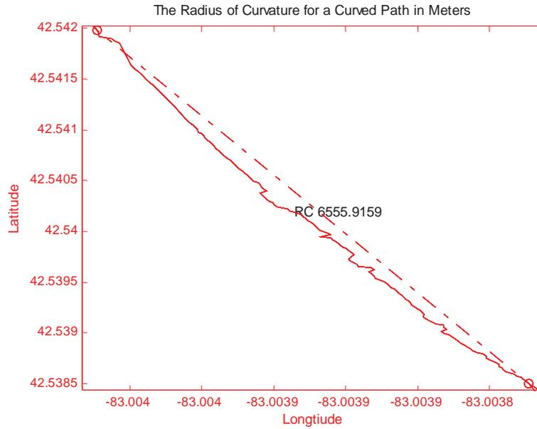
Figure 14: Method Two – Radii of Curvature for Straight Road
