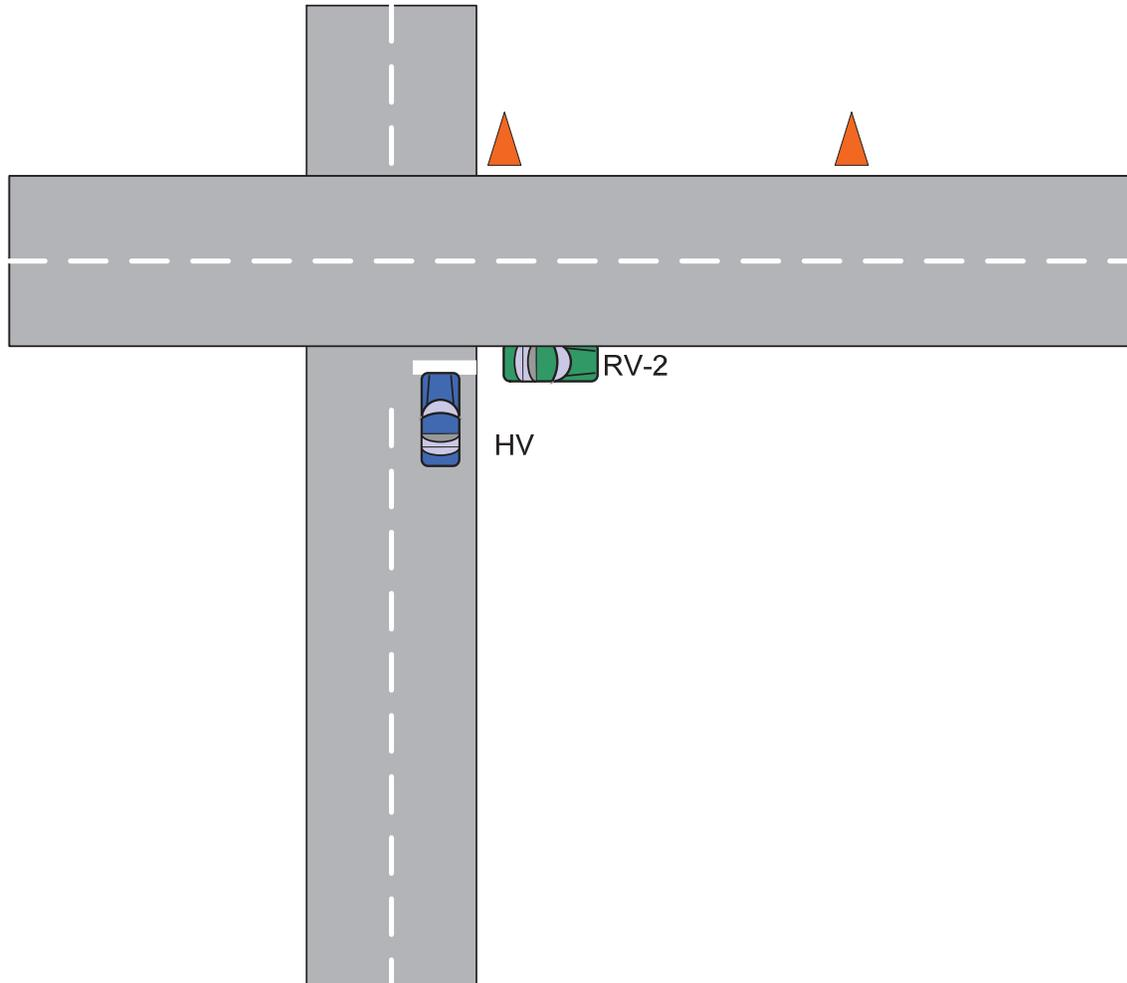
**Figure 8-5: Test Setup for Blocking Vehicle Test**
