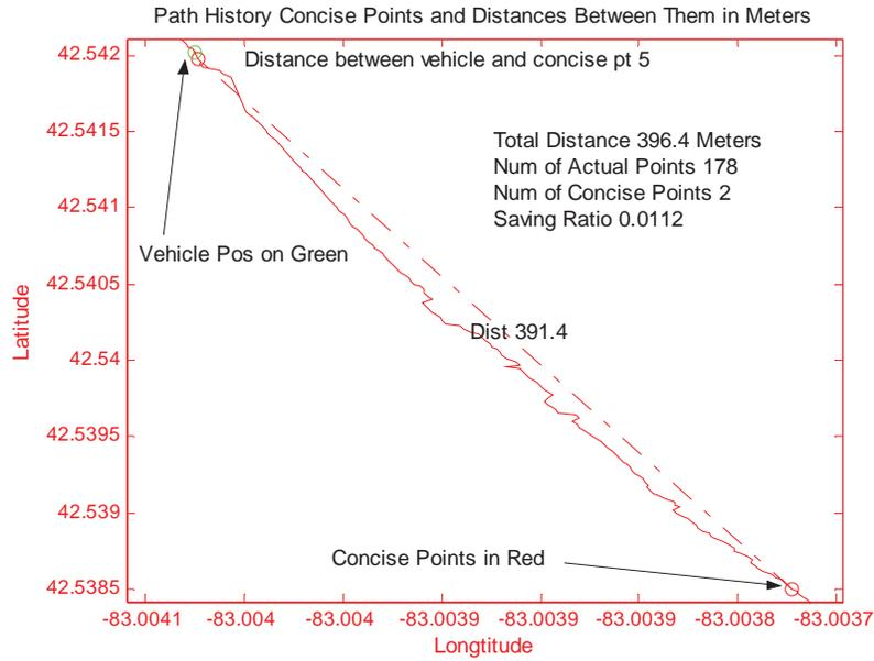
Figure 19: Method Two – PH Representation of Straight Road
