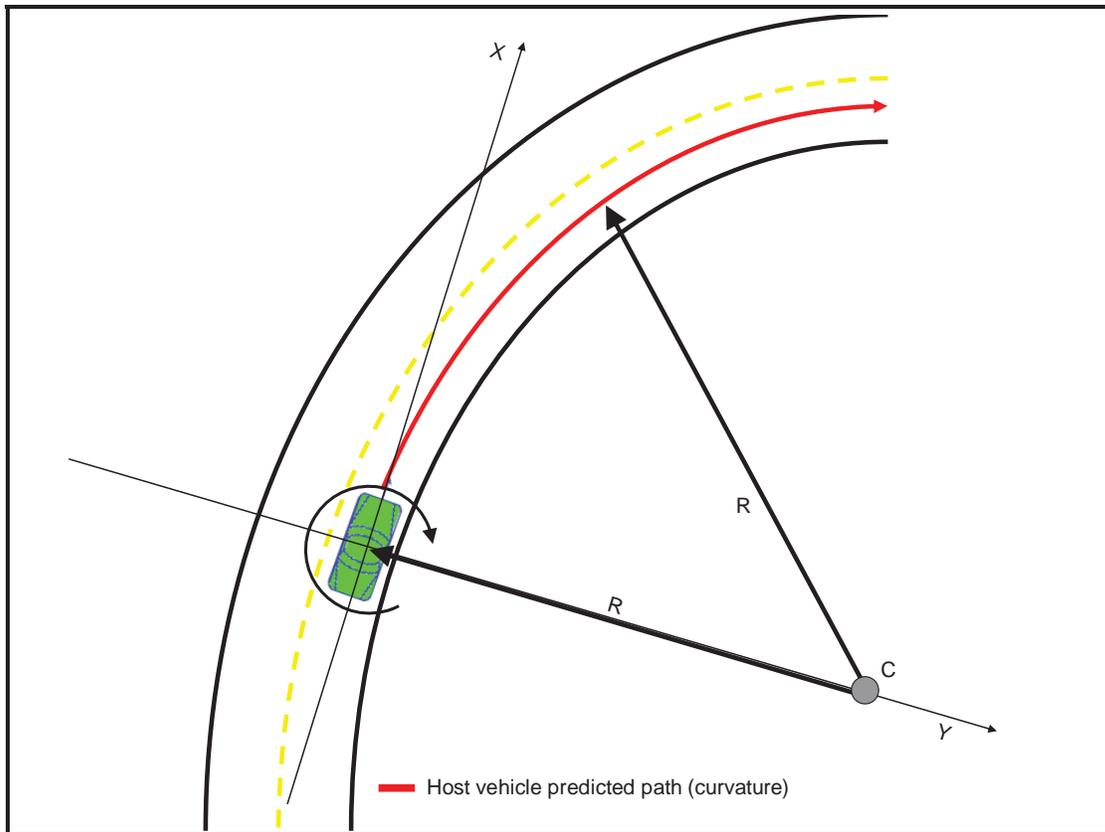
**Figure 1: Host Vehicle Projected Path**
