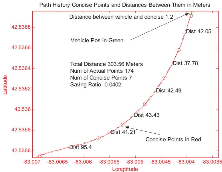
Figure 17: Method Three – PH Representation of Curved Road
