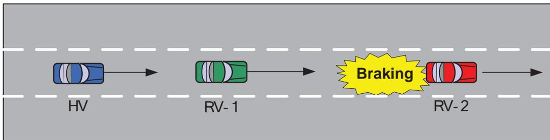
Figure 4-3: RV in Same Lane with Blocking Vehicle
