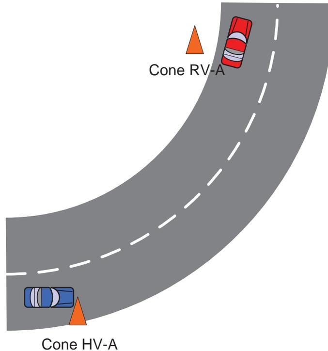
**Figure 5-6: RV in Left Lane on Curve (False Positive)**
