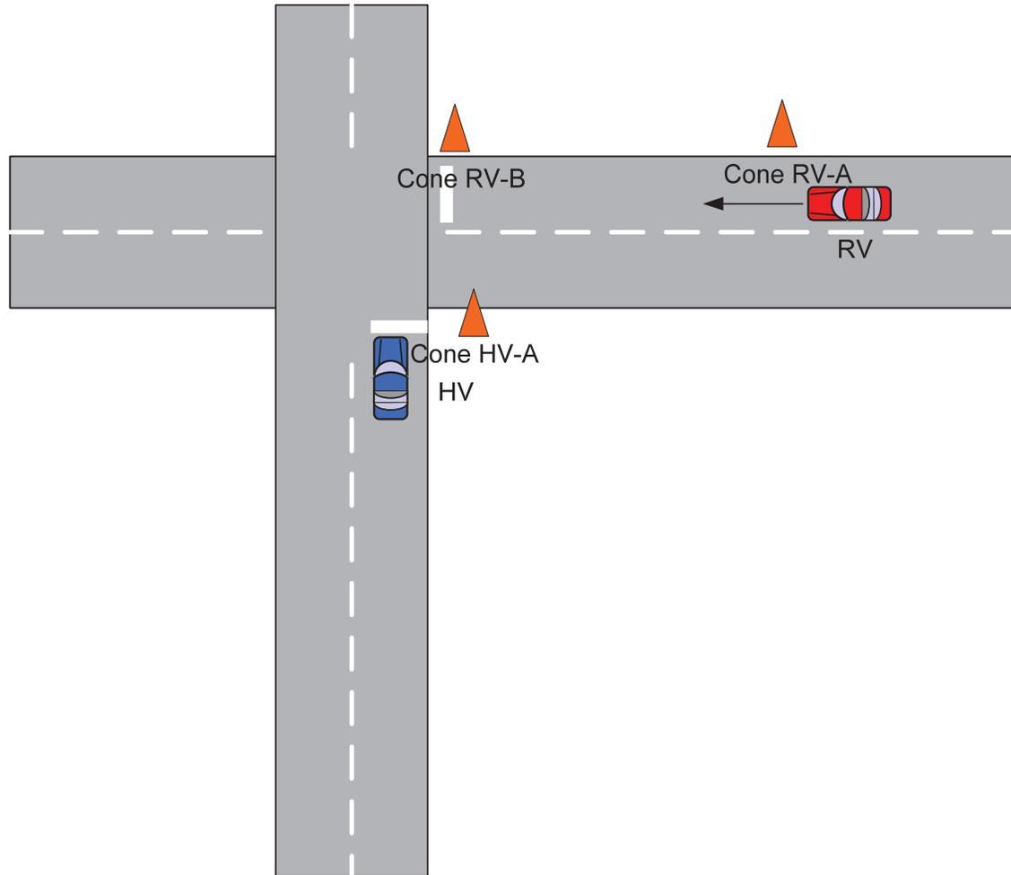
**Figure 8-2: Test Setup for Stopped Vehicle False Positive Test**
