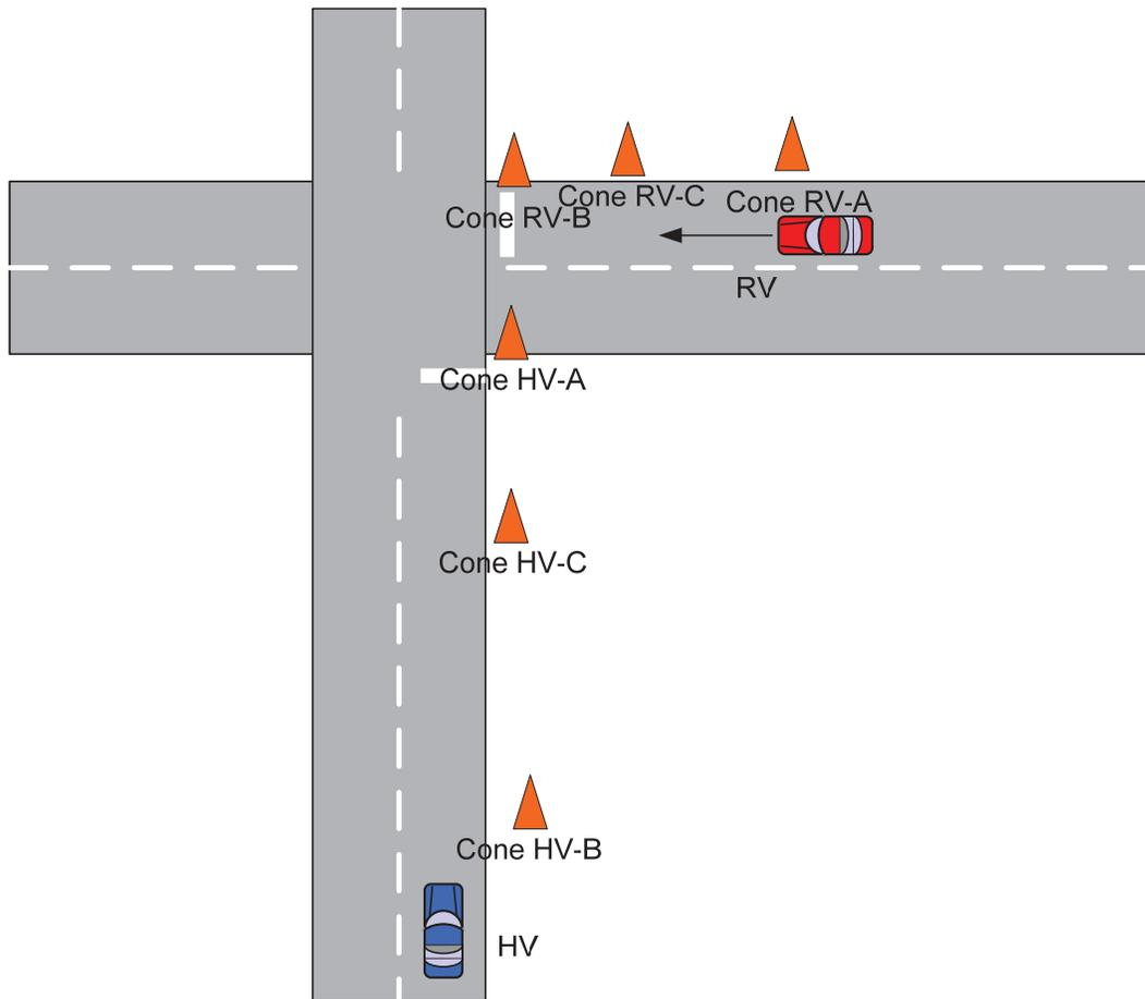
**Figure 8-3: Test Setup for Variable Speed Approach Tests, Both Vehicles Moving**
