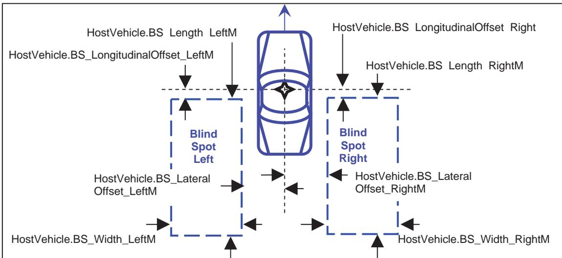
**Figure 4: Vehicle Blind Spot Zone Parameters**
