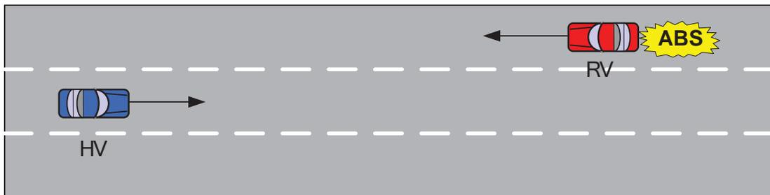
Figure 9-3: HV and RV in Opposite Directions
