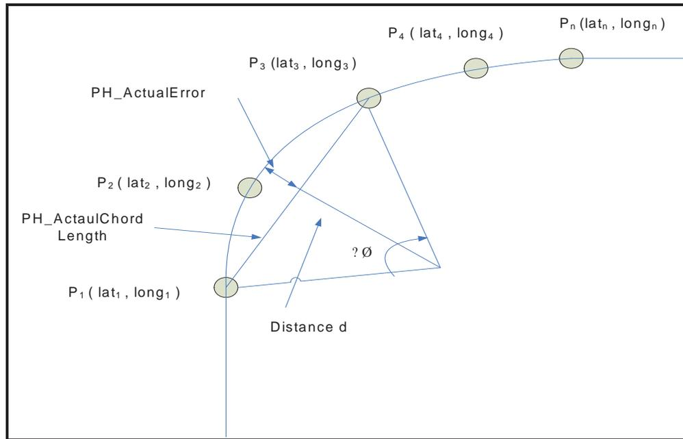
**Figure 11: Representation of PH Error**
