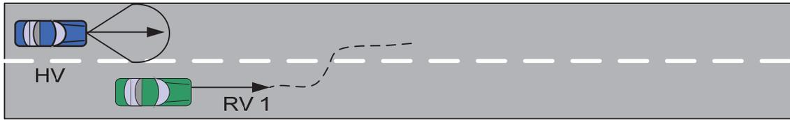
Figure 9: Cut-in of Lead Vehicle
