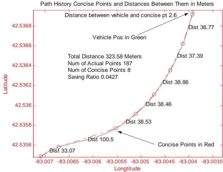
Figure 16: Method Two – PH Representation of Curved Road
