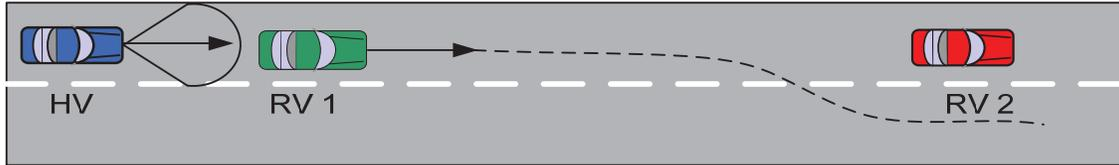
Figure 11: Cut-out of Lead Vehicle Reveals Stopped Vehicle In-lane
