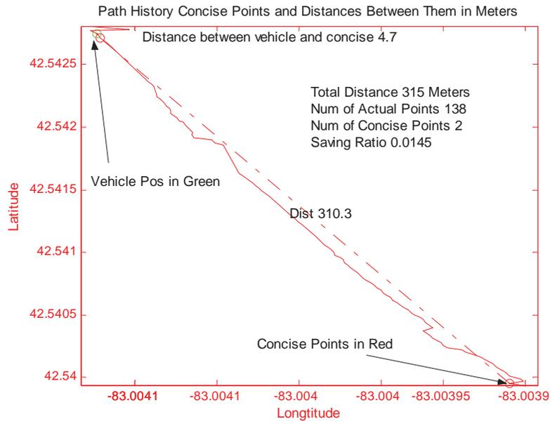
Figure 20: Method Three – PH Representation of Straight Road
