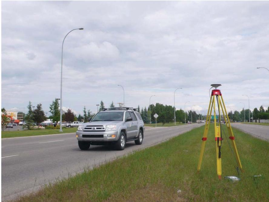
**Major Rural Throughway Representative of Low Elevation Masking Trees - Also Shows Test Vehicle Passing GPS Infrastructure Station**
