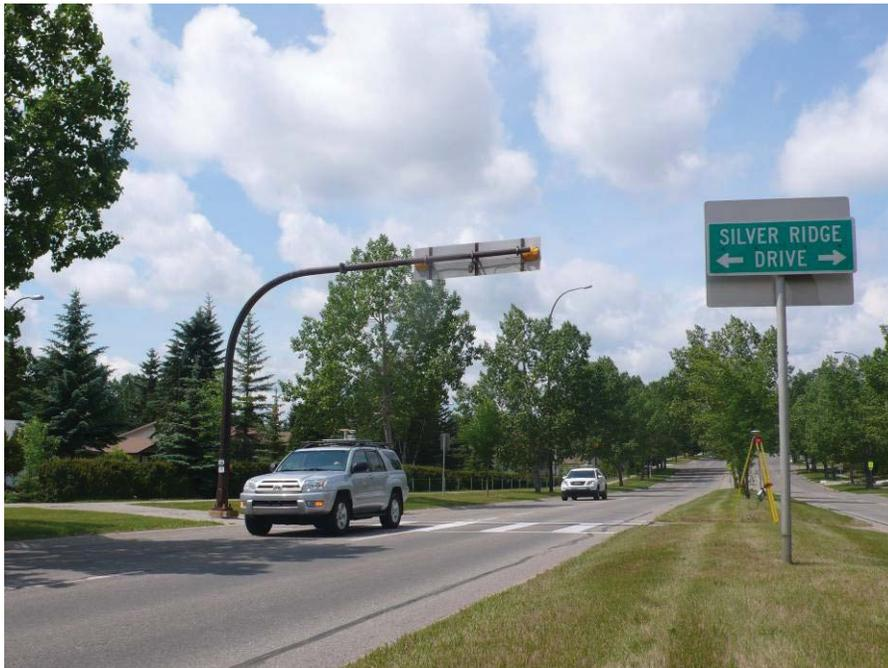
**Local Roads with Very High Foliage Signal Masking ( > 60 Degrees) and Location of a V2I Station**
