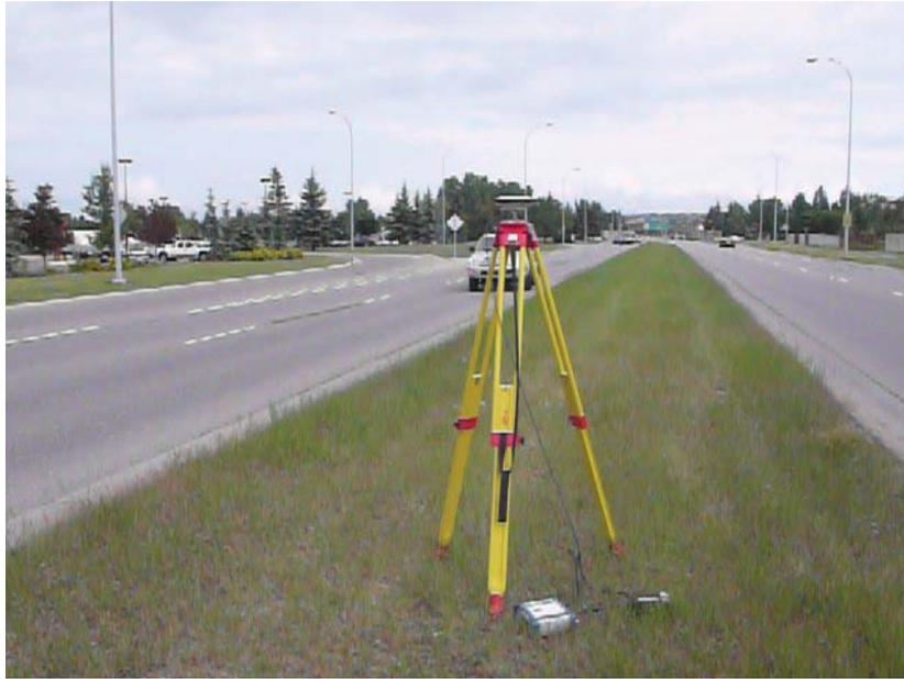
**Figure 3-5: Tripod Mounted Antenna and Receiver Used in V2I Tests**
