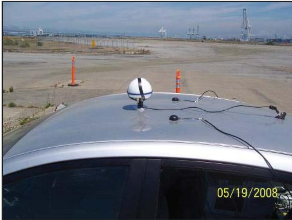
**Figure 3: Transmit Vehicle Antenna Placement: DSRC (2, Black) and GPS (White Sphere)**
