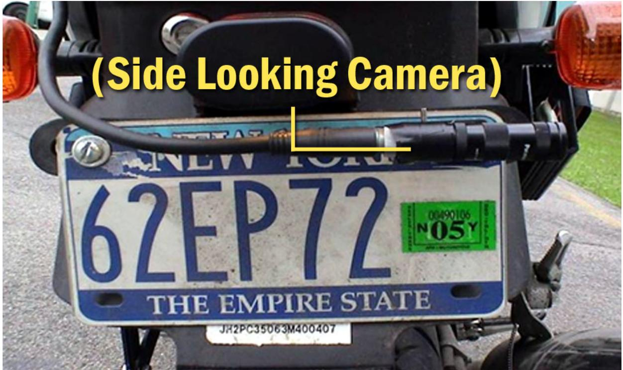
Figure 15. Side looking camera - Canadian test site
