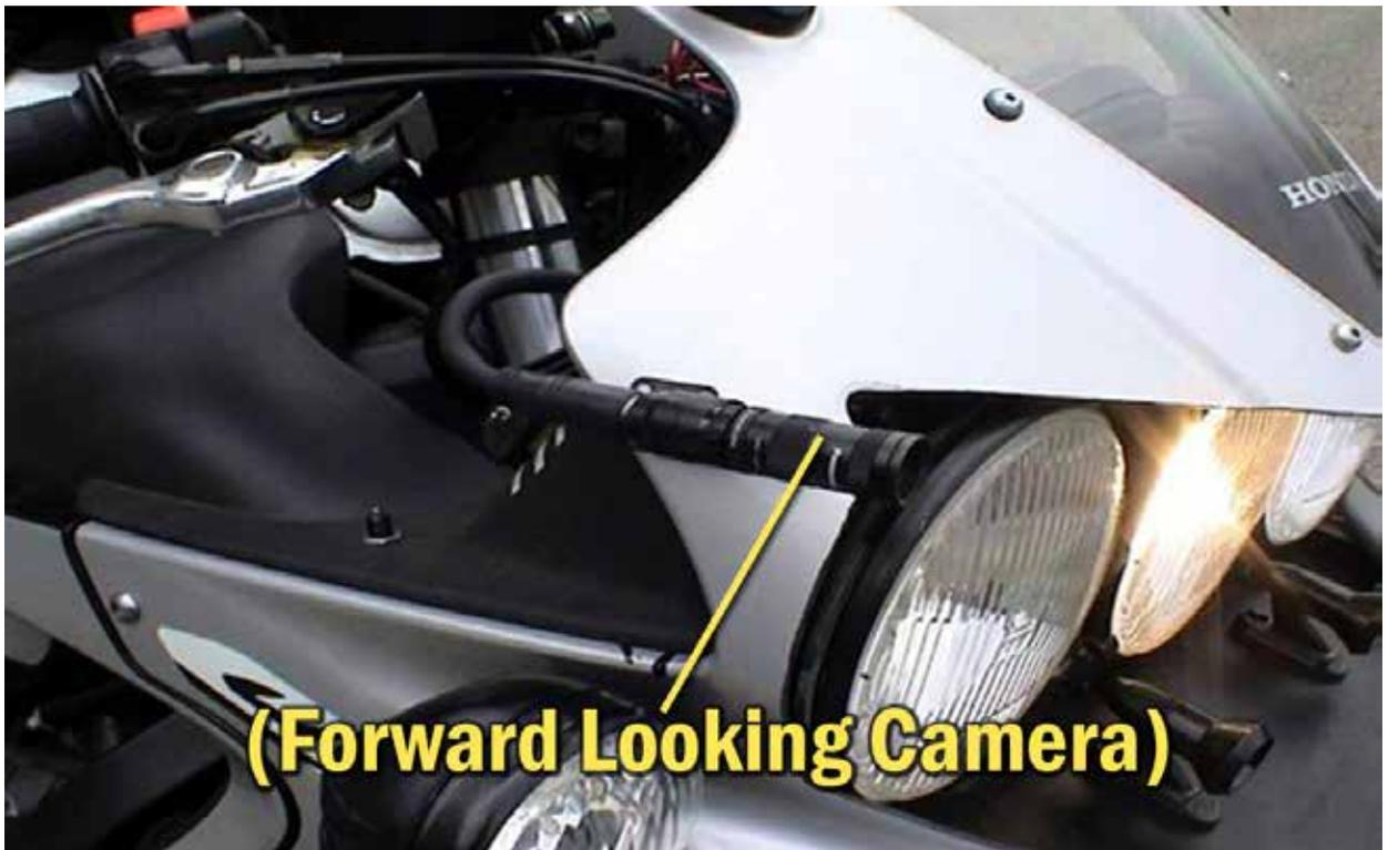
Figure 16. Forward looking camera - Canadian test site
