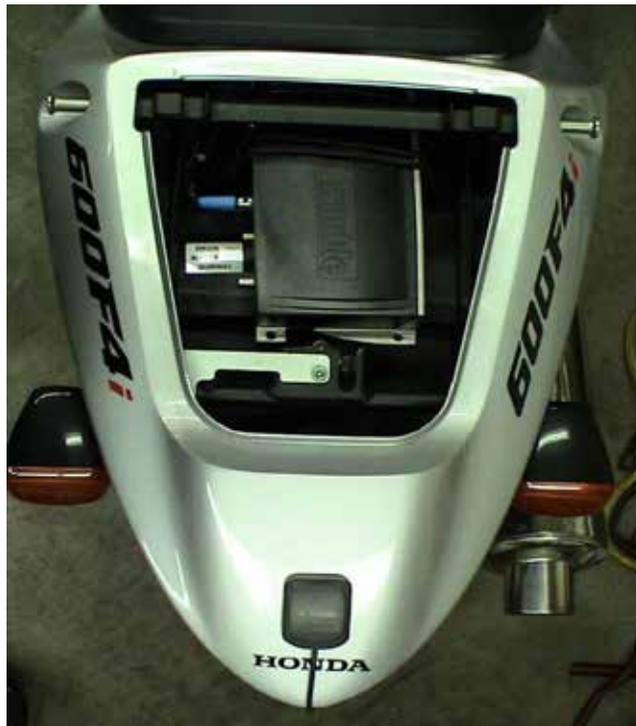
**Figure 26. Trimble Crosscheck, installed on motorcycle**
