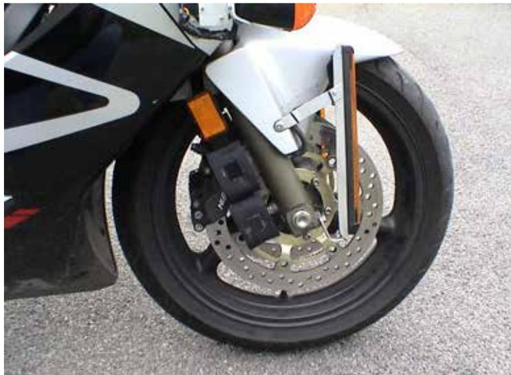
**Figure 22. Side retro-reflectors, standard configuration**
