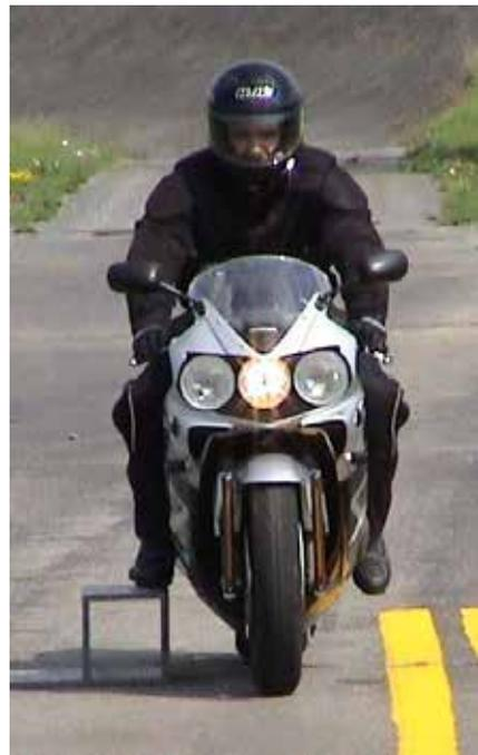
**Figure 5. Reduced intensity upper beam**
