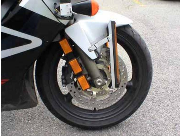
**Figure 21. Side retro-reflectors, all potential configurations**
