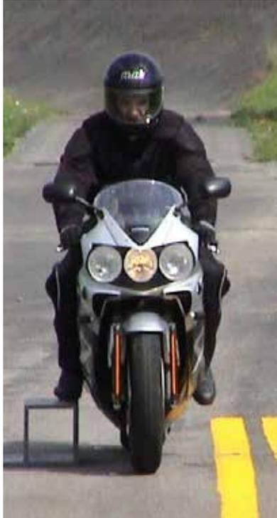
**Figure 6. Lower beam with fork lights**
