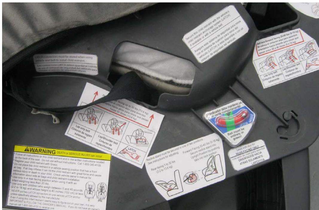
**ComfortSport rearranged label:** Recline label close to recline adjuster. Forward-facing belt routing directions under FF belt path. Rear-facing belt routing directions under RF belt path. Instructions to secure CRS with belt or LATCH in between belt paths. Instructions to store LATCH connectors near storage location. Level instructions under level.
