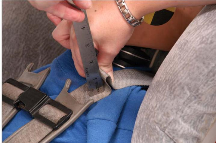
**Figure 8. Measuring amount of harness slack.**
