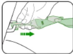
5 Press down and tighten LATCH belt
