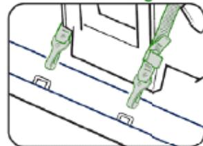
Pull connectors to make sure they are really attached to the vehicle anchorages.
