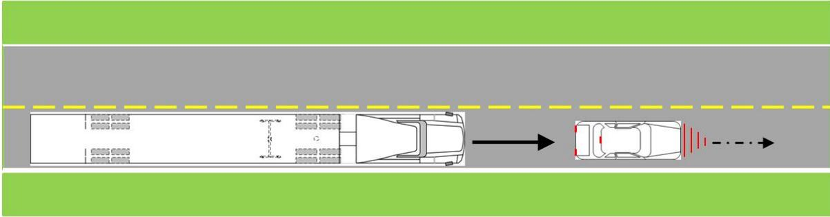
**Figure 8. Rear-End/Lead Vehicle Decelerating Crash Type**
