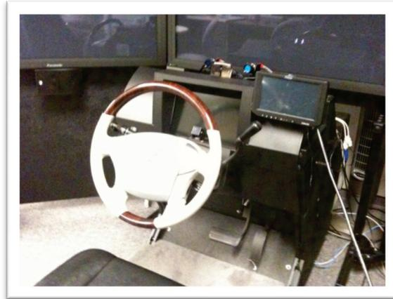
Figure 5. The NADS MiniSim with the 7-inch touchscreen display.
