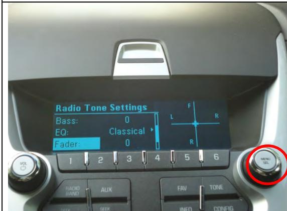
Continue to rotate the right knob, until “Fader” comes into view. Then PUSH the knob to select it.
