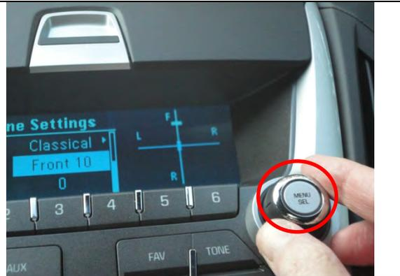
Then rotate to move the fader position toward the “F” for “front” by a noticeable amount
