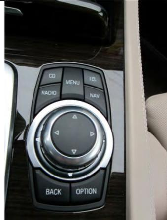
Primary manual control located on lower center console. The center circle contains the following controls:
