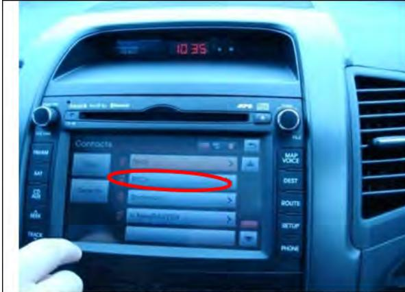
This brings the target name into view. Touch the name of the desired contact, “RICH” (this results in a display change, in which the name “Rich” is *replaced* on the next screen by Rich’s cell phone number).
