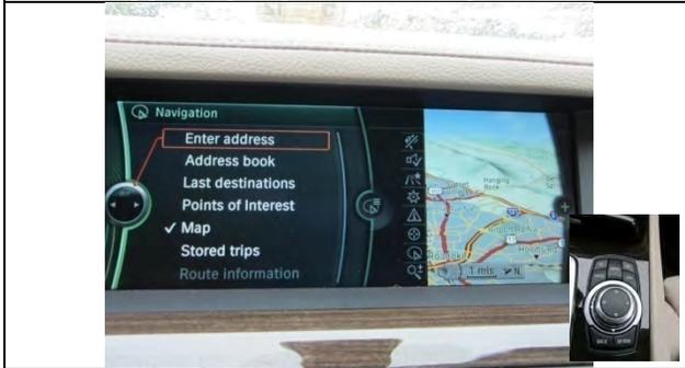
Turn rotary knob to highlight "Enter Address" and press knob.
