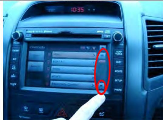
On the list of contact names that now appears on the screen, search for the desired name. To bring more names into view on the screen, press the down-arrow region of the scroll bar (touch screen lower right).
