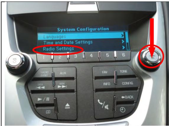
When “Radio Settings” is highlighted, PUSH in on center of knob.
