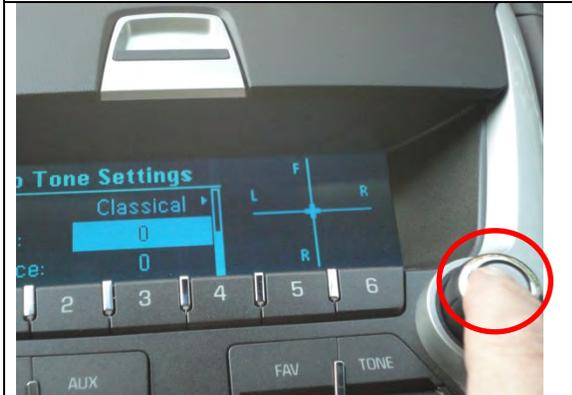
The screen shows the audio is balanced between front and back. Push on knob.
