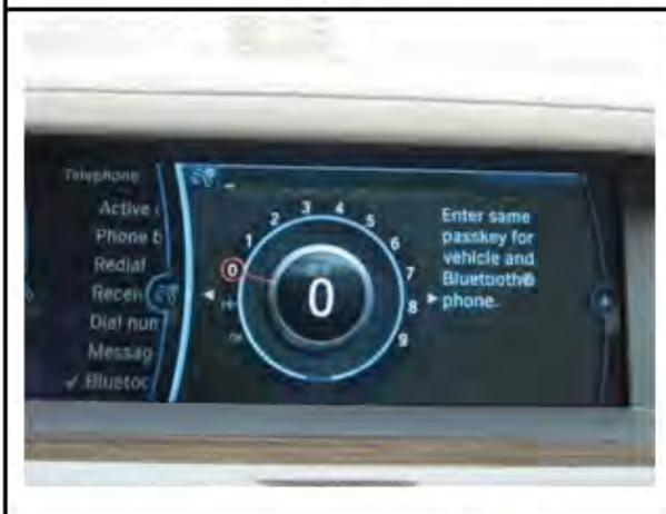
Enter that same passkey to the vehicle by using rotary dial to highlight the correct number and pressing knob to select correct number. Repeat for each number.
