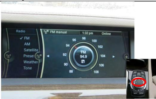
Turn rotary knob to station requested. (Task is finished when correct radio band and frequency is displayed).
