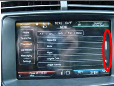
On the list of contact names that has appeared on the screen, search for the desired name by using the white vertical scroll bar on the right side of the screen, by touching it and moving it downward. (An alternate method would be to push the downward arrow twice on the touch screen but that would need to be tested separately.)
