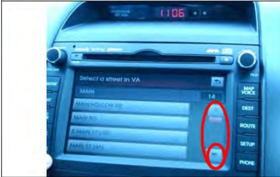
List of street names appears on the screen. To bring the desired street name into view, press down scroll arrow button on touch screen.
