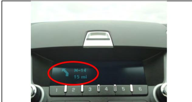
Immediately following the turn (just as a driver completes the maneuver), the route guidance system informs the driver that the next turn is 15 miles away and will involve bearing left on M-14. This allows the driver some ‘closure’ and enables the driver to focus on just driving until the next route guidance instruction is received. It **represents the end state** of this dependent task.
