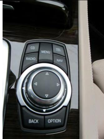
Primary manual control located on lower center console. The center circle contains the following controls:
