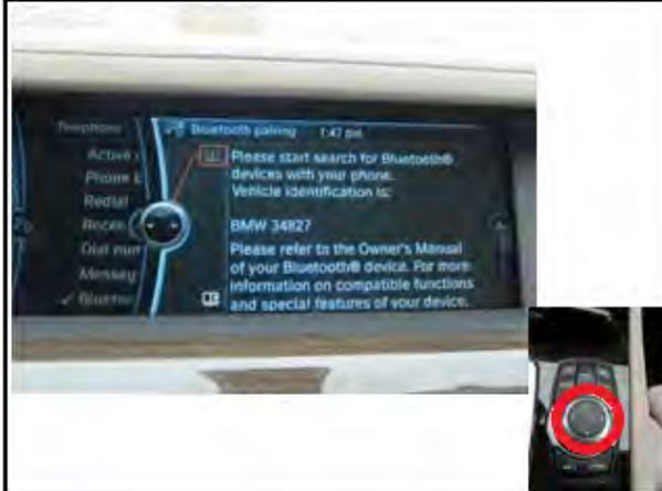
Use Bluetooth on handheld phone to connect by identifying vehicle on phone and entering a passkey on phone.
