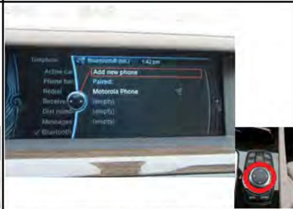
Turn the rotary knob to highlight "Add new phone" and press in knob.
