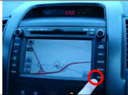
Push "Phone" button (a hard button next to screen). (Note: An alternate method would be to start the process with a press on the steering wheel button for phone. However, this would constitute a separate, testable task; one that should also be tested.)
