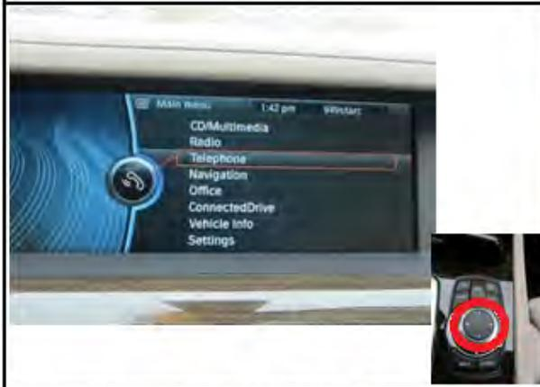
Turn the rotary knob to highlight "Telephone" and press in knob.
