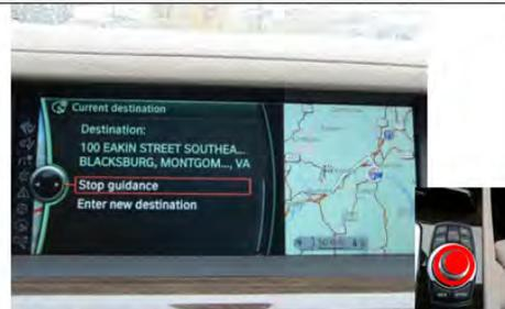
Press in knob to stop guidance. Task is finished at this point.
