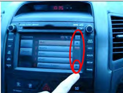
To continue bringing more names onto the screen in search of the desired name, press the scroll down-arrow again (2<sup>nd</sup> time).
