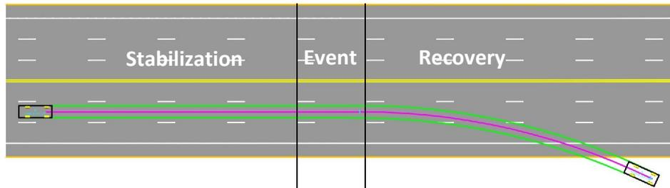
The drawing block for the straight parallel lane is shown in Figure 4. The 1,200 meter length provides adequate room for vehicle speed stabilization, the execution of a maneuver, and room to recover control of the vehicle. The roadway can be configured to simulate many roadway types, both freeway and non-freeway.
