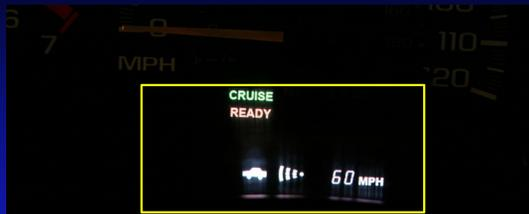
The ACC system has a display located in the lower portion of the speedometer, shown above. This display indicates the presence of a vehicle in front of you, your current distance setting, and your set speed.
