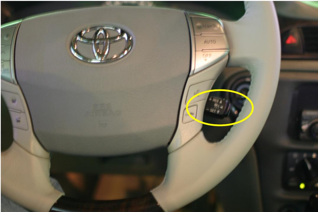
Figure 1: ACC Controls in NADS-1.
