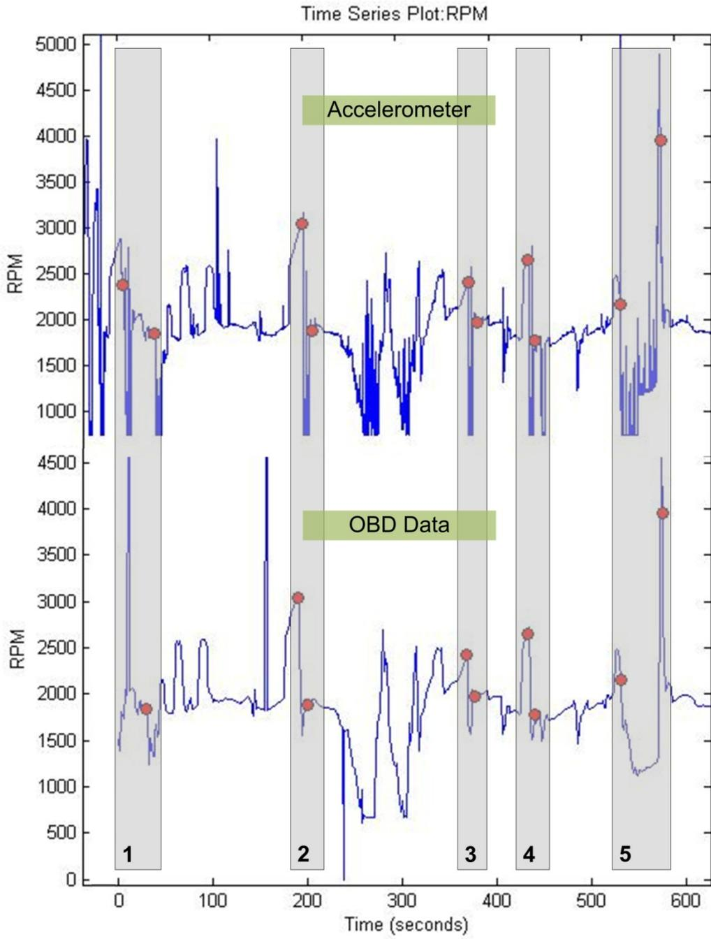
Figure 20: OBD and Accelerometer Data: Engine RPM
