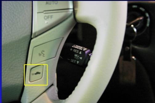
During your drive, you will be able to change the ACC system distance setting by pressing the distance setting button on the steering wheel, shown above.
