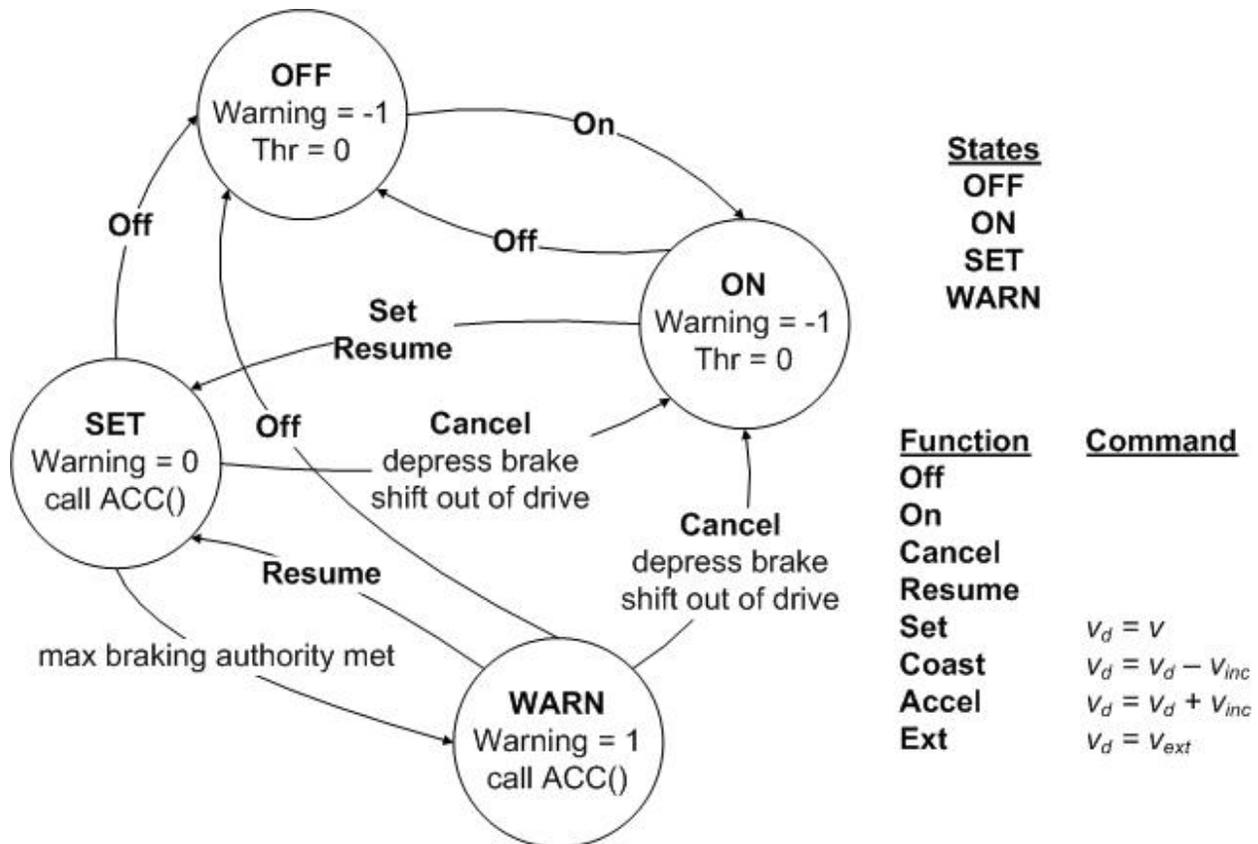
Figure 22: Cruise control state transition diagram
