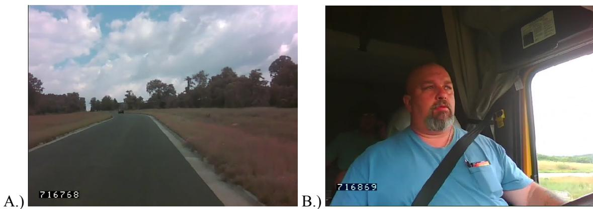
**Figure 3. (A) Sample Image of the Forward-Facing Video Collected by the MiniDAS (B) Sample Image of the Driver-Facing Video Collected by the MiniDAS**
