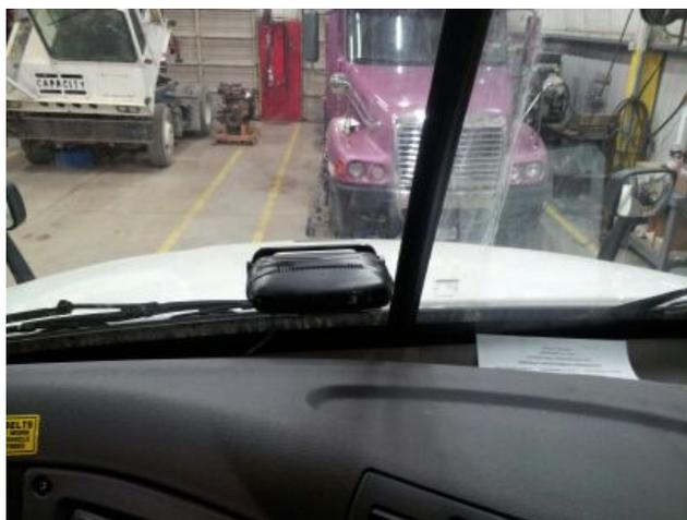
**Figure 2. MiniDAS Placement in Center of Windshield**
