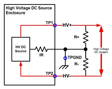
Figure 11. Test points for source without disconnects.
