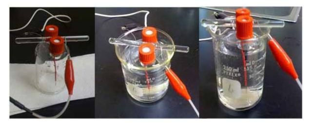
Figure 19. Glass electrode for megohmmeter.
