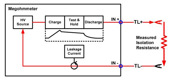
Figure 1. Diagram of a megohmmeter with positive and negative test leads, TL+ and TL-, respectively.
