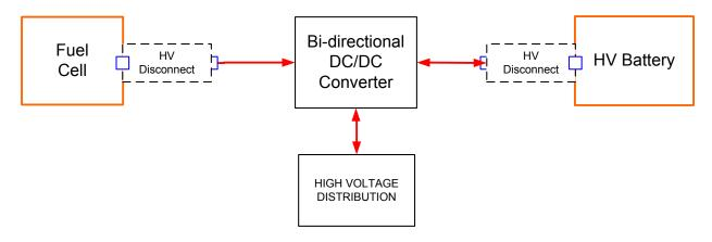
Figure 9. Simplified HFCV power system diagram.
