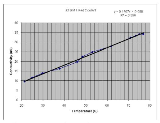
Figure 23. Aged Glysantin sample from General Motors results at increasing temperatures.
