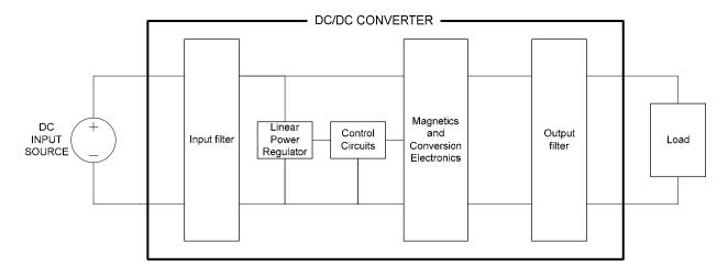
Figure 14. DC to DC converter block diagram.
