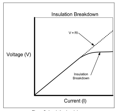
Figure 5. Insulation breakdown.
