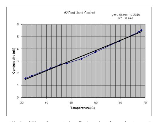
Figure 22. Aged Glysantin sample from Ford results at increasing temperatures.
