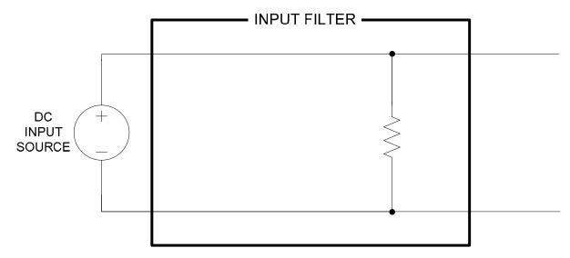
Figure 16. Input power filter DC equivalent circuit.
