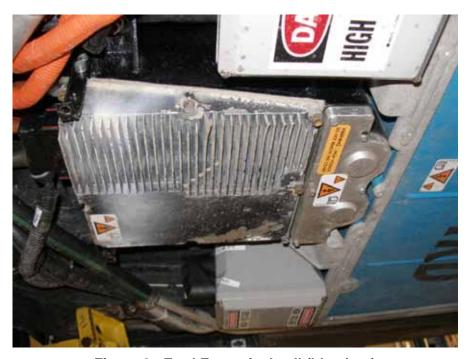
Figure 3. Ford Focus fuel cell (blue box) and electronic/disconnects enclosure.
