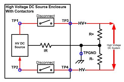
Figure 3. High-voltage source with marked test points having direct access to the high-voltage terminals.
