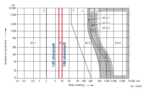
Figure 2. Conventional time/current zones of effects of DC currents on persons for a longitudinal upward current path (IEC TS 60479-1: 2005-07) with 100 ohms/volt and 125 ohms/volt references added.
