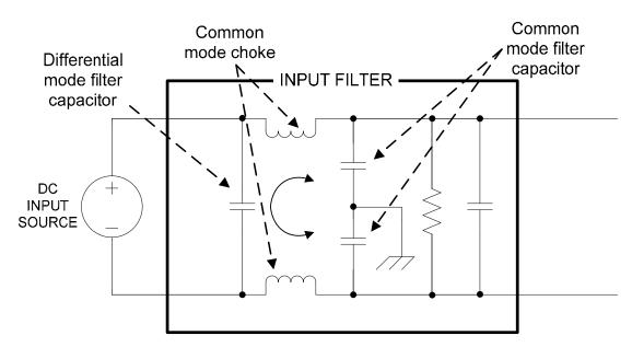
Figure 15. Input power filter.
