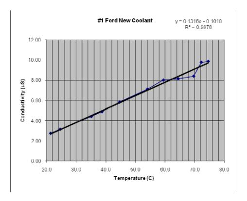
Figure 21. New Glysantin sample from Ford results at increasing temperatures.
