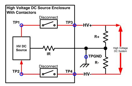
Figure 12. Test points for source with disconnects.
