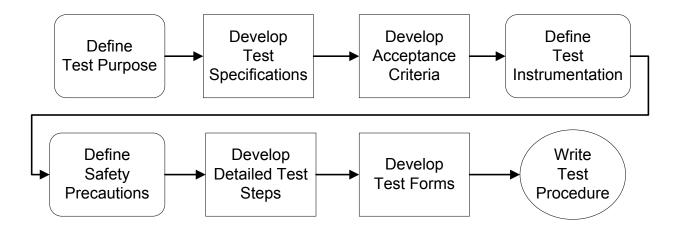
Figure 1. Test procedure development diagram.
