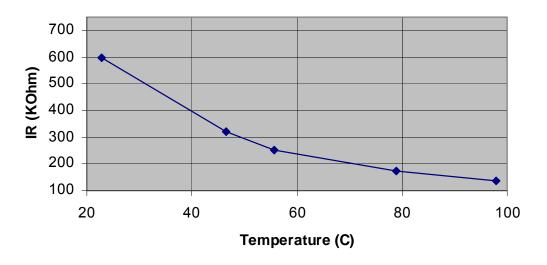
Figure 20. Glysantin megohmmeter results at increasing temperatures.
