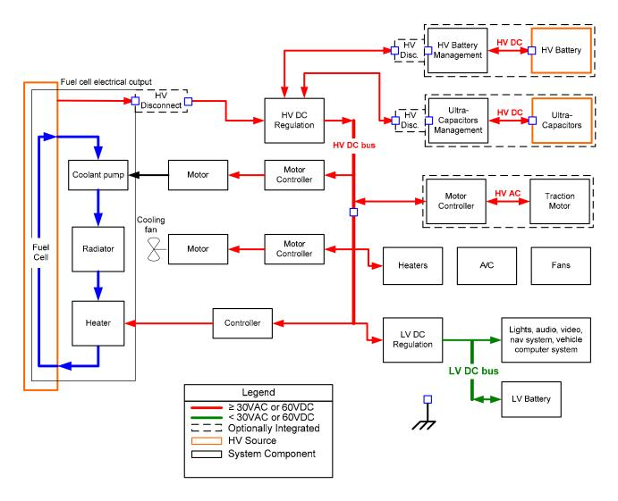
Figure 8. General block diagram for an HFCV with test points and disconnects.
