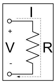
Figure 4. Voltage (V), current (I), and resistance (R) of a conductor.
