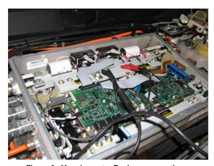
Figure 2. Megohmmeter Equinox connections.
