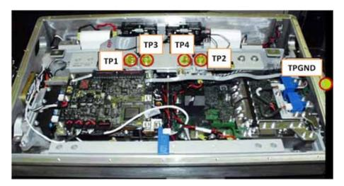
Figure 13. GM Chevrolet Equinox test point locations.
