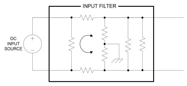
Figure 17. Input power filter AC equivalent circuit.
