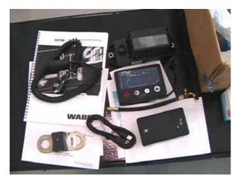
Figure 2.9. Components Kit for IVTM Flow-Through 10-Tire System
