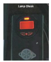
Figure 2.17. Power-Up Lamp Check
