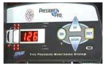
Figure 2.38. PressurePro Display Showing 126 psi Tire Pressure in Right Front Tire Instead of the Applied 130 psi CIP
