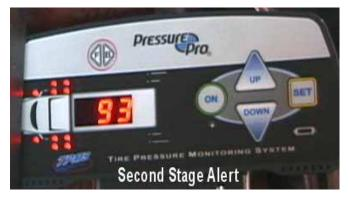
Figure 2.36. Left Front Steer Tire Channel Is Warning of a Second Stage Low-Pressure Detection
