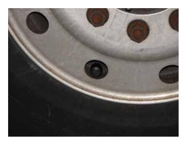
Figure 2.13. PressurePro Transmitter on Valve Stem in Aluminum Steer Wheel of the Tractor with Small Hand Holes
