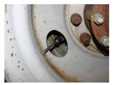
Figure 2.14. Side View of Two PressurePro Sensors Mounted on Dual Steel Wheels Sensors Were Installed With the Wheels Already Mounted on the Hubs
