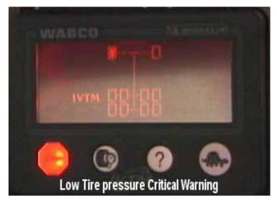
Figure 2.30. Critical Low-Pressure Warning Indicates to Driver to Stop and Service Tire
