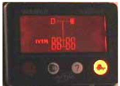
Figure 2.29. First Low-Pressure Warning in Right Front Steer Tire
