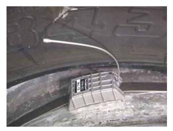
Figure 2.4. Rim-Mounted Tire-SafeGuard Sensor with High-Gain Antenna Note-Tire is Pushed Back and Must Clear Antenna When Tire is Moved to Final Position
