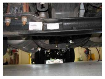
Figure 2.3. SmartWave Receiver/Gateway Mounted on Transmission Lower Crossmember
