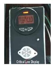
Figure 2.21. Critical Low-Pressure Warning
