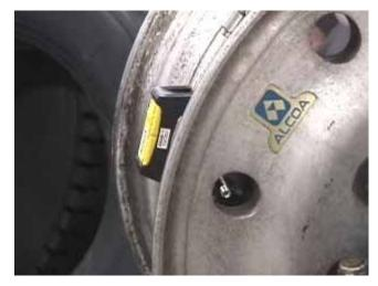
Figure 2.2. SmartWave Sensor Mounted on Lowest Section of Rim with Steel Band
