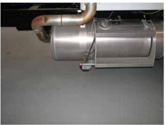
Figure C.5. Noncontact Radar Speed Sensor Mounted Beneath the Aluminum Fuel Tank
