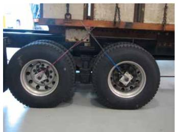
Figure B.2. Air Lines and Rotary Unions on Right Side Drive Tires of the Truck
