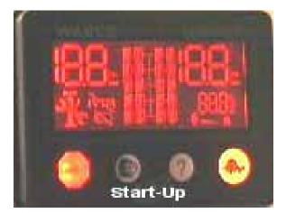
Figure 2.26. Startup Lamp Check
