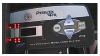
Figure 2.39. PressurePro Display Showing All Active Sensors, But No Pressure Indications
