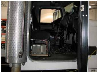
Figure C.4. Data Acquisition Computer Mounted Beneath the Observer's Seat
