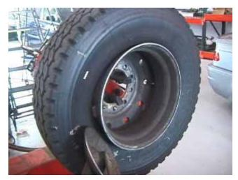
Figure 2.6. Tire Being Removed from Rim-Mount Tire-SafeGuard
