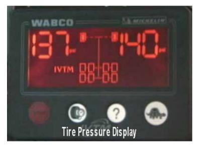
Figure 2.28. Steer Tire Pressures after "Hot" Calibration Test
