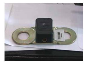
Figure 2.11. IVTM Wheel Lug Plate with Mounted Transmitter Port at Front Connects Air Line to Valve Stem
