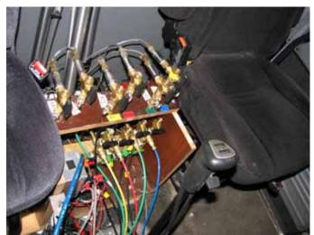
Figure B.4. Pressure Control Manifold Showing All Ten Ports
