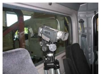
Figure C.1. Video Camera Mounted Between Driver and Observer For Logging All Test Activities
