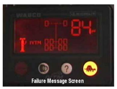
Figure 2.31. Information Screen Showing Tire Pump Signifying that a Tire Needs to be Re-Inflated
