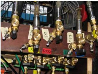
Figure B.1. Pressure Transducers and Signal Conditioners
