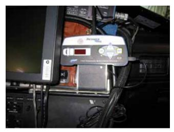
Figure 2.12. PressurePro Driver Display Mounted in the Truck
