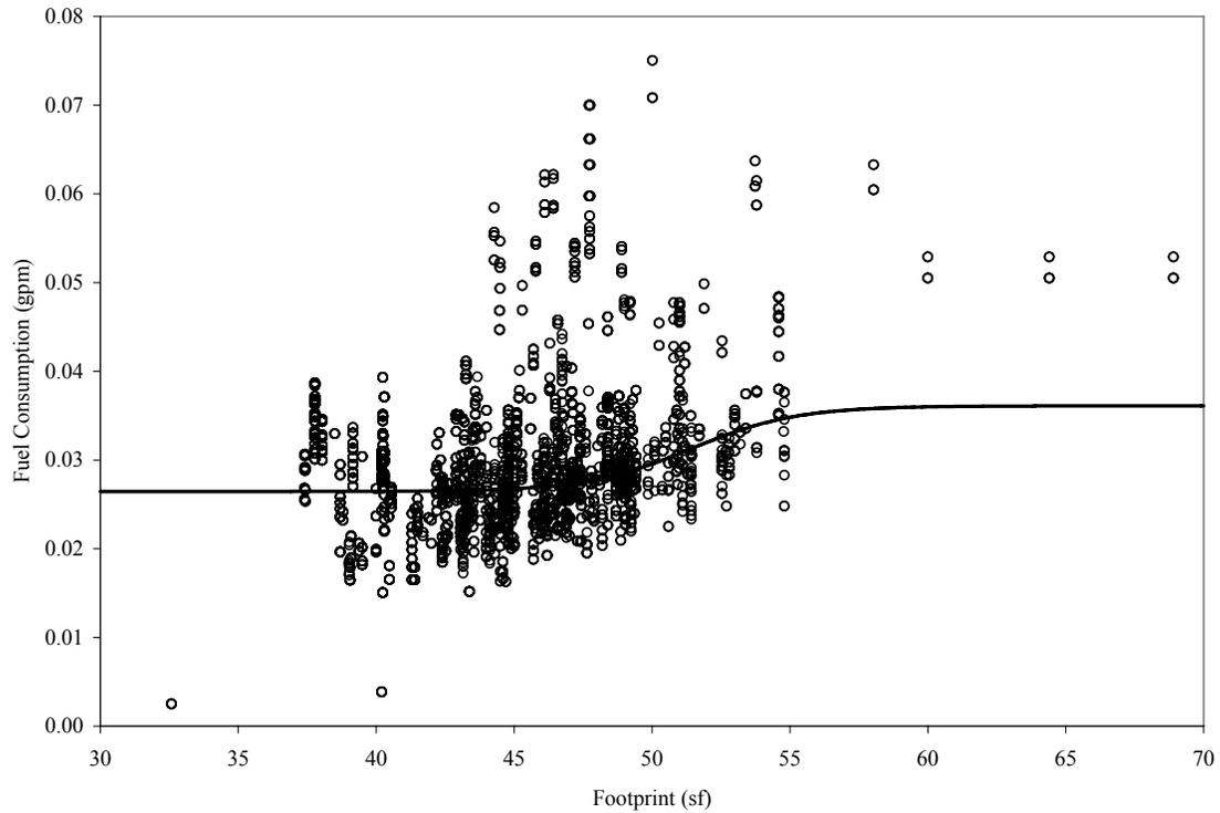
For light trucks, the same procedure yielded a curve with the following coefficients:  $A = 36.43$  mpg,  $B = 26.43$  mpg,  $C = 56.41$  square feet, and  $D = 4.28$  square feet. This curve, shown below on a fuel consumption (*i.e.*, gpm) basis, produced an average absolute difference of 14 percent.
