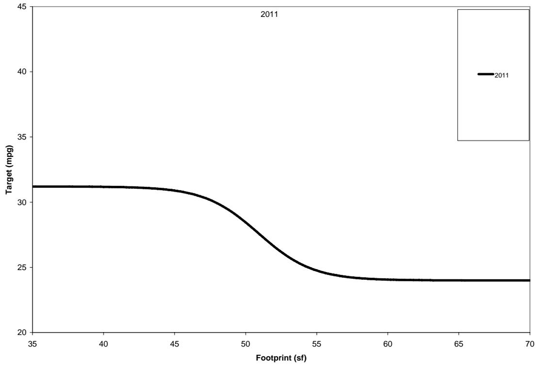
**Figure V-7. Final Light Truck Target Functions**
