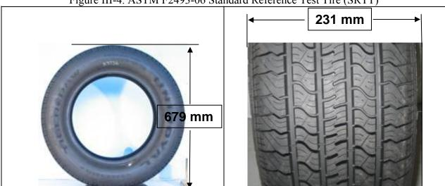
Figure III-4. ASTM F2493-06 Standard Reference Test Tire (SRTT)
