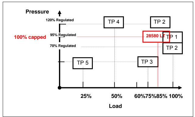
Figure III-3. ISO 28580 Draft Standard Test Conditions for "C" or LT,  $Li \ge 121$  Tires
