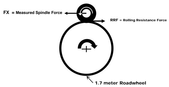
Figure IV-2. Force Method Rolling Resistance
