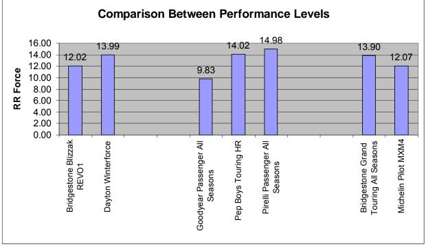
Figure III-20. Comparison between performance levels for passenger tires.
