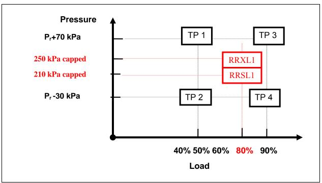
Figure III-2. ISO 28580 Test Conditions for Standard Load (RRSL1) and Extra Load (RRXL1) Passenger Tires
