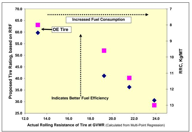
Figure IV-4. Tire Rating Versus Estimated On-Vehicle Tire Rolling Resistance, RRF (Blue) or by RRC (Pink)
