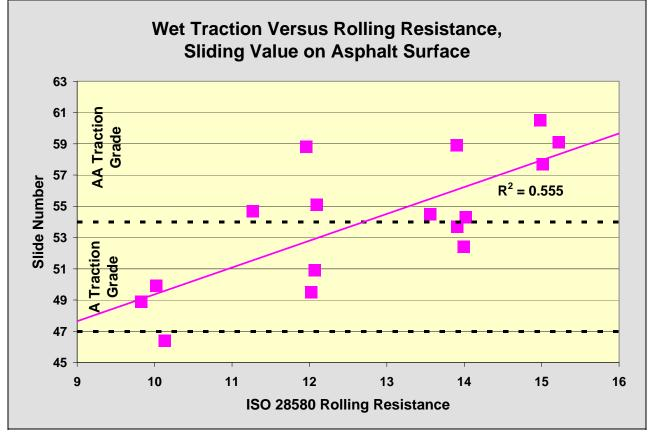
Figure III-16. Asphalt Wet Traction Rating Versus ISO 28580 Rolling Resistance
