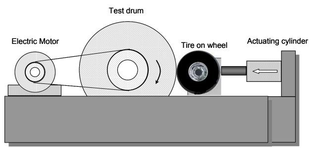
Figure IV-1. Typical Test Configuration for Rolling Resistance Measurements
