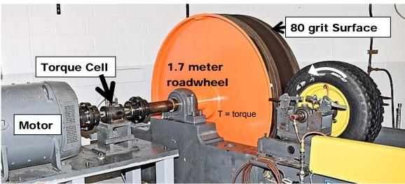
Figure IV-3. Torque Method Rolling Resistance
