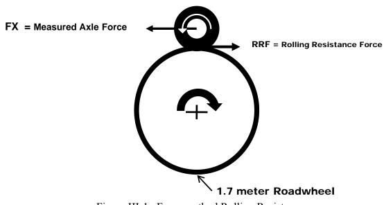
Figure III-1. Force method Rolling Resistance
