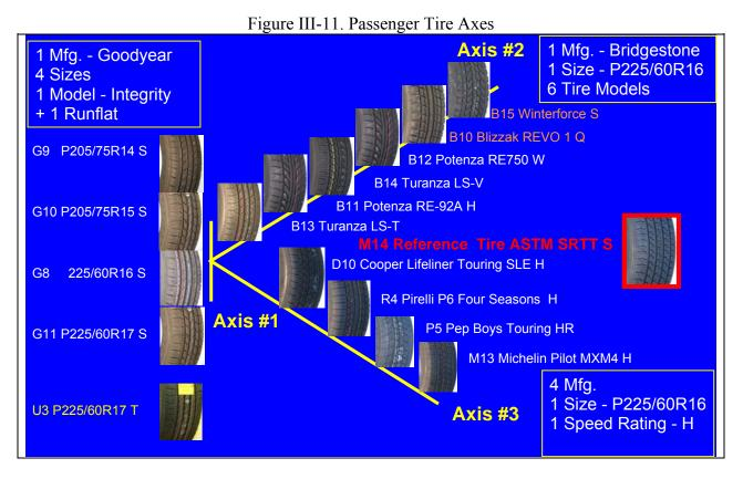
When possible, tires were tested on wheels of the corresponding "measuring rim width" for their size. Wheels of each size used in the test program were purchased new, in identical lots to minimize wheel-to-wheel variation. Tires participating in multiple tests at the same lab or between two labs were mounted once on a single wheel and continued to be tested on that same wheel until completion of all tests.
