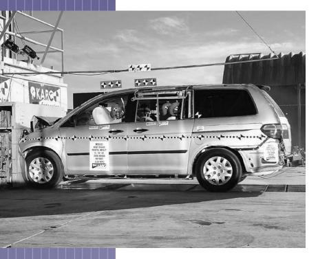
Using engineering principles and techniques, NHTSA conducts biomechanical research on impact injuries. Based on this knowledge, the agency develops crash test dummies, injury test criteria, and performance limits to provide the best possible safety for people in crash situations. A complete "family" of crash test dummies — including infants, children, adolescents, adults, and pregnant women — is used to ensure that all safety systems required by NHTSA regulations provide protection for everyone.
