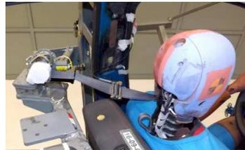
**Relocated Retractor 3-Point Belt (i.e. Seat Integrated)**
