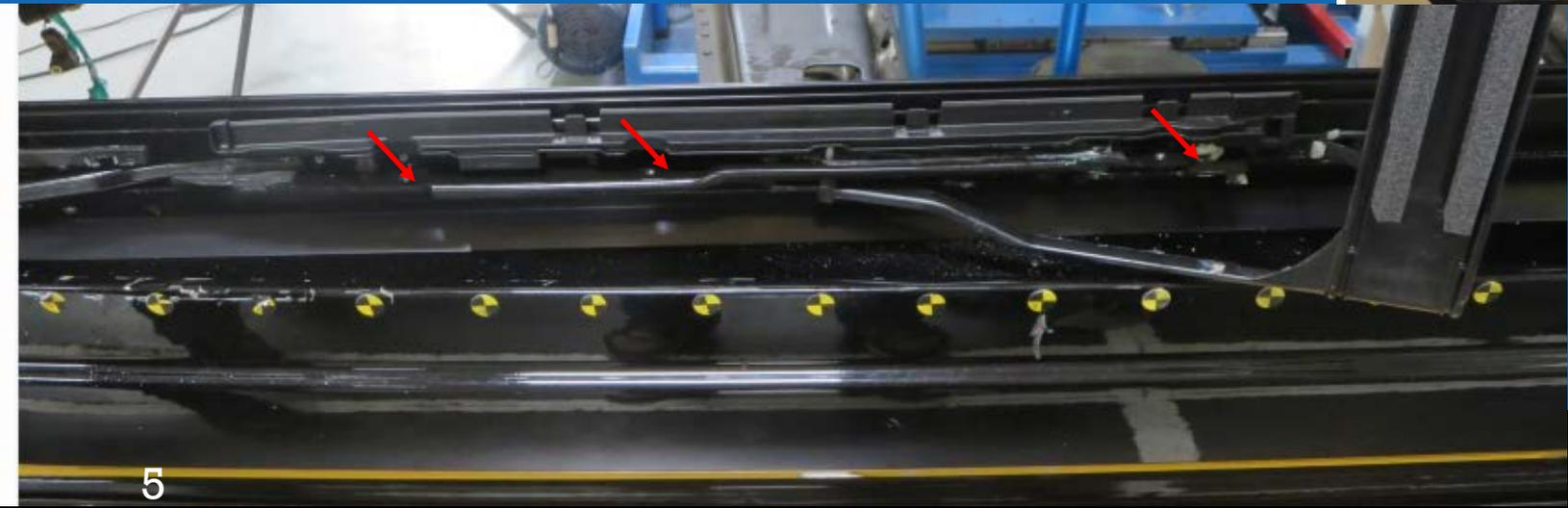
Panel attached (6 screws) from the outside to rails that moves in a C channel
