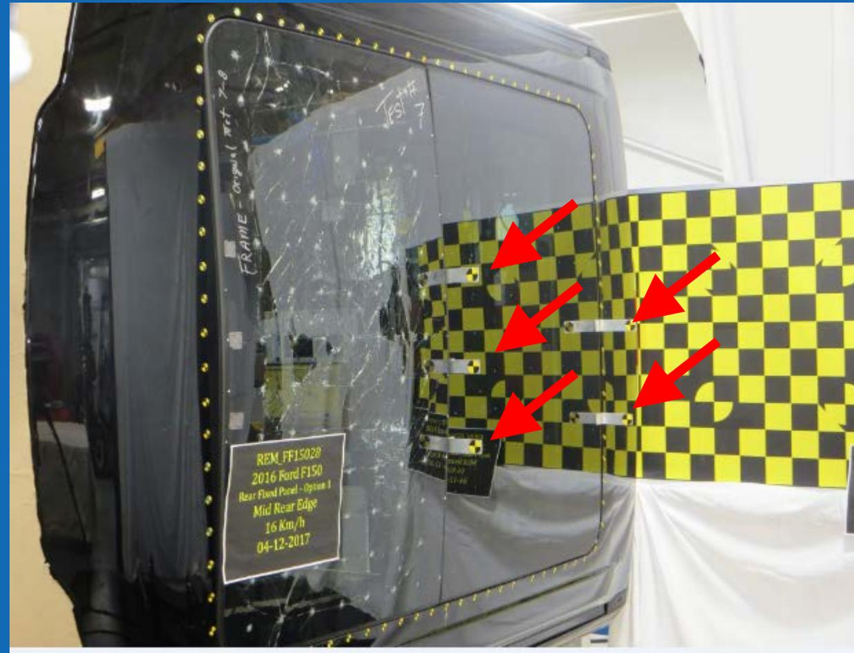
Targets at unsupported edges to measure dynamic excursion using photogrammetry (TEMA)
