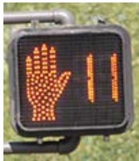
**Figure 22. Pedestrian countdown signal. (Source: *Resident's Guide for Creating Safer Communities for Walking and Biking*).**
