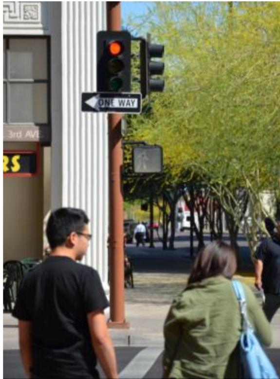
**Figure 29. This Leading Pedestrian Interval in Phoenix, Arizona, gives pedestrians a five second head-start before drivers get a green light. Note that the pedestrian WALK indication is on while the motorists are still briefly held with a red light. (Source: Federal Highway Administration, *Designing for Pedestrian Safety Course 201*).**
