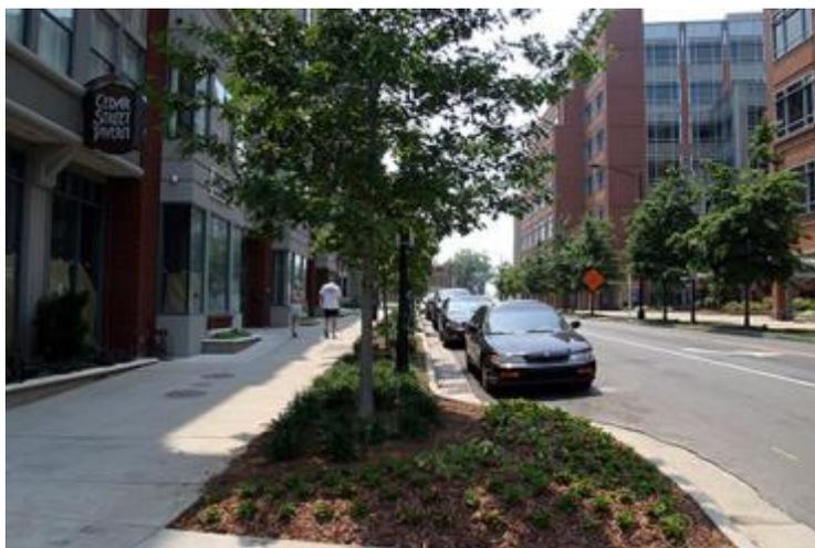
**Figure 27. Sidewalk with landscaped buffer and curb extension.**
