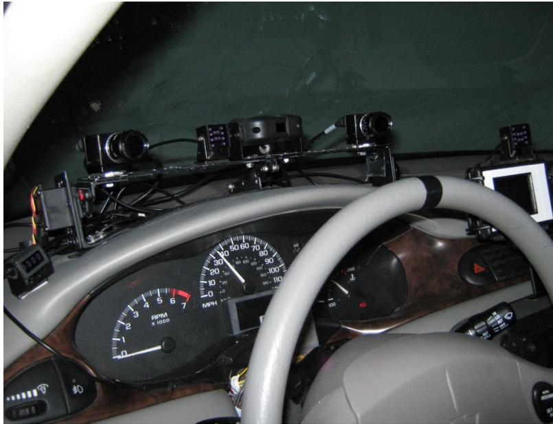
Figure 6. Face Lab Cameras Mounted in the Malibu Cab with a Separate Head Tracking System Mounted between Them
