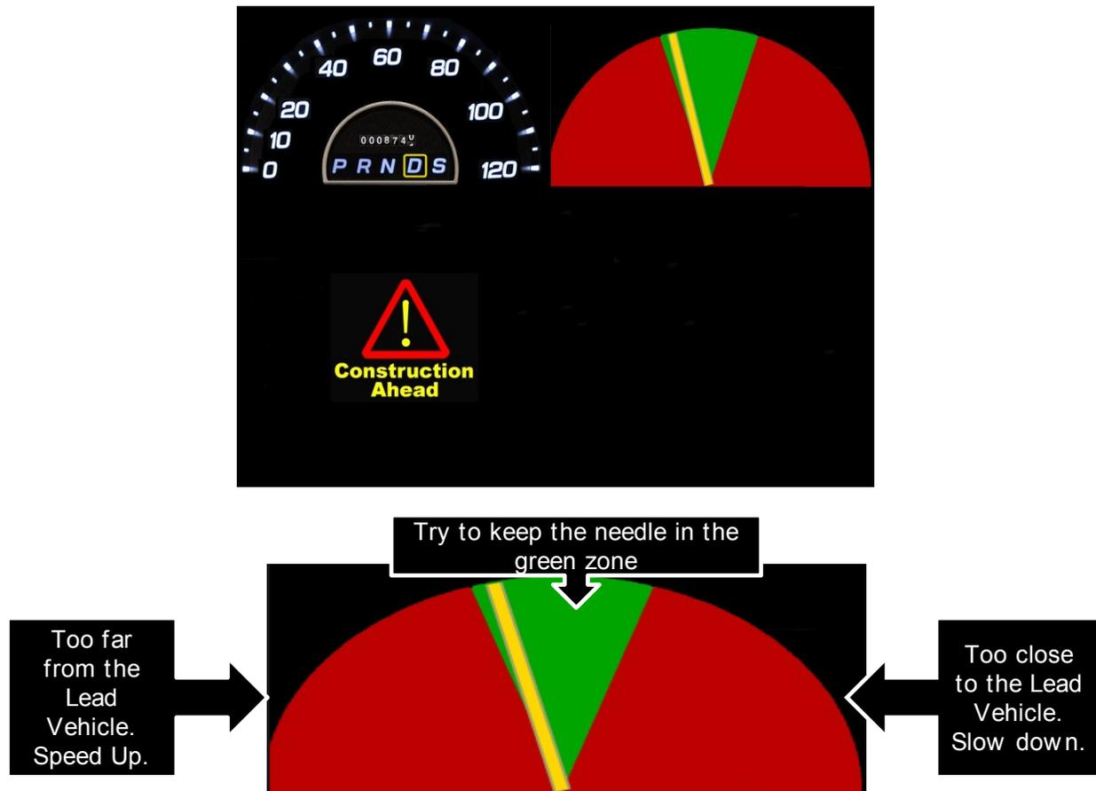
**Figure 4. Headway Display Gauge (Upper Right)**
