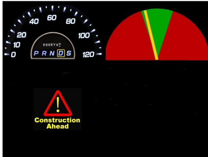
**Figure 3. Headway Display Gauge (Upper Right); Early Alert Icon (Lower Left)**
