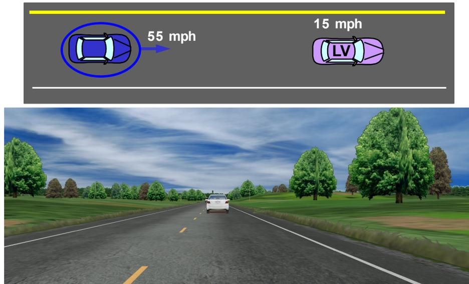
**Figure 2. Example Lead Vehicle Critical Braking Event**
