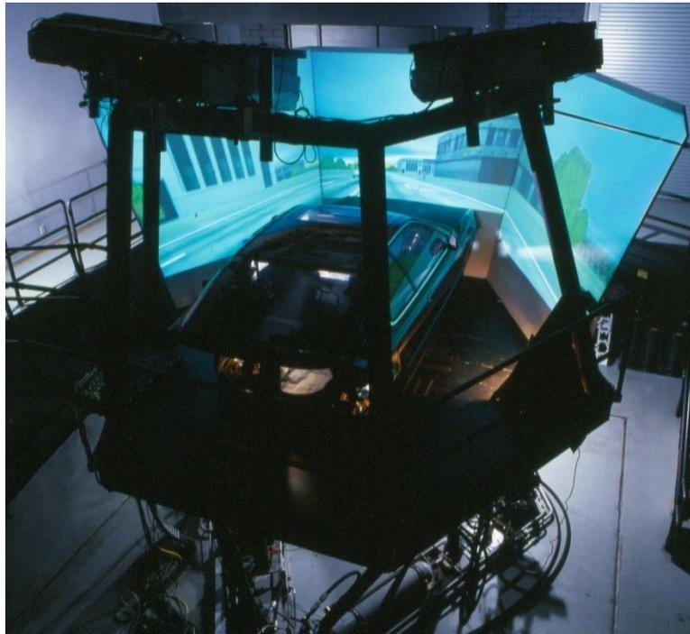
**Figure 1. DRI Motion Based Simulator**
