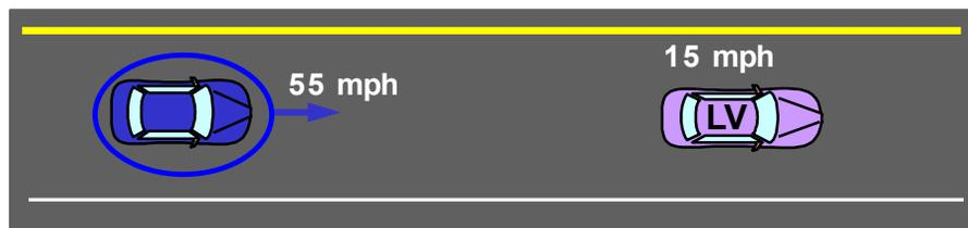
**Figure 2. Example Lead Vehicle Critical Braking Event**
