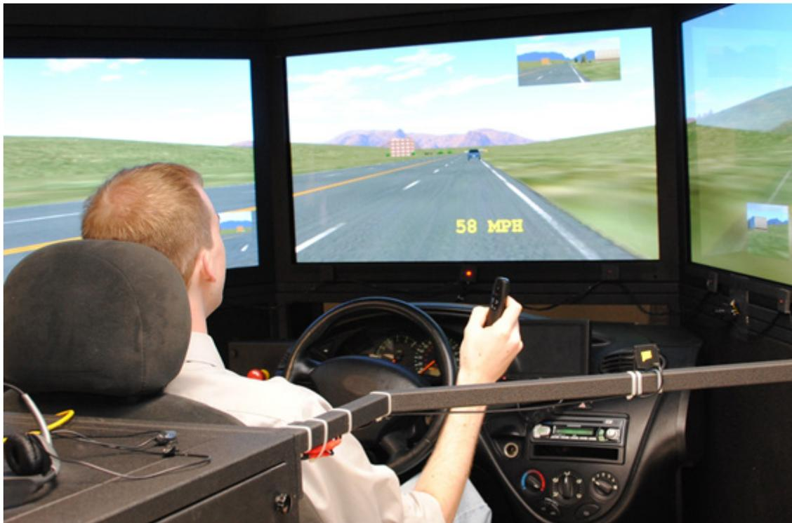
**Figure 1. GMU Driving Simulator illustrating LED lights for the peripheral detection task and response apparatus.**
