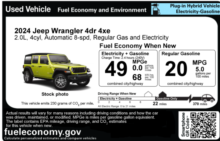
Figure C.2.3-2. Fuel Economy Label for the 2024 Jeep Wrangler 4xe Plug-in Hybrid Showing the Electricity and Gasoline Miles-per-Gallon Equivalent (MPGe) 33
