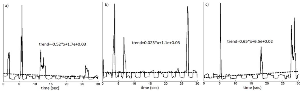
Figure 21 Trend information for 30-second segments of driving with visual task: a) negative slope; b) zero slope; c) positive slope. The conversion from pixels to angles could be done through 1:0.05 ratio.
