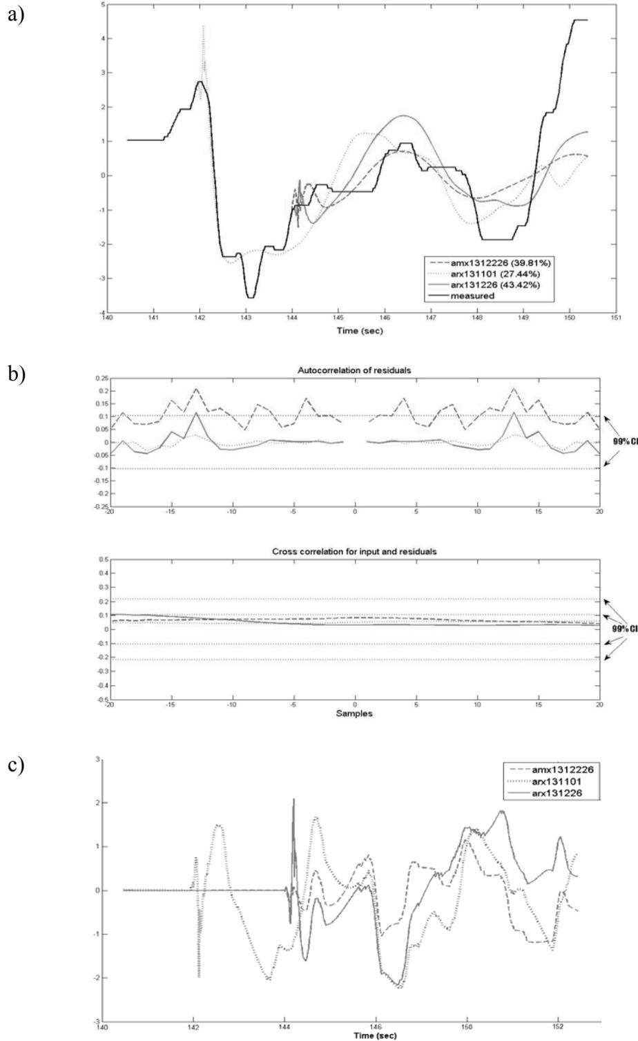
Figure 16 Comparison of candidate models for baseline driving: a) simulated and measured output comparison with Best Fit values; b) auto- and cross- correlation for residuals (the horizontal scale is the number of lags (samples) between the signals at which the correlation is estimated); and c) measured minus simulated output (error).
