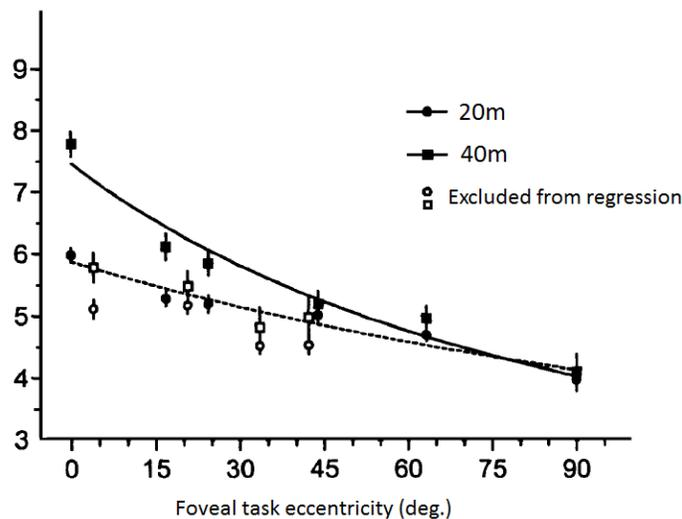
Figure 3 Mean time-to-collision at the point of brake application (in seconds) as a function of foveal task eccentricity for 20 m and 40 m headways (Lamble et al., 1999).
