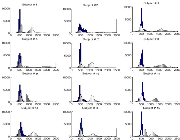
Figure 12 Distribution of (a) steering angle and (b) horizontal eye position for non-distracted (dark bars) and visually distracted (white bars) conditions
