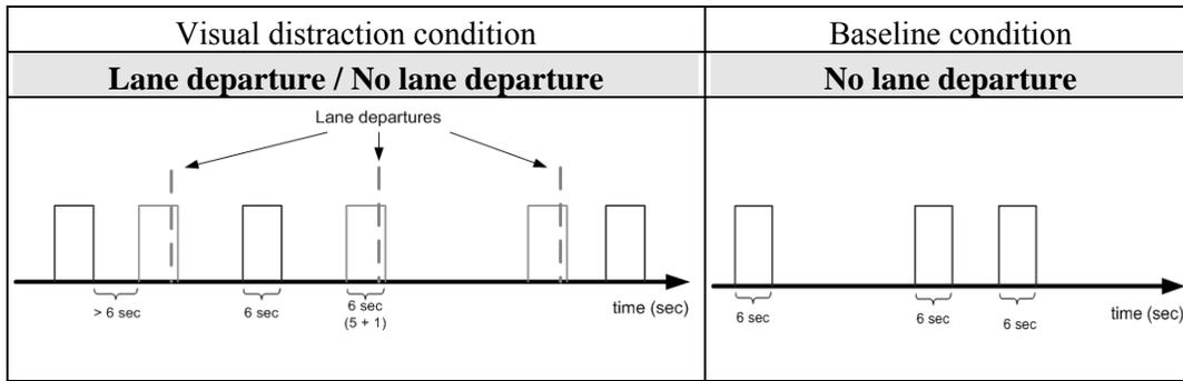
Figure 31 Samples of 6-second segments represent baseline and visually distracted driving with and without lane departures. Lane departures (see vertical dashed lines) are shown at the fifth second of the sample due to the method of triggering the selected sample. This allows each lane departure to have at least five seconds of history associated with it.
