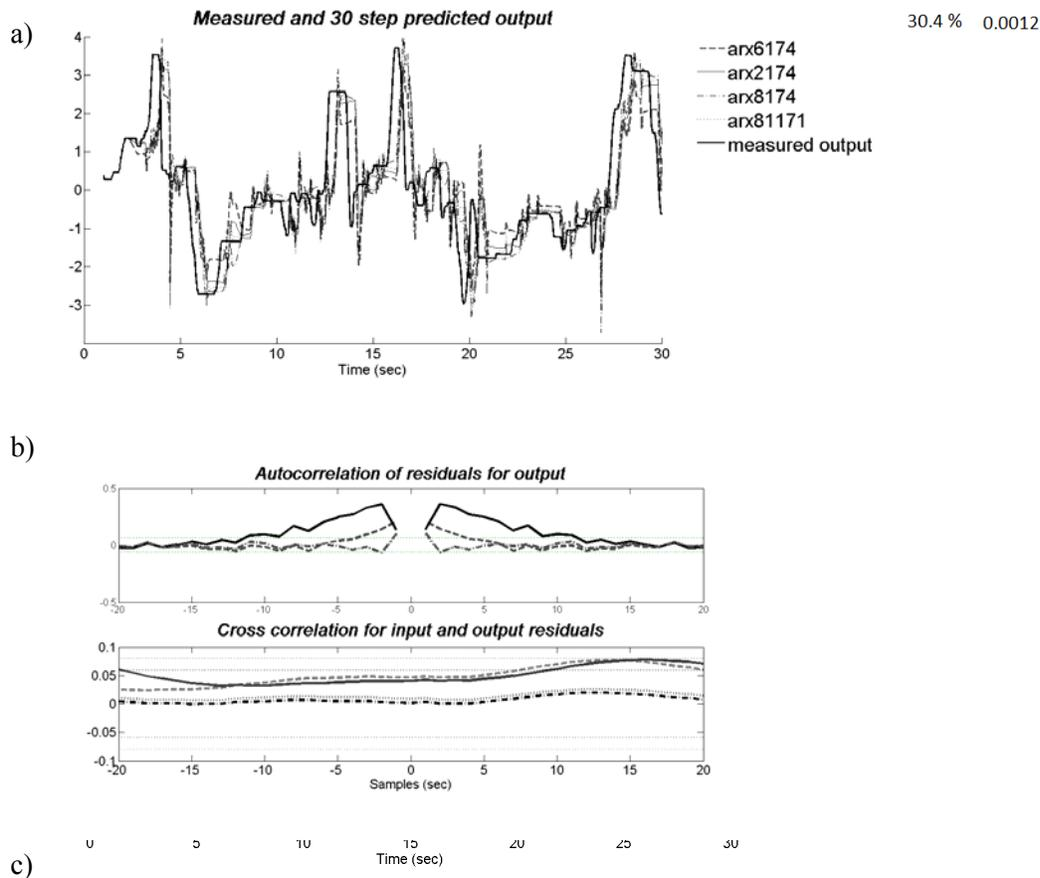
Figure 23 Comparison of candidate models for non-distracted driving of Subject 1: a) 30 steps ahead predicted and measured output comparison; b) auto- and cross- correlation for residuals (the horizontal scale is the number of lags (samples) between the signals at which the correlation is estimated); and c) residuals (error).
