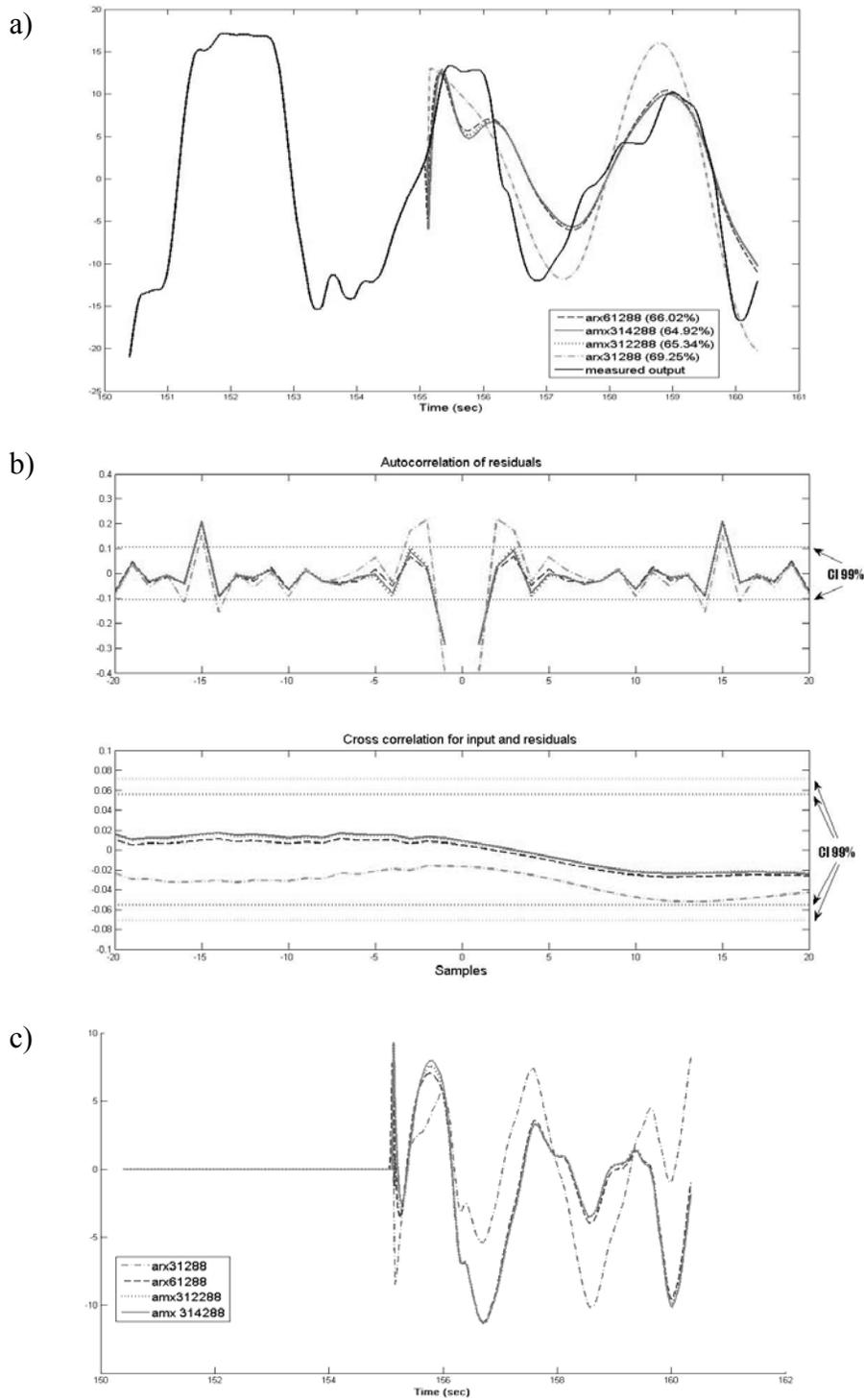
Figure 18 Comparison of candidate models for distracted driving (with visual task): a) simulated and measured output comparison with *Best Fit* values; b) auto- and cross- correlation for residuals (the horizontal scale is the number of lags (samples) between the signals at which the correlation is estimated); and c) measured minus simulated output (error).
