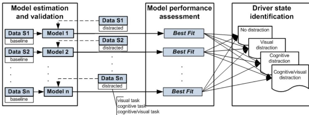
Figure 19 Schema of model development and driver state identification through model performance for a single driver (step 1). Step 2, when the data of non-distracted and distracted driving from all the drivers are applied to each model, is not shown on the schema.
