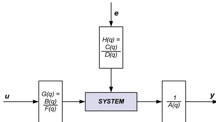
Figure 8 General linear model structure.
