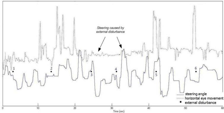
Figure 15 Steering angle and horizontal eye position (60-second sample of non-distracted driving)
