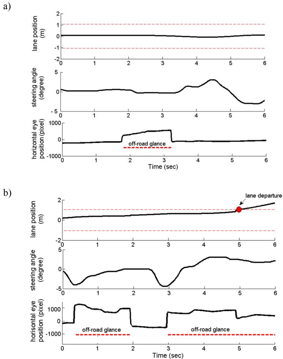
Figure 11 The sample of eye movements, steering responses, and lane position time series for (a) non-distracted and (b) distracted driving
