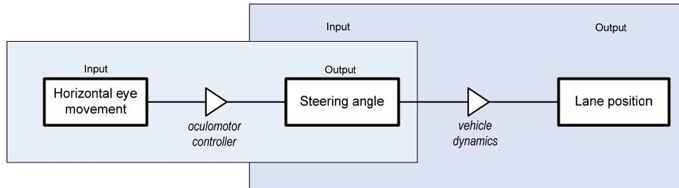
Figure 9 Eye movement – steering – lane position relationship.
