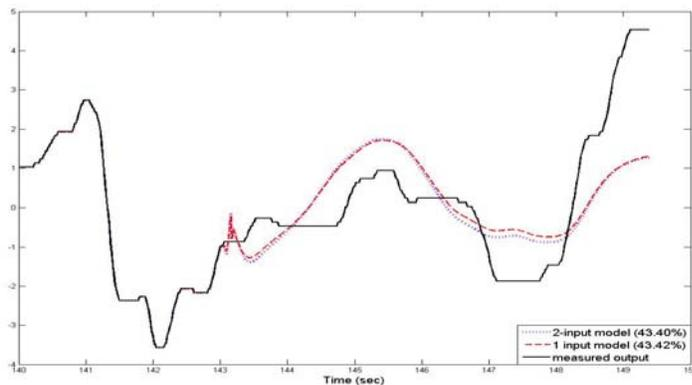
Figure 17 Comparison of SISO (one-input) and MISO (two-input) models.
