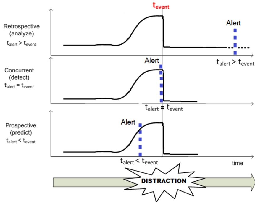
Figure 10 Comparison of the different timelines for distraction indication. Time of event is associated with the time of maximum risk of crash caused by distraction.
