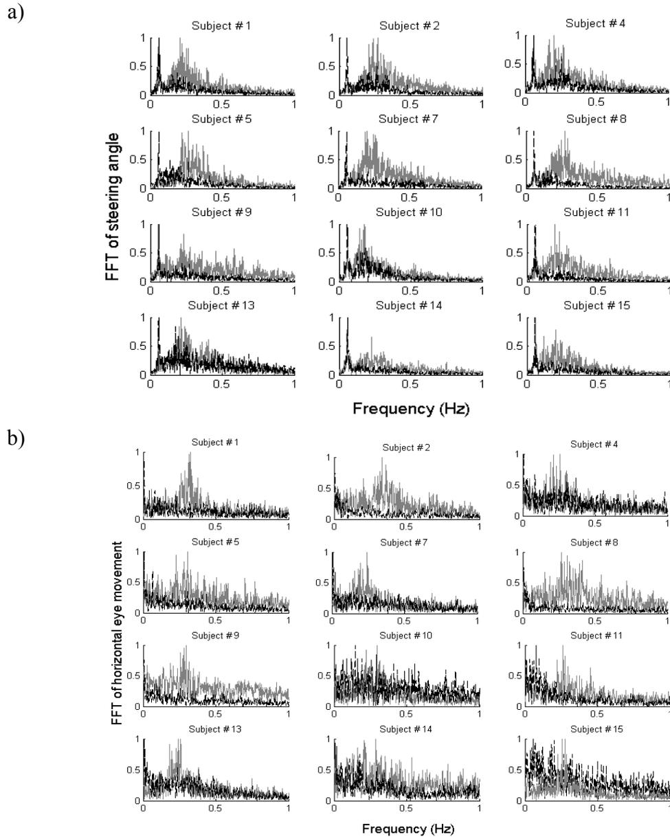
Figure 13 Detrended (a) steering angle and (b) horizontal eye position spectra for non-distracted (dashed black line) and distracted (gray solid line) conditions
