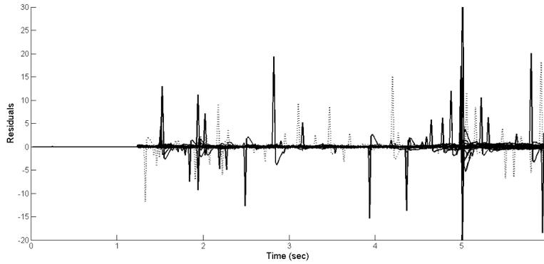
Figure 32 The residuals (predicted minus measured output) for two groups of segments with (solid line) and without (dotted line) lane departures for the visual distraction condition.
