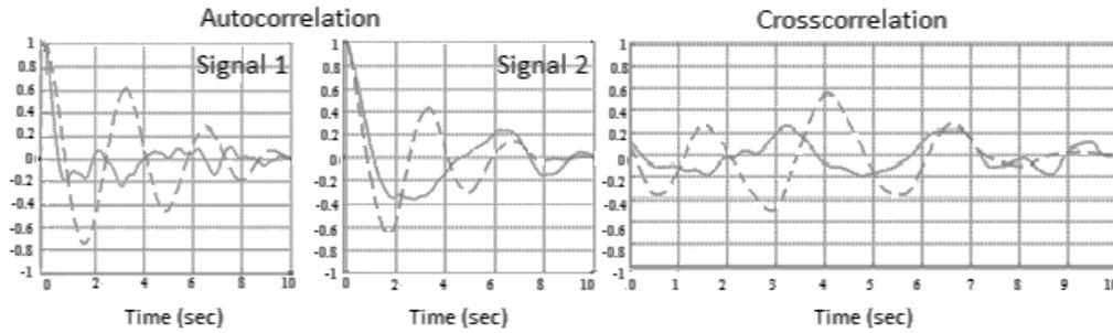
Figure 14 Auto- and cross- correlation functions calculated for eye and steering signals for 10-second segments of non-distracted (solid line) and distracted (dashed line) conditions
