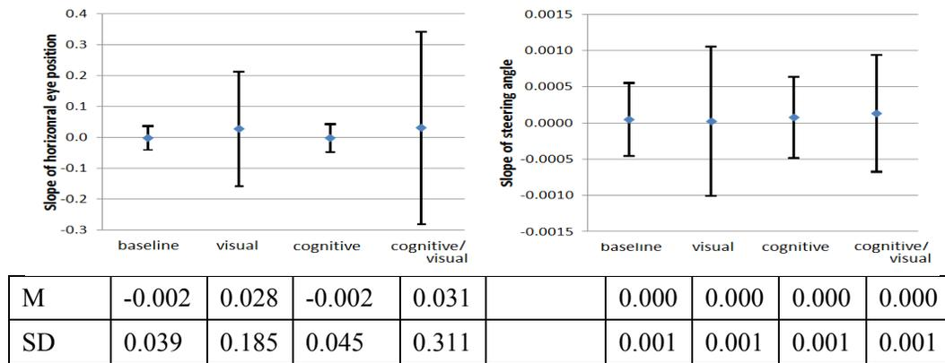
Figure 20 Slope statistics: mean values (with standard deviation bar) for non-distracted and distracted driving.
