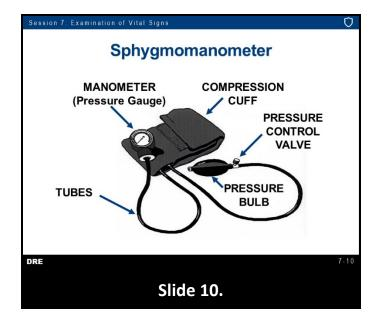
The device used for measuring blood pressure is called a sphygmomanometer. The sphygmomanometer has a special cuff that can be wrapped around the subject's arm and inflated with air pressure.
