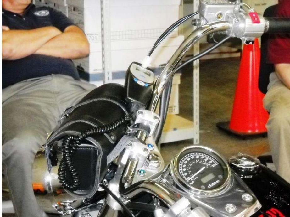
**Figure 13: Handlebar secure pouch with interlock at rest atop**
