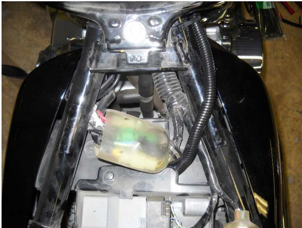
**Figure 12: Seat removed, battery hookup connectors**
