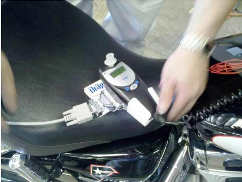
**Figure 15: Arrangement for download of data to computer via handset**
