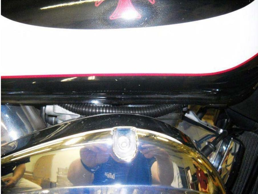
**Figure 11: Wire cable runs beneath the fuel tank toward the battery**
