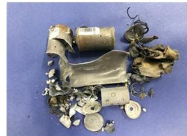
Figure 7. Degradation observed in -X series inflators under laboratory accelerated cycling conditions leading to an inflator rupture.
