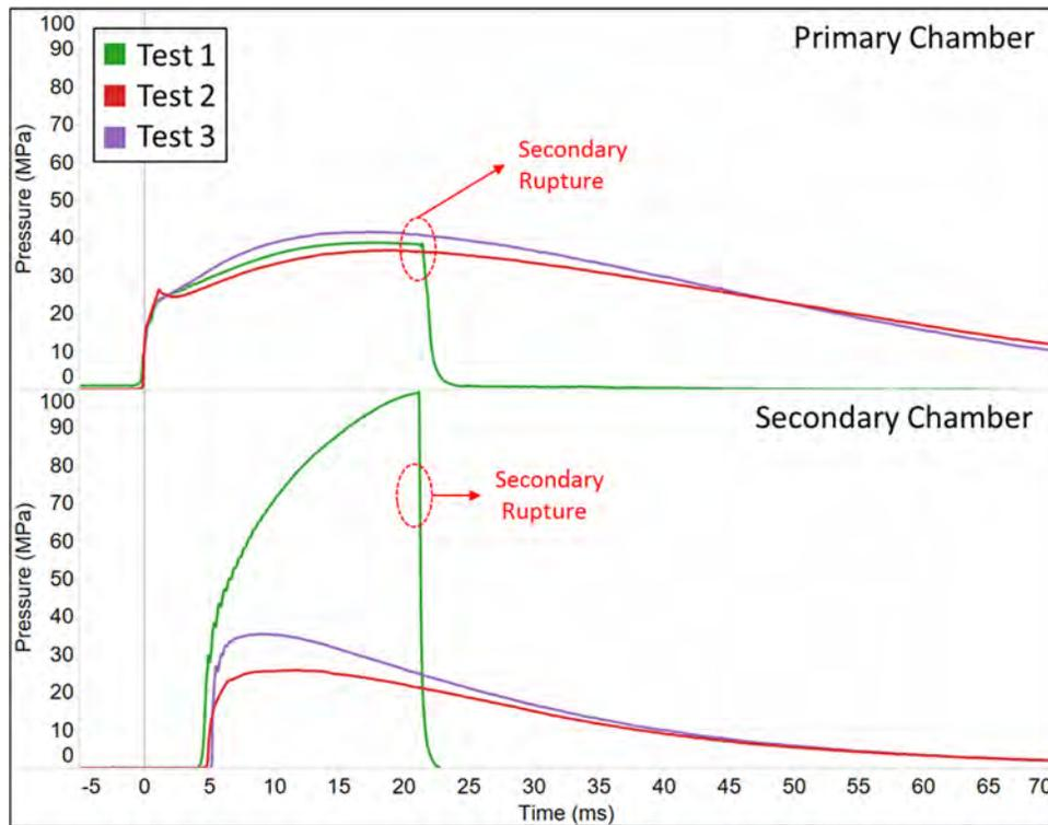
Figure 15. Inflator pressure-time history of virgin PSPI-L inflators cycled 800 times (2-80°C, 4 hours/cycle).
