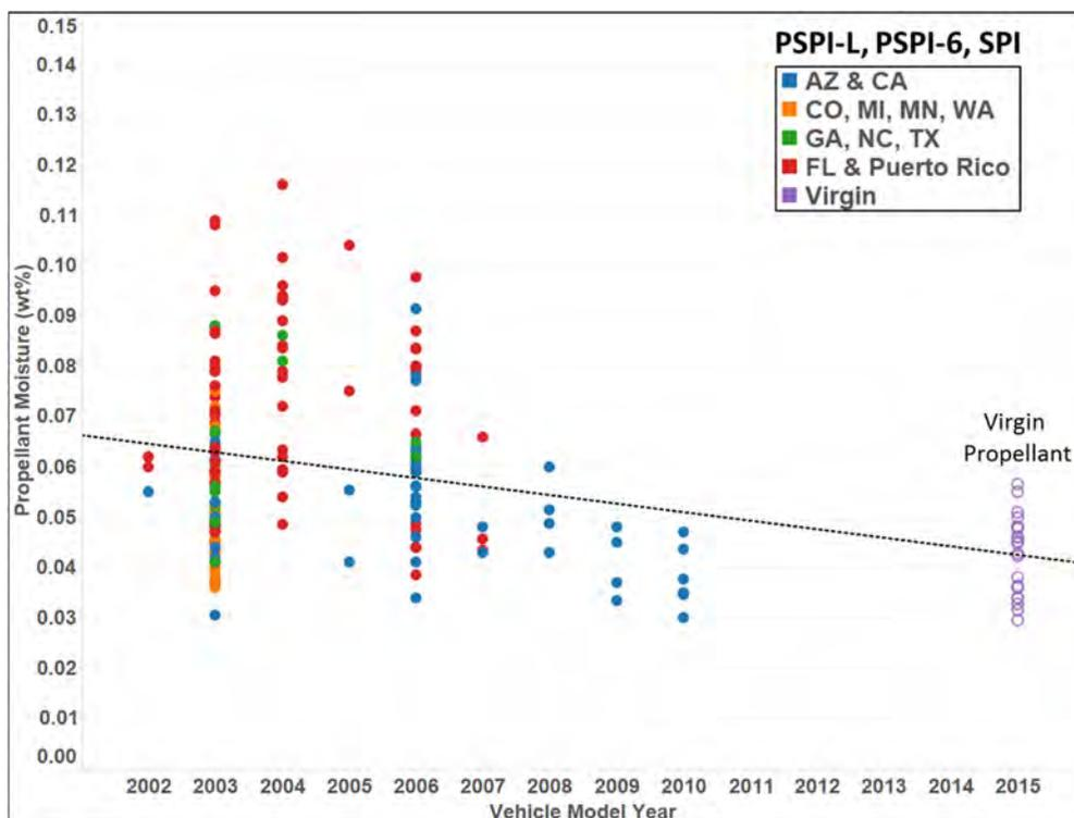
Figure 4. Moisture content in the 2004 propellant in various field returned inflators. (Data from the primary and secondary chambers are shown. The dotted line shows a linear fit through all of the presented data.)
