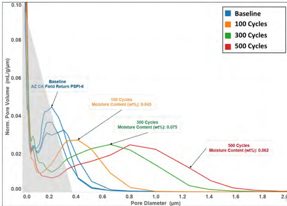
Figure 16. MIP pore size distribution of field returned 2004 propellant cycled (2-95°C, 3 hours/cycle) in 77 mL chambers. (The baseline data were obtained from the population of 2007 model year Arizona and California field samples that were used in the subsequent cycling.)
