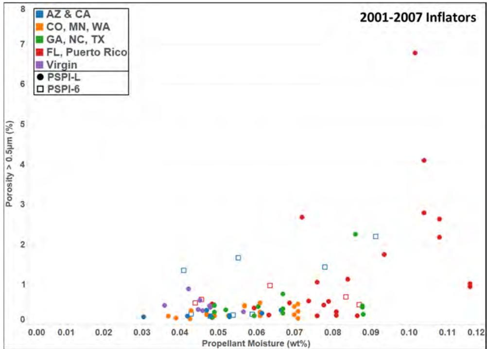
Figure 7. MIP porosity versus propellant moisture for 2001-2007 inflators from selected states.
