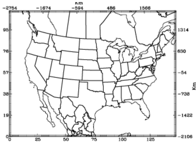
Figure D.1.2-1. CMAQ Modeling Domain for the NHTSA Phase 2 MDHD Air Quality Modeling Analysis (Horizontal Grid Spacing is 36 kilometers [22.4 miles])
