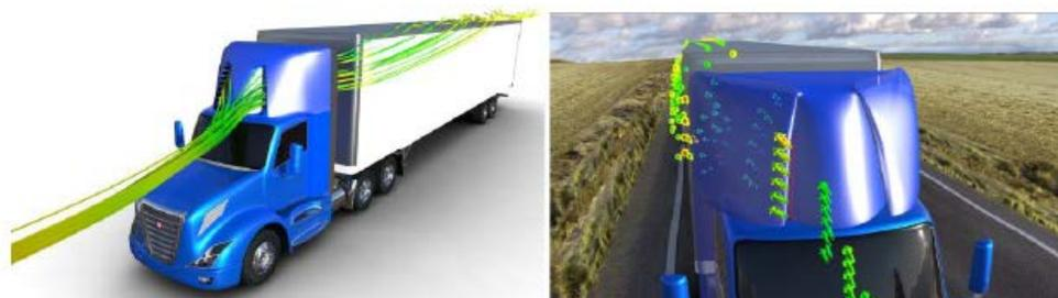
Figure 3: SABIC concept roof fairing showing directed airflow
