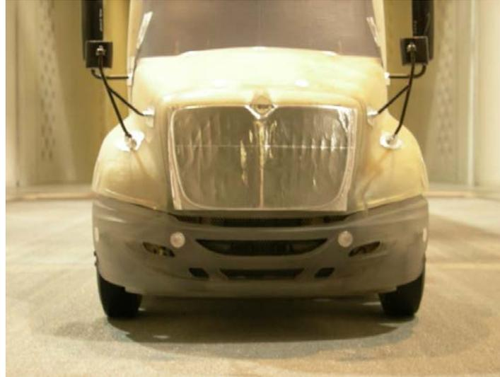
**Figure 2-8 Photo of 1/8th Scale Model of a Tractor with the Front, External Grille Covered With Aluminum Tape to Simulate A Closed Grille Configuration**
