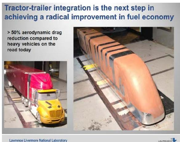
**Figure 2-11 Pictures Showing Future Heavy-Duty Tractor Trailer Concept to Achieve >50 percent Aerodynamic Improvement for Class 8 Line Haul Heavy-Duty Vehicles**
