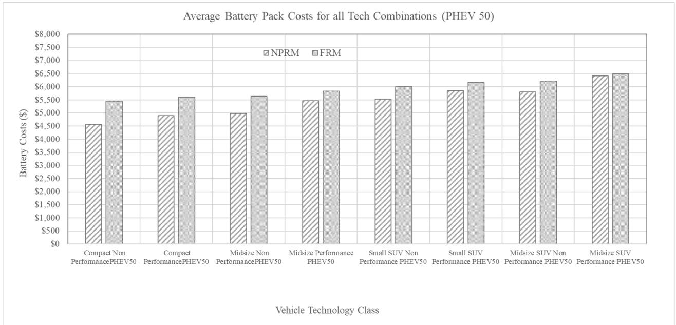
Figure VI-41 - Comparing PHEV50 Average Battery Costs (Costs do not include RPE or Learning Curve Adjustment)
