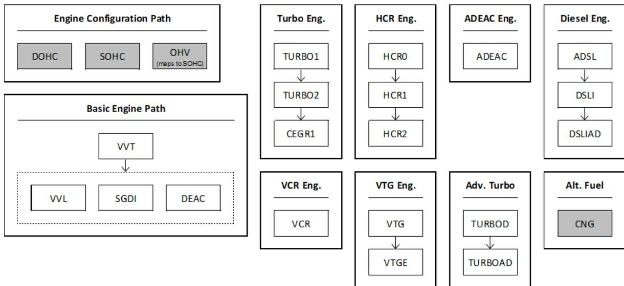
Figure VI-19 – Engine Paths Used for the Final Rule Analysis
