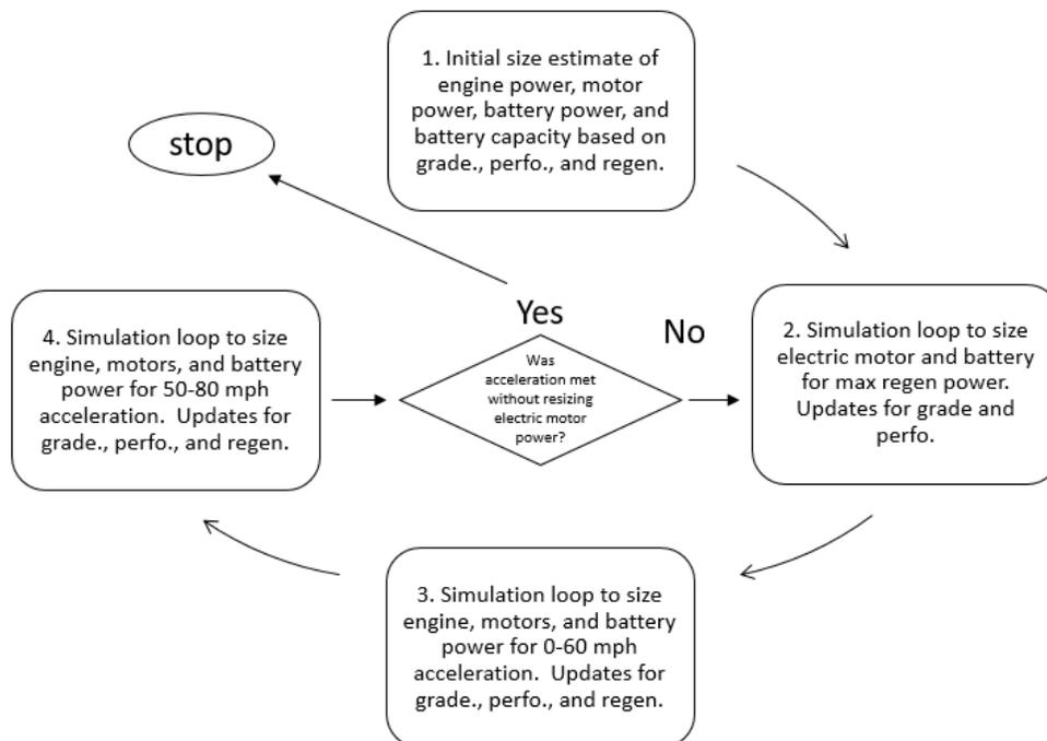
Figure VI-33 – Simplified SHEVP2 Sizing Algorithm in Autonomie
