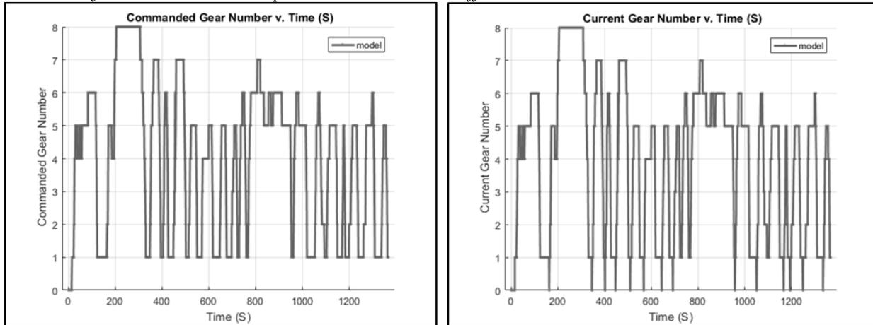
Figure VI-6 – Comparison of Commanded Gear Shift versus Actual Gear Shift for the UDDS<sup>622</sup>
