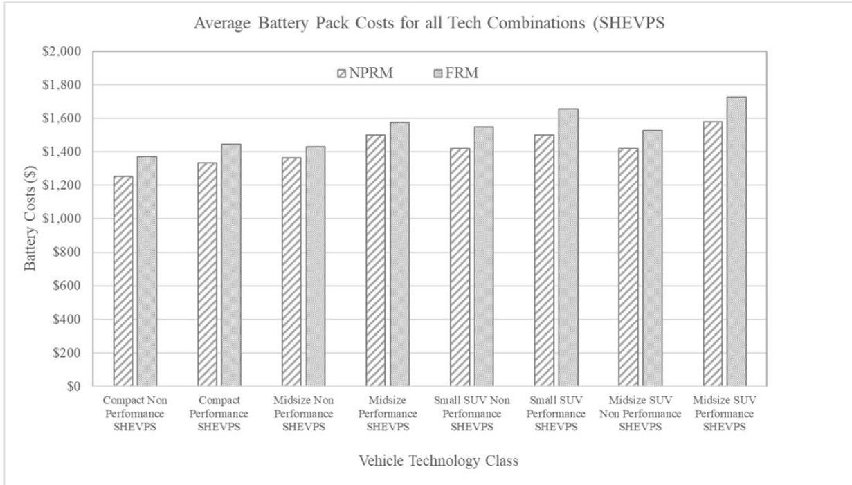
Figure VI-40 – Comparing SHEVPS Average Battery Costs (Costs do not include RPE or Learning Curve Adjustment)
