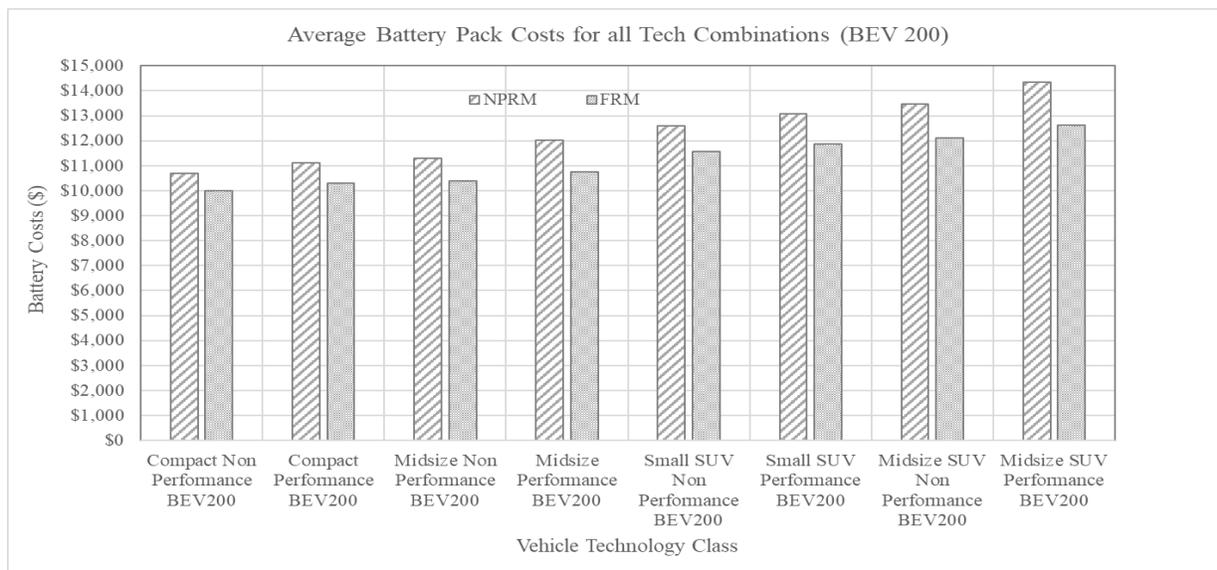
Figure VI-42 – Comparing BEV200 Average Battery Costs (Costs do not include RPE or Learning Curve Adjustment)
