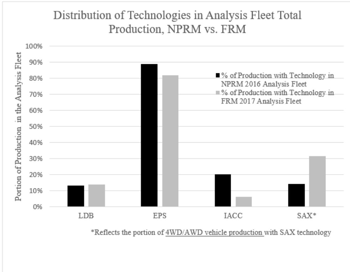
Figure VI-54 – Distribution of Technologies in Analysis Fleet Production
