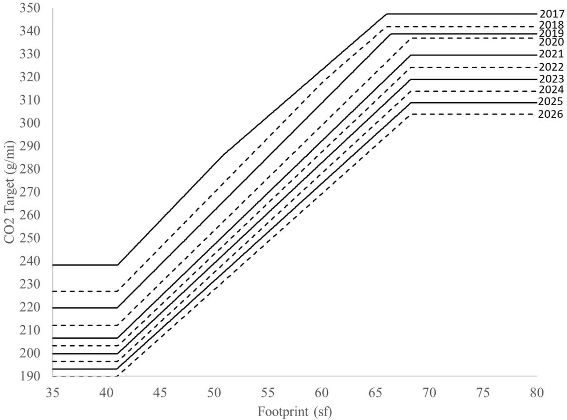
Figure II-4 – Light Truck CO<sub>2</sub> Targets
