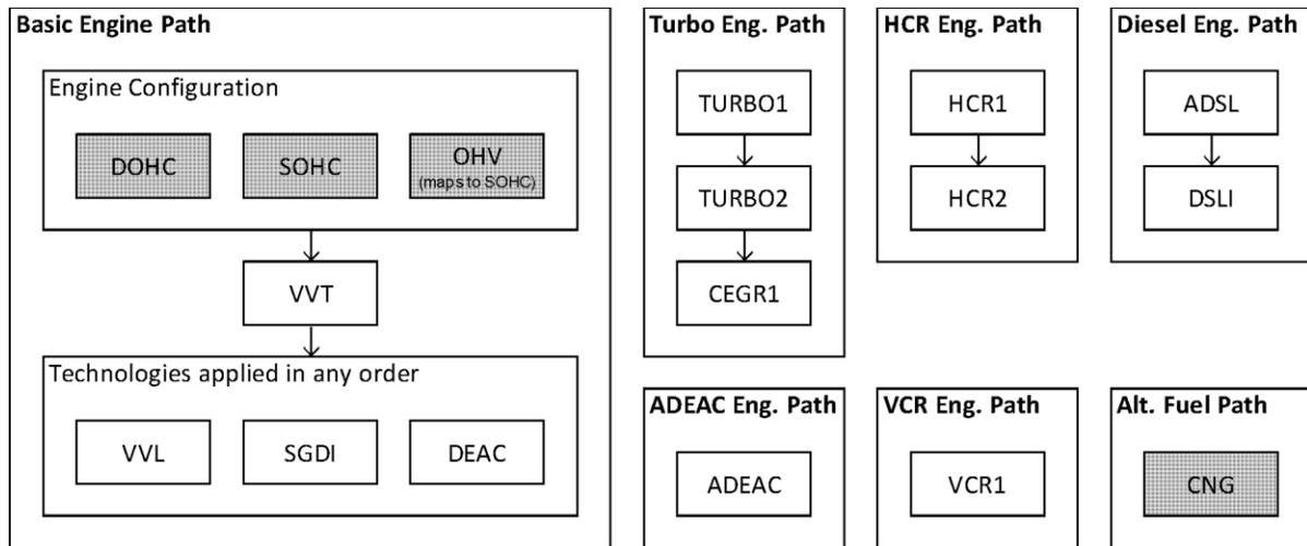
Figure VI-18 – Engine Paths Used for the NPRM Analysis
