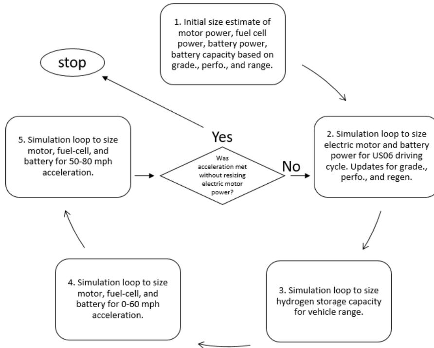
Figure VI-36 – Simplified Fuel Cell Vehicle Sizing Algorithm
