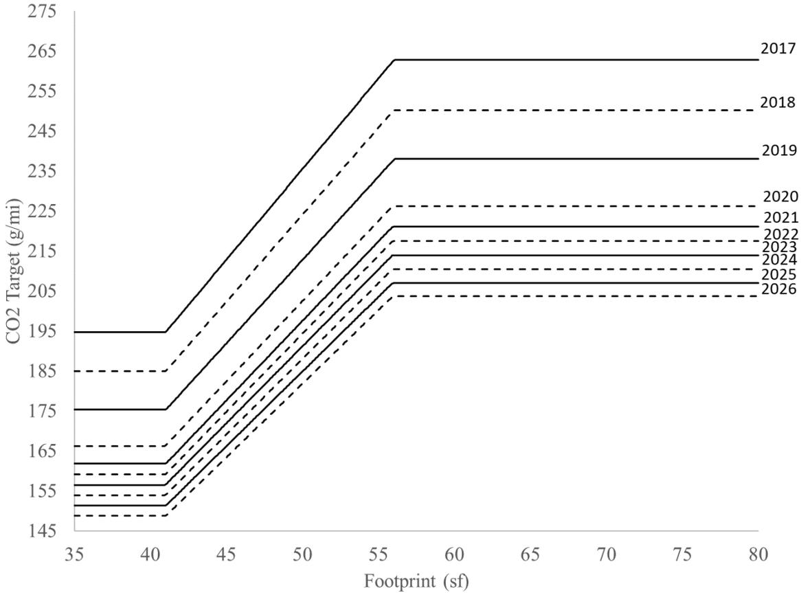
Figure II-3 – Passenger Car CO<sub>2</sub> Targets
