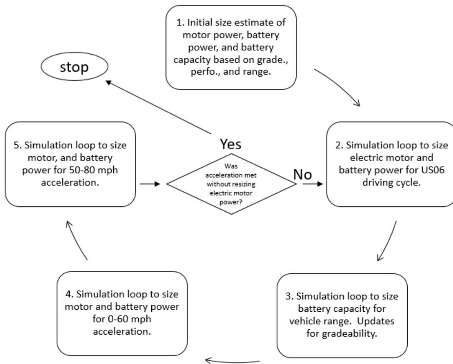
Figure VI-35 – Simplified BEV Sizing Algorithm in Autonomie
