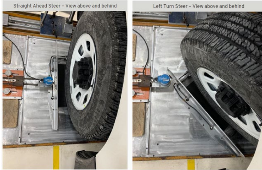
Figure 36. Road wheel angle measurement fixture
