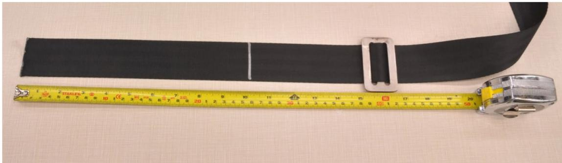
7. Thread the end of the webbing down through the split drum of the surrogate retractor until the 250 mm mark is visible. Then direct the webbing tail under the top framing bracket along the right side of the spindle.
