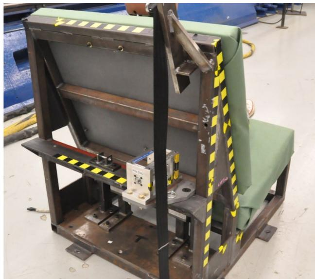
5. Turn the spindle 10 half turns (5 full rotations) to create the 213-specified belt tension. Note that the user should only turn the spindle in the direction indicated by the arrow on top of the retractor hardware, so that the spring will work correctly and not break. Once you have completed winding, pin the retractor using any pin slot. This will prevent rotation of the spindle while the belt is threaded through the retractor.
