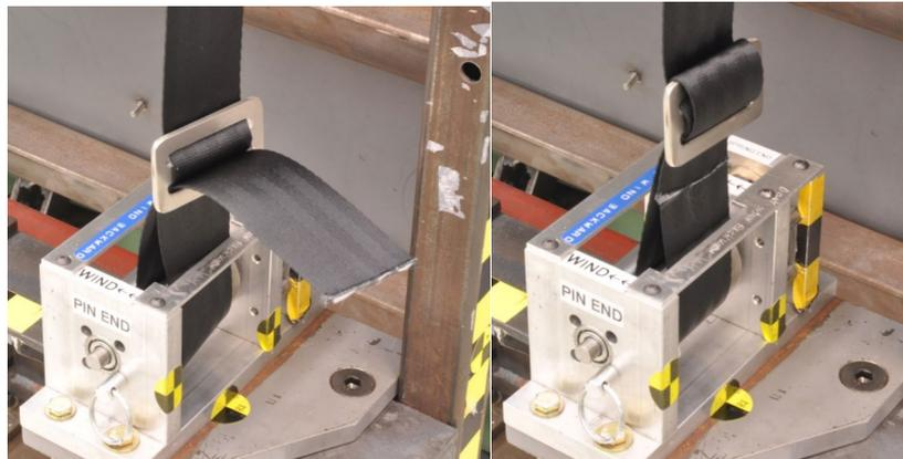
9. Hold the belt webbing above the 3-bar clip. Unpin the surrogate retractor and allow 50 mm (2 inches) of the webbing to wind back on the spindle by allowing the spindle to rotate one-quarter of a turn. (Note: the spring tension will turn the spindle opposite to the arrow direction, but this ok.) The quarter-turn change is represented in the photos below by the movement of the pink dot from the top to the right side of the spindle. Re-pin the retractor using any slot.
