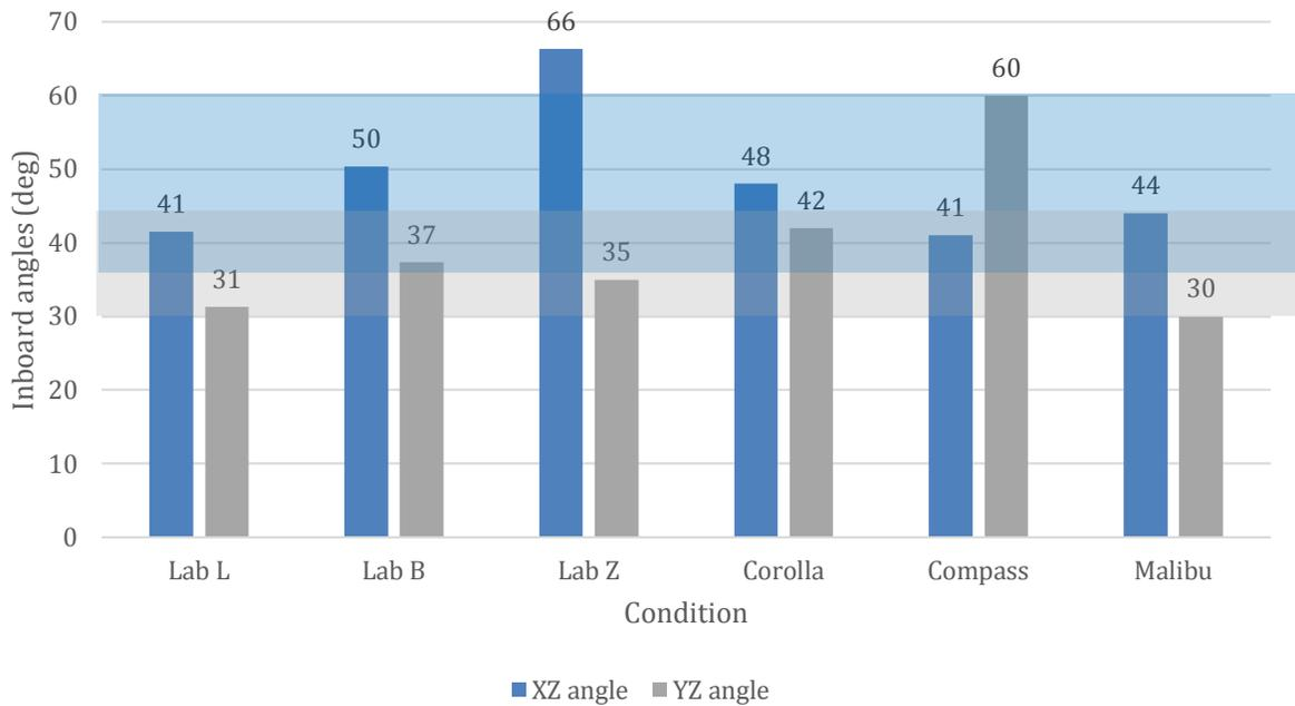
Figure 13. Inboard angles across vehicle and lab conditions, compared to fleet +/- 1STD.
