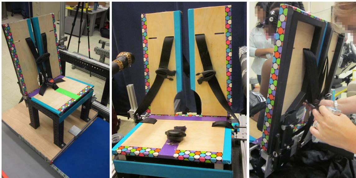
Figure 17. Hardseat used for measuring subject reference landmarks.
