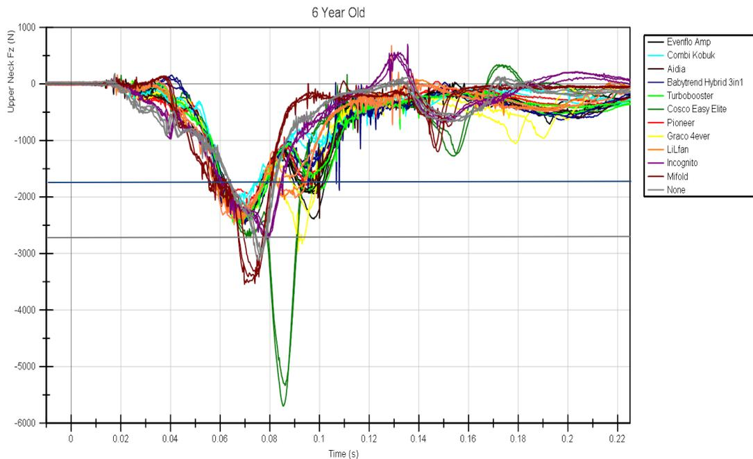
Figure 36. Neck axial load for 6YO tests.
