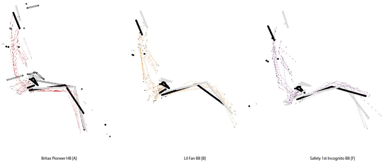
Figure C12. Comparison of postures of child volunteers with 10YO and small female across applicable booster configurations in MALIBUU vehicle. Cushion Length = 475 mm; Seat back angle = 23-deg; Cushion angle = 13-deg
