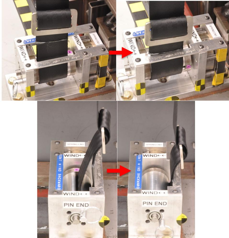
10. Secure the webbing at the outboard lap belt anchor, removing all excess belt from the system without shifting the ATD position.
