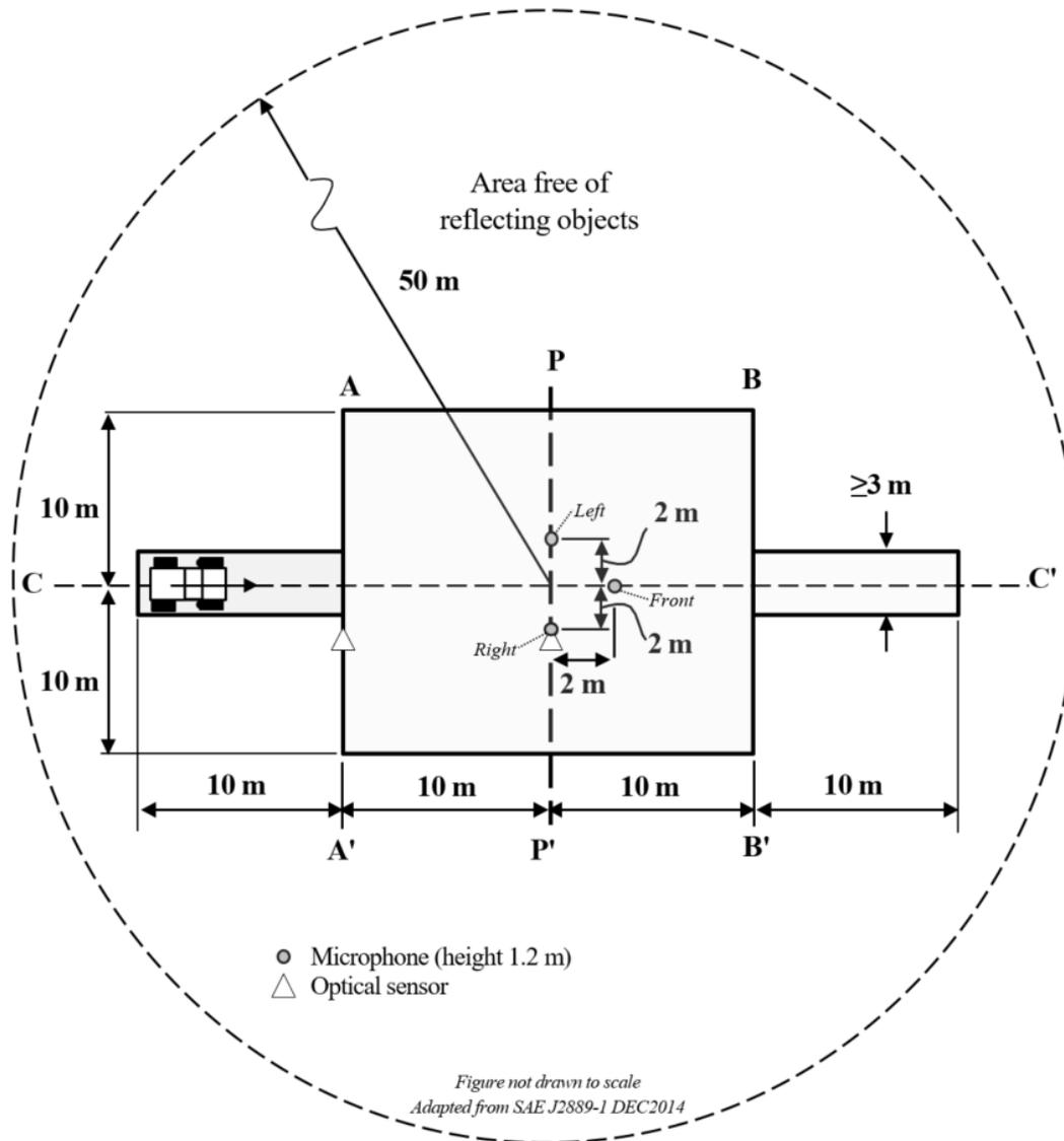
**Figure 1: Test site dimensions. Adapted from SAE J2889-1. Modifications include addition of a front microphone used only during stationary/directivity measures and optical sensors to record trigger signals for pass-by tests.**
