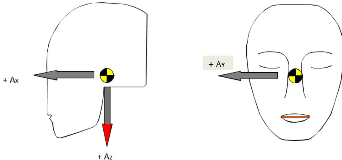
**Figure 5.** FMH Accelerometer Sign Convention
