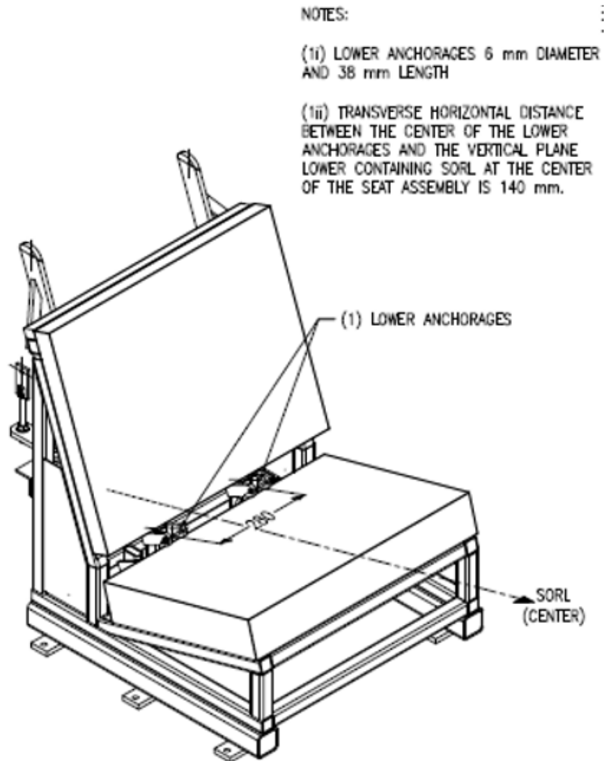
FIGURE 29. SORL AND LOCATION OF THE LOWER ANCHORAGES OF THE CHILD RESTRAINT ANCHORAGE SYSTEM ON THE FISA
