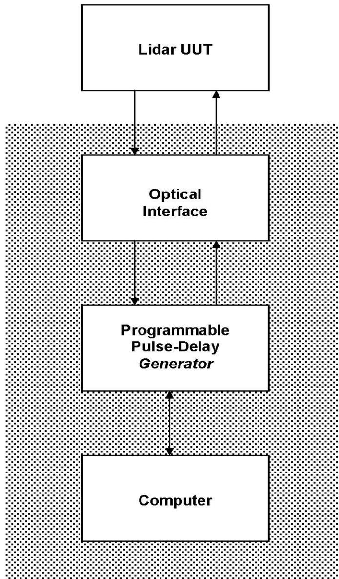
*Figure 1. Block diagram illustrating the Lidar Unit Under Test (Lidar UUT) interfaced with the Target Speed Simulator (TSS). The TSS is composed of three components: the Optical Interface, the Programmable Pulse-Delay Generator and the Computer.*
