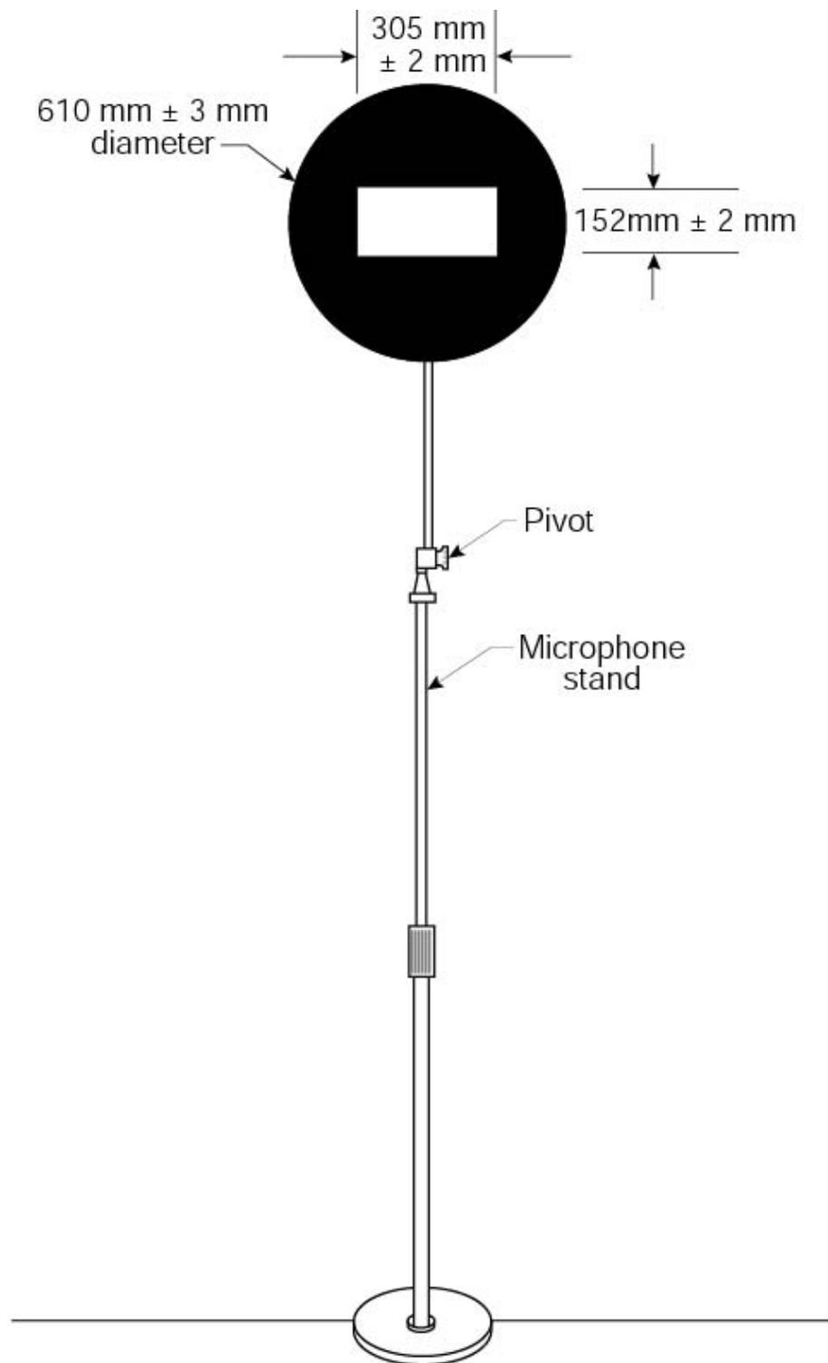
Figure 6. Schematic of the long-range target apparatus
