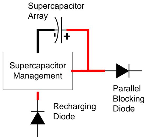
Figure 4-40. Simplified supercapacitor with charge and discharge management.
