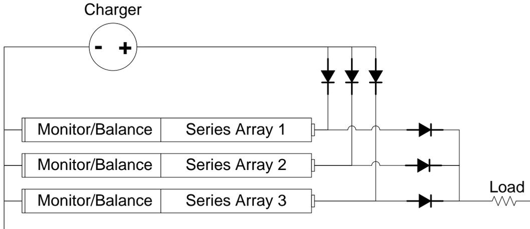
Figure 4-7. Simplified parallel array of series cells.
