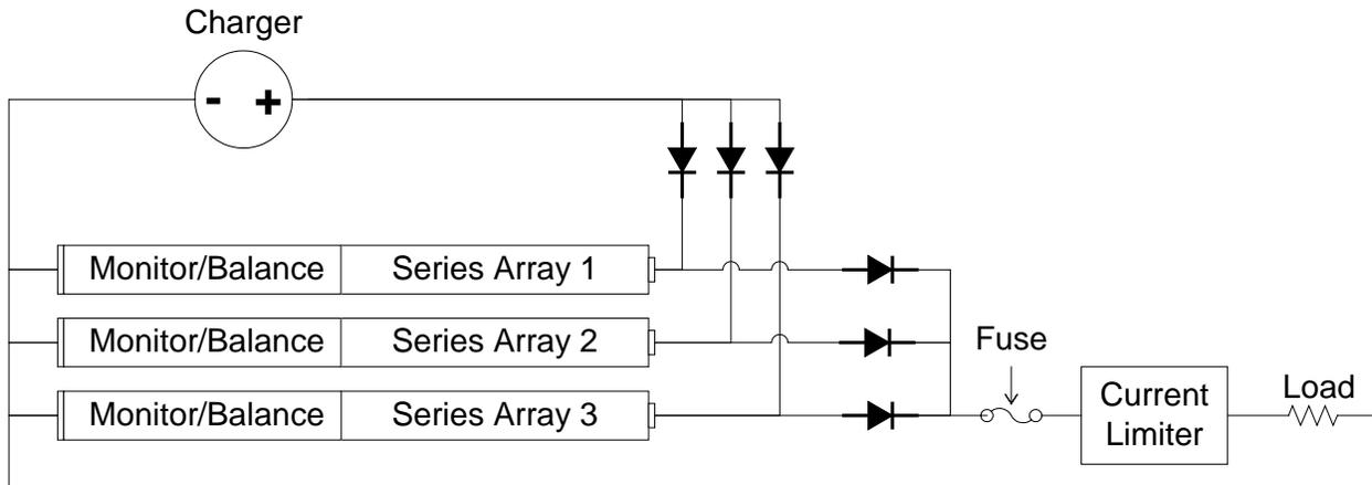
Figure 4-11. Battery module with one fuse per module.
