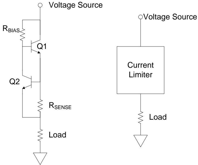
Figure 4-8. Simple current limiting circuit and general symbol.
