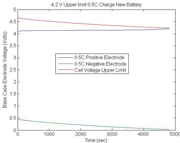
**Figure 7-3. Positive and negative electrode voltages at the separator interfaces for a charging rate of 0.5 C**
