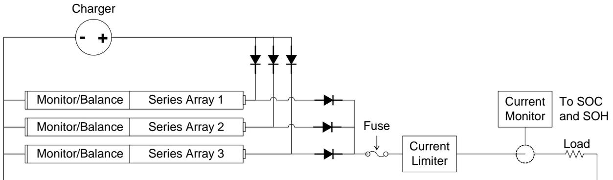
Figure 4-13. Battery module with one current monitor per module.
