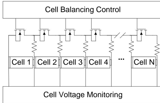
Figure 4-3. Series battery array with a charge control.
