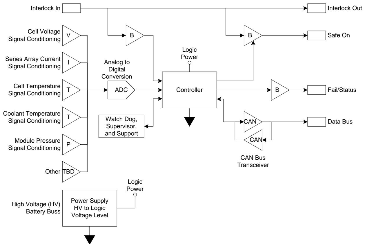
**Figure 4-27. Module control electronic block diagram elements.**
