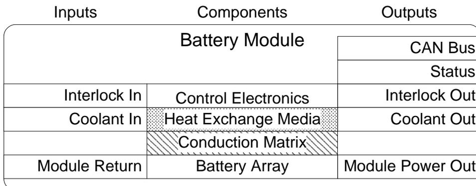
Figure 4-29. A compact model of a battery module.
