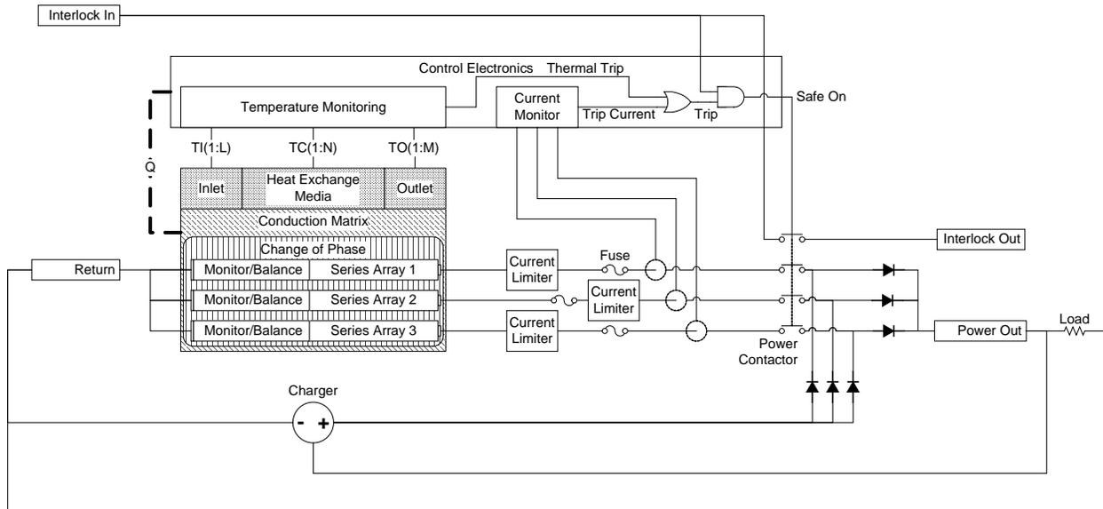
Figure 4-25. Module model with Interlock design elements.
