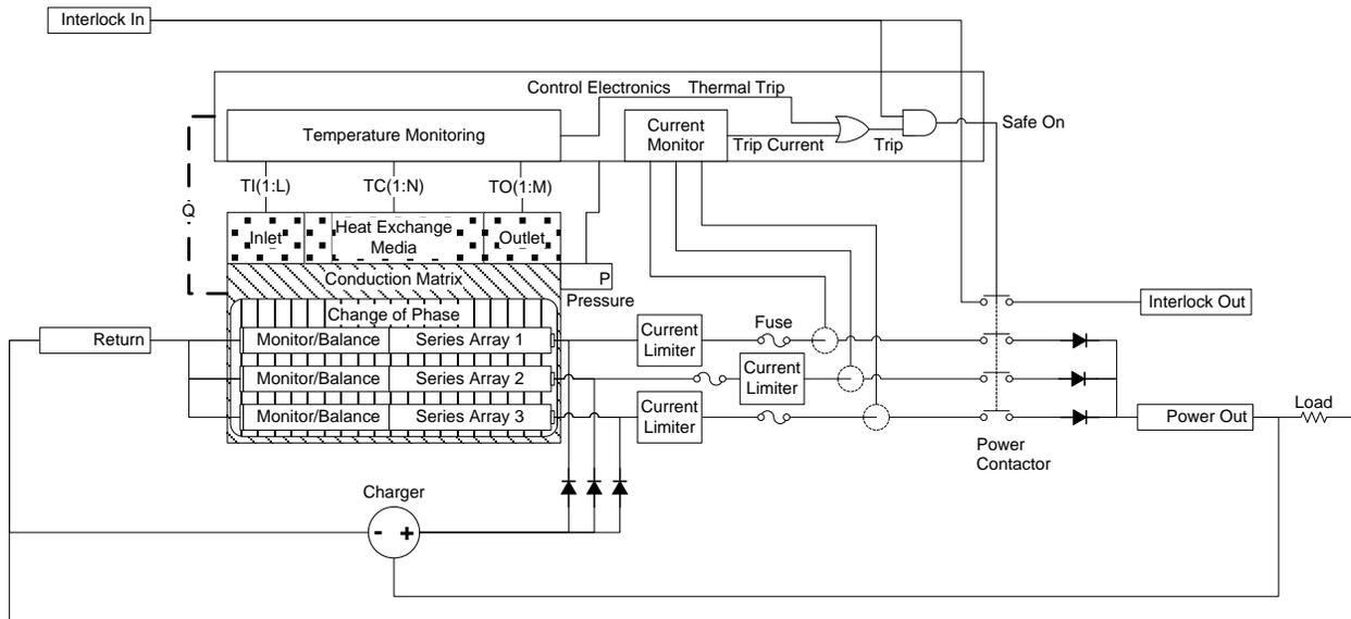
Figure 4-26. Module model with a pressure sensor.
