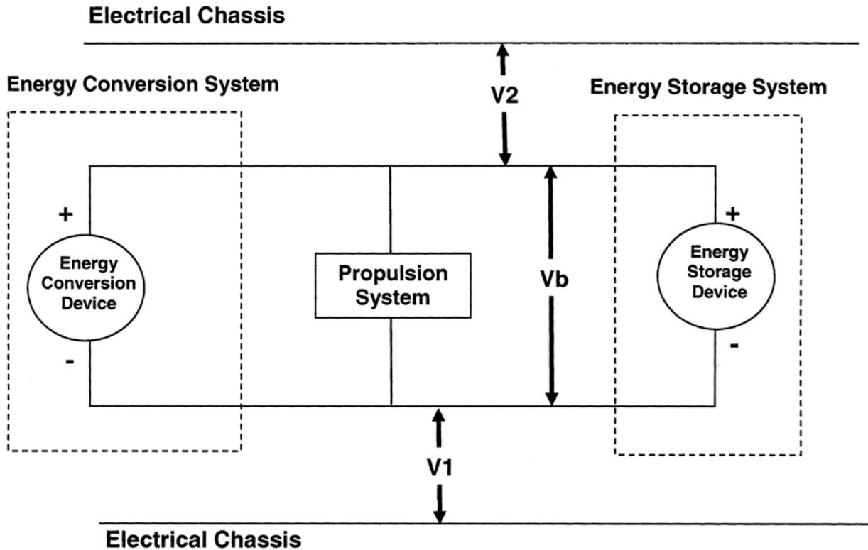
Figure 10-3. FMVSS 305 high-voltage system schematic (NHTSA 2011 Response).
