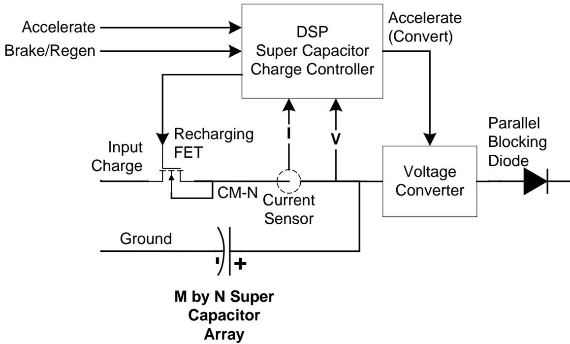
Figure 4-39. Supercapacitor array with recharge and discharge management.
