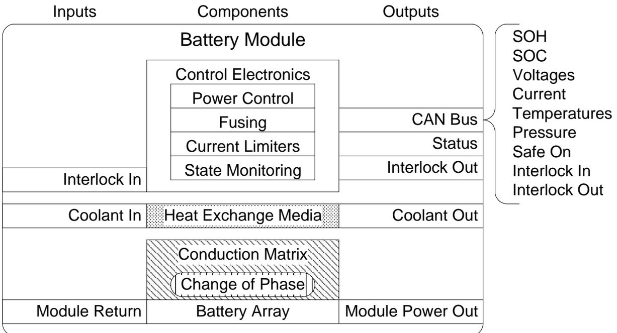
Figure 4-28. A complete model of a battery module.
