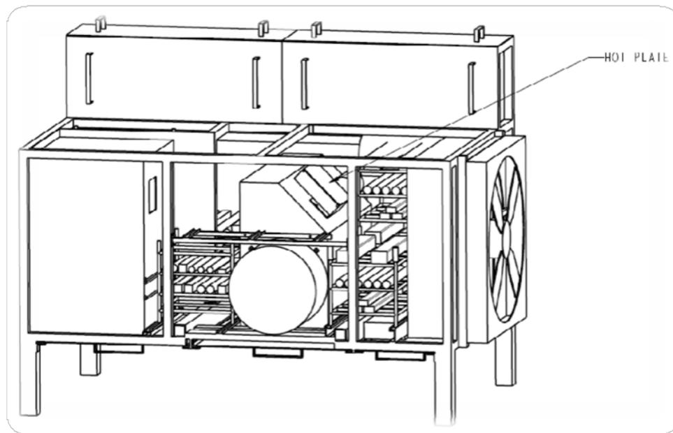
**Figure 4. Hot Surface Re-Ignition Fire Scenario (View of Forward Side).**
