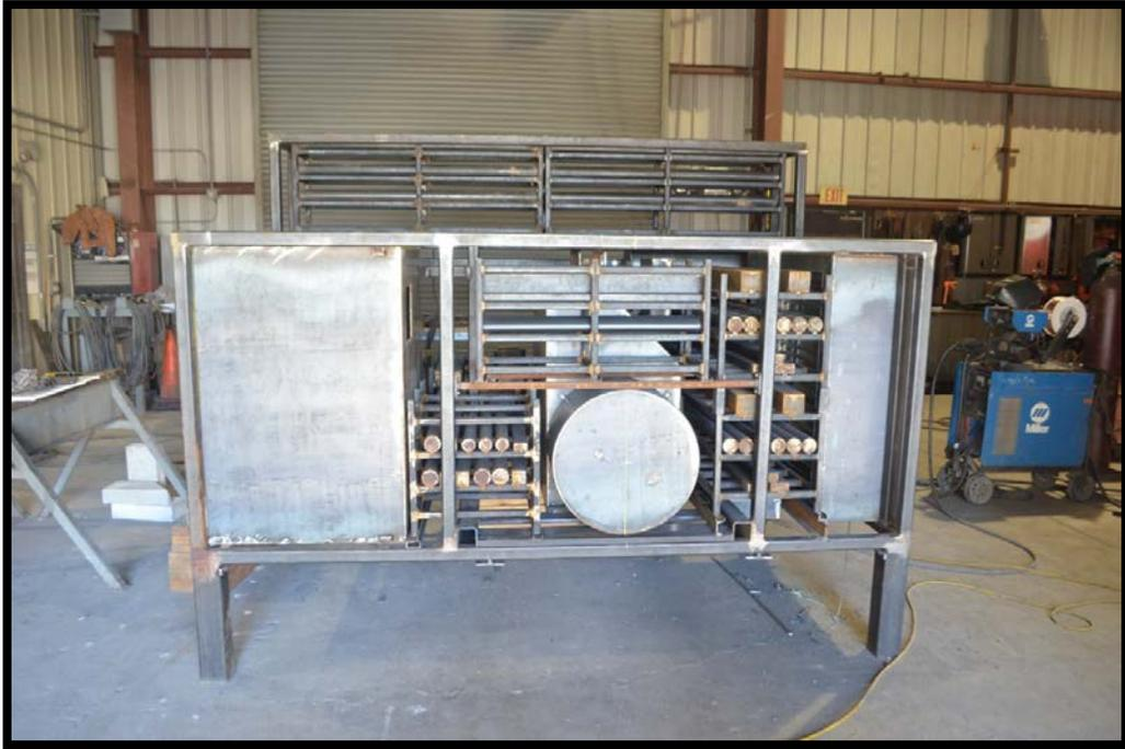
**Figure 19. Engine Compartment Mockup Test Fixture
