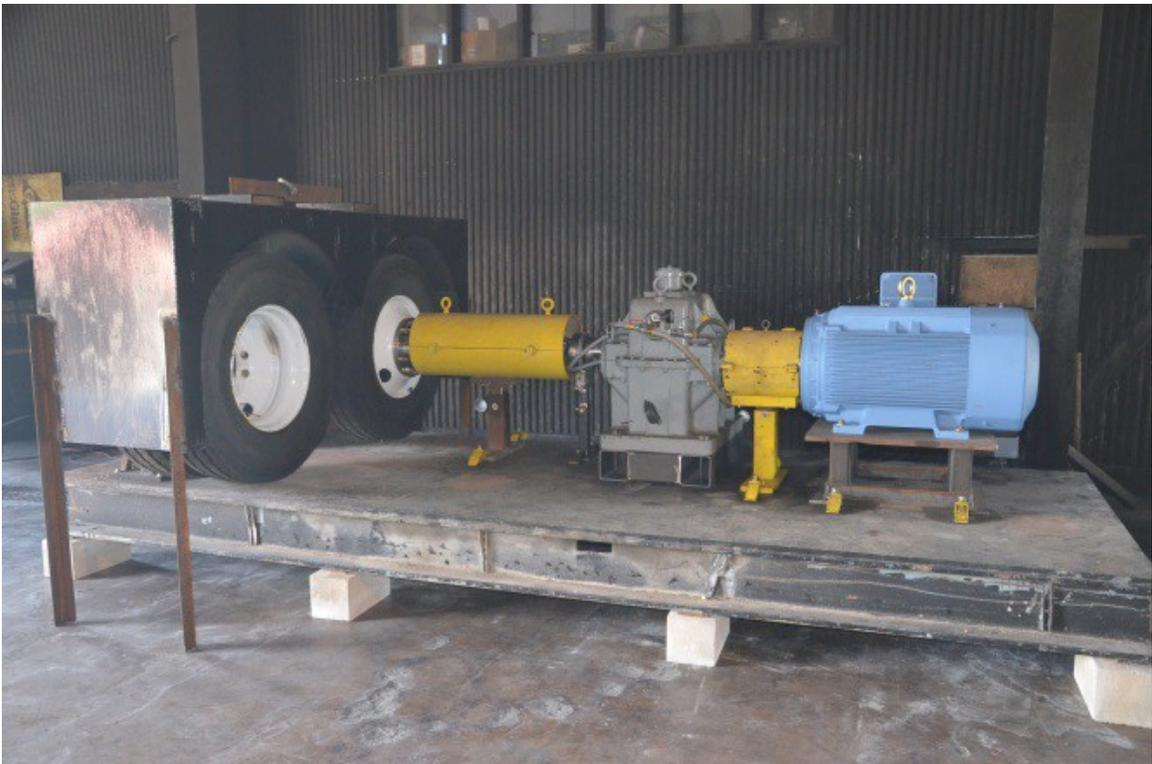
**Figure 3. Wheel Well Mockup Test Fixture (Ground Level View).**
