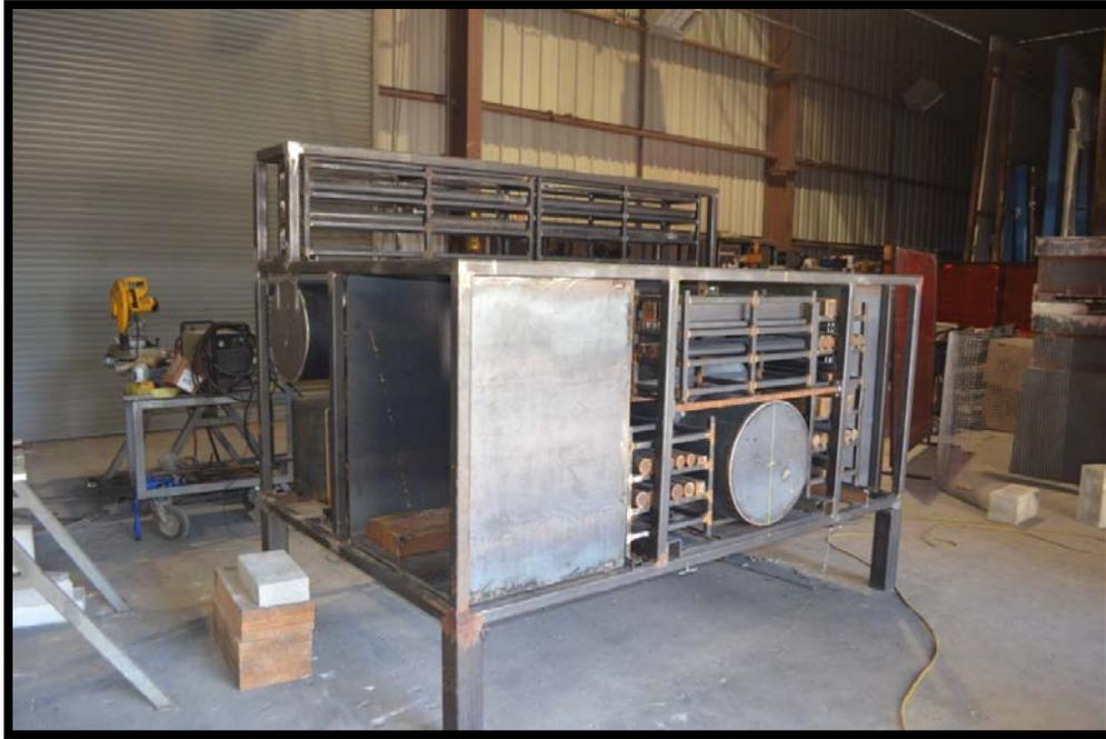
**Figure 17. Engine Compartment Mockup Test Fixture
