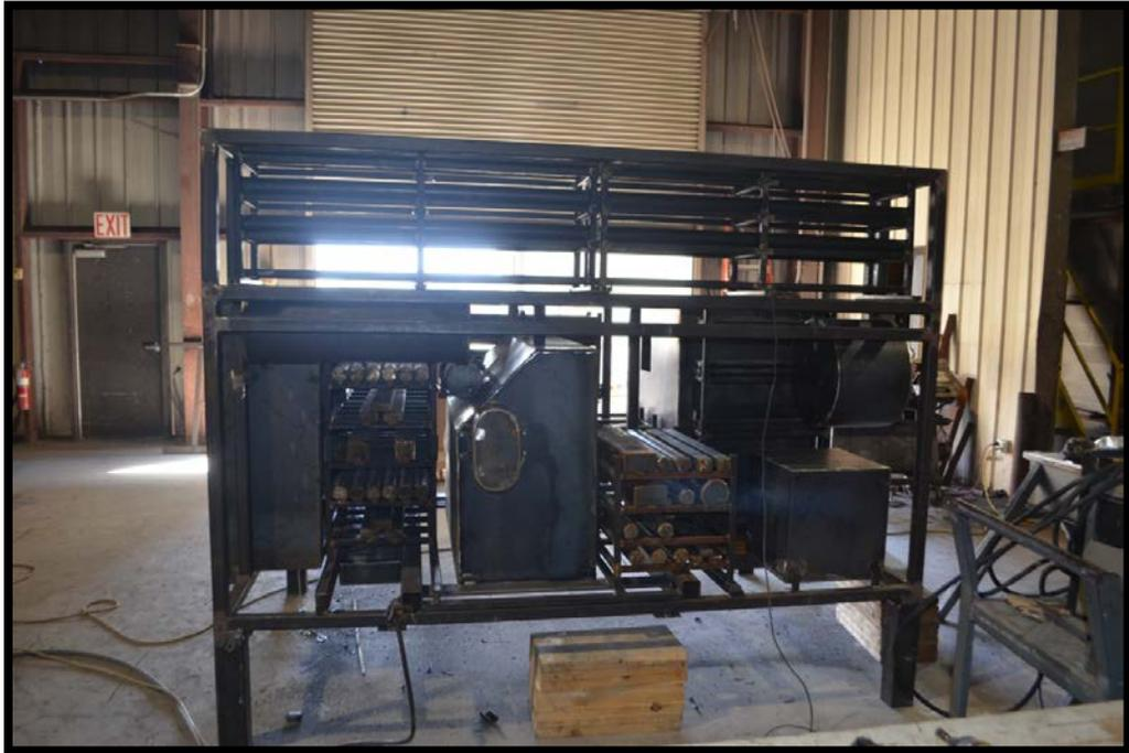
**Figure 20. Engine Compartment Mockup Test Fixture
