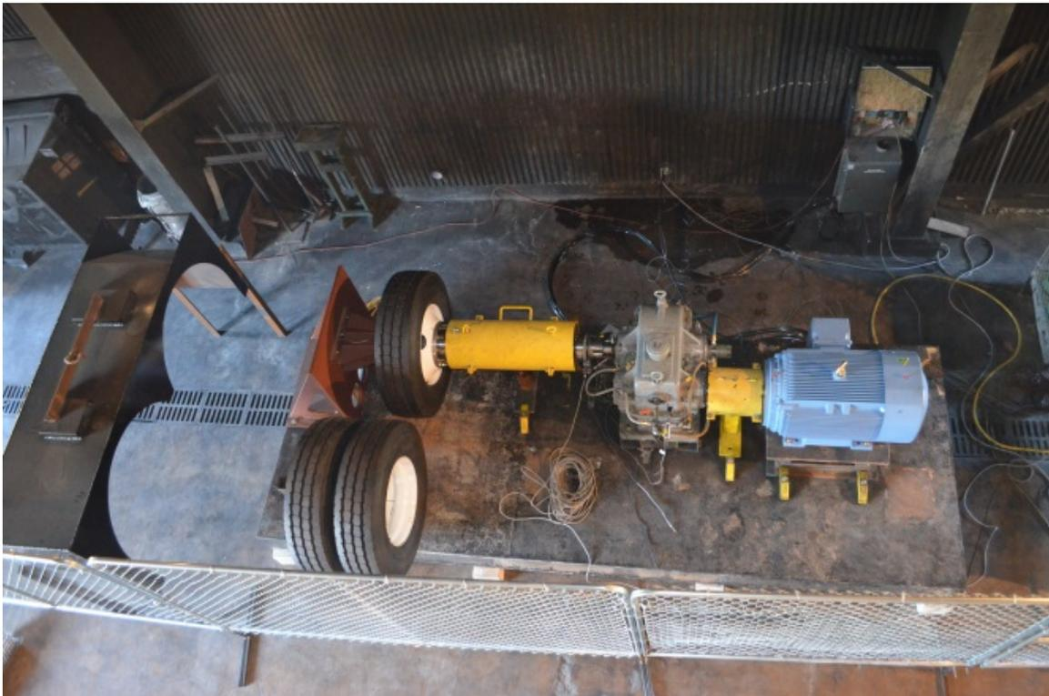
**Figure 38. Wheel Well Mockup Test Fixture (Overall Plan View).**
