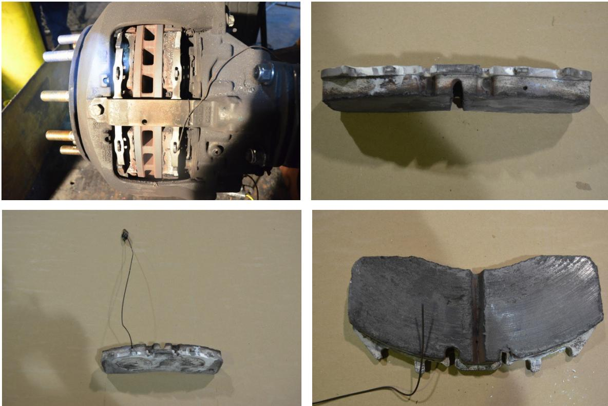
**Figure 4. Brake Pad Thermocouple Location and Construction.**
