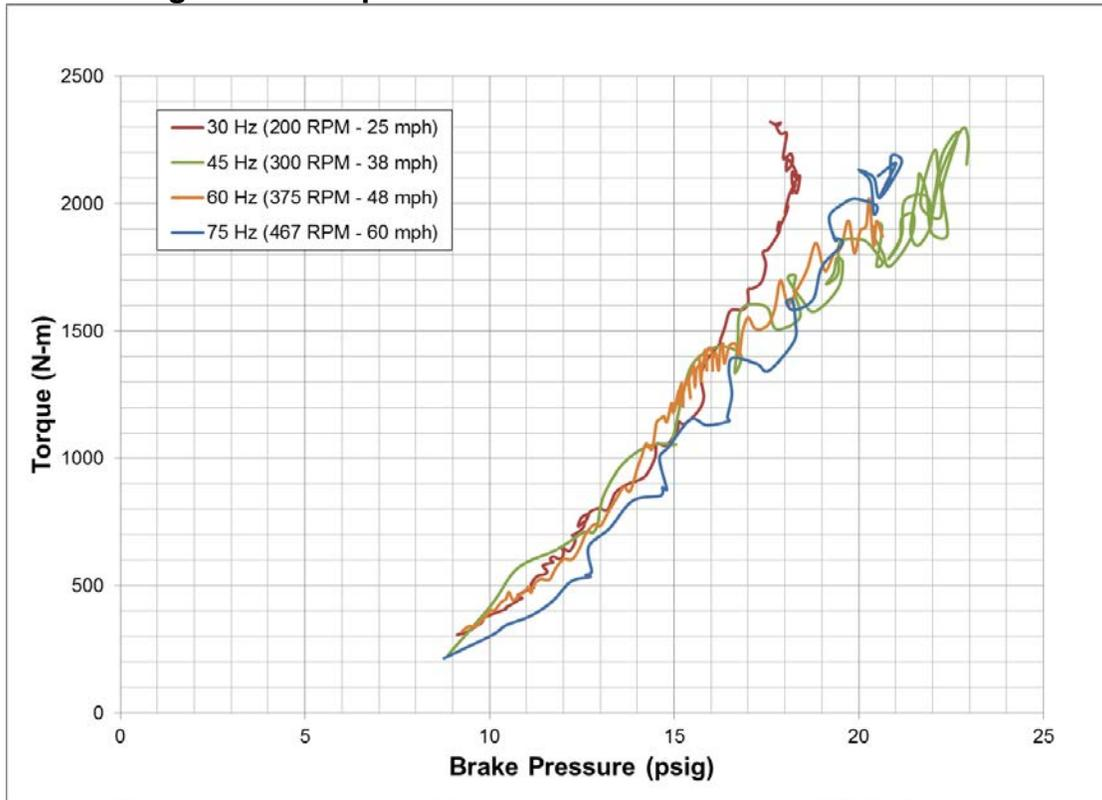
**Figure 45. Torque as a Function of Applied Brake Pressure.**
