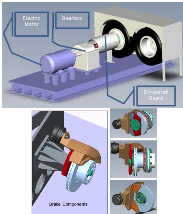
**Figure 37. Motorcoach Wheel Well Test Fixture Final Design.**
