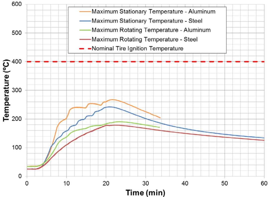
**Figure 57. Comparison of Steel and Aluminum Wheel Temperatures in Short Test.**
