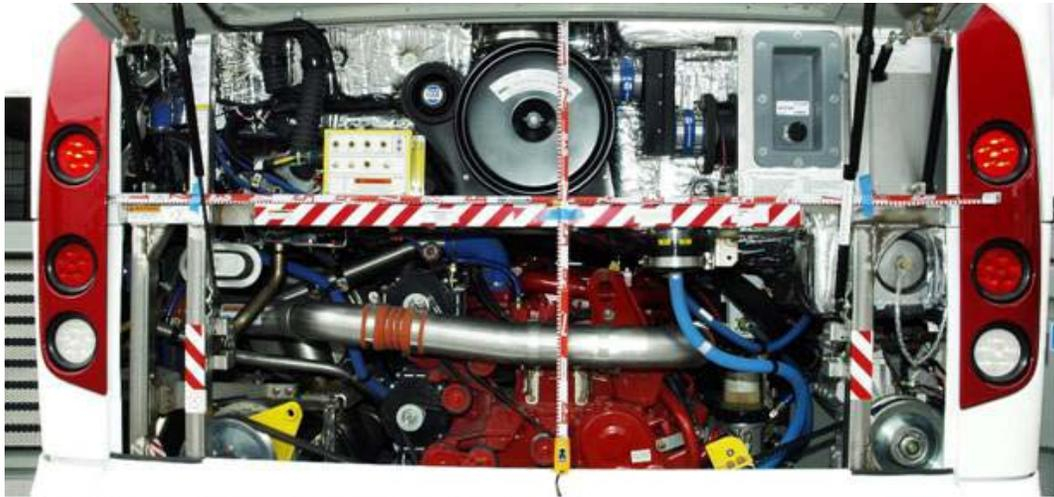
**Figure 5. Photograph of Motorcoach A with Gross Volume of 7.4 m<sup>3</sup>.**
