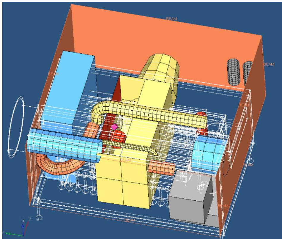
**Figure 9. 3-D Model of Motorcoach B Engine Compartment.**
