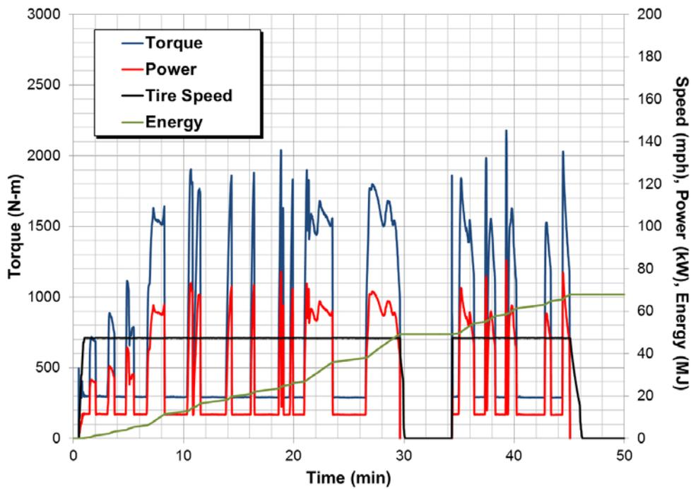
**Figure 48. Heat Input Data from Tire Blowout/Fire Test.**
