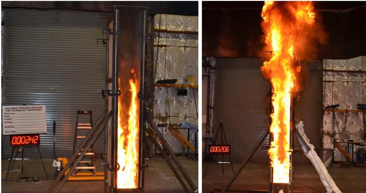
**Figure 73. Parallel Panel Test – Left: Coated GRP, Right: Uncoated GRP.**
