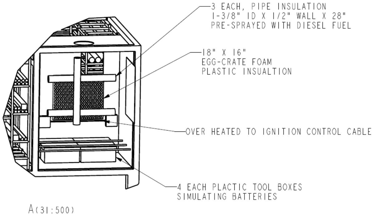
**Figure 13. Battery Compartment Fire Scenario (Close-up View).**
