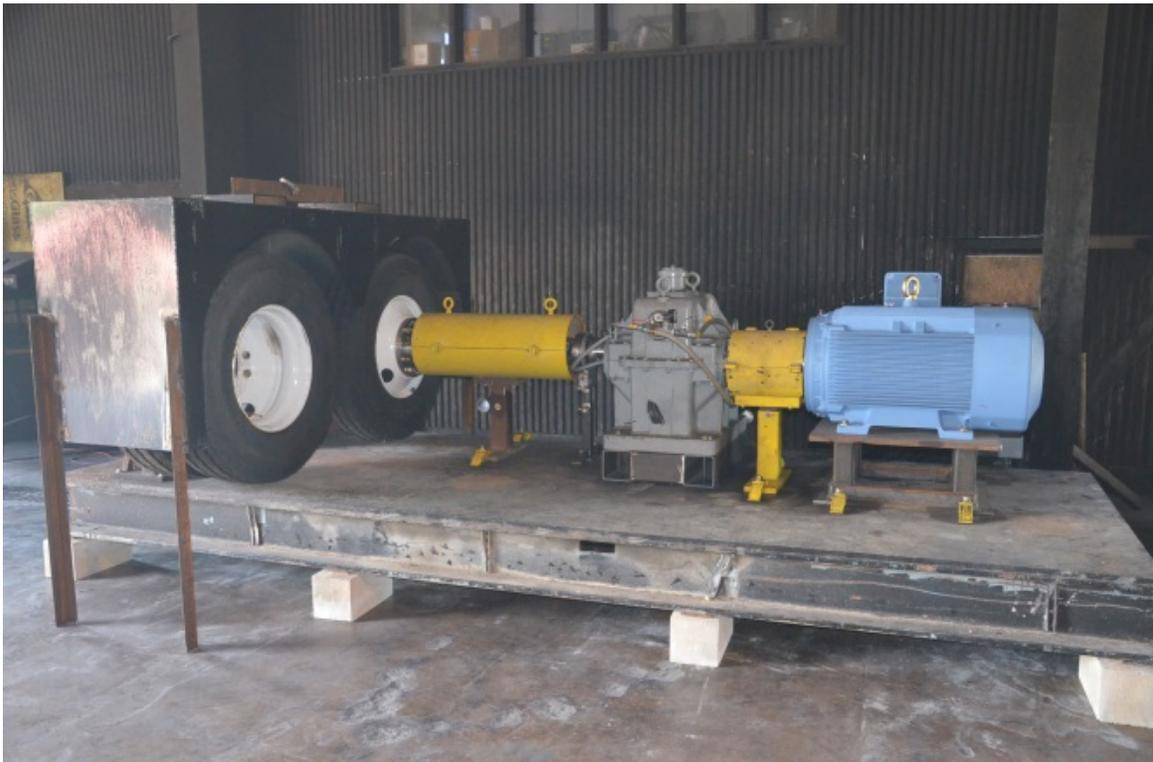
**Figure 39. Wheel Well Mockup Test Fixture (Ground Level View).**
