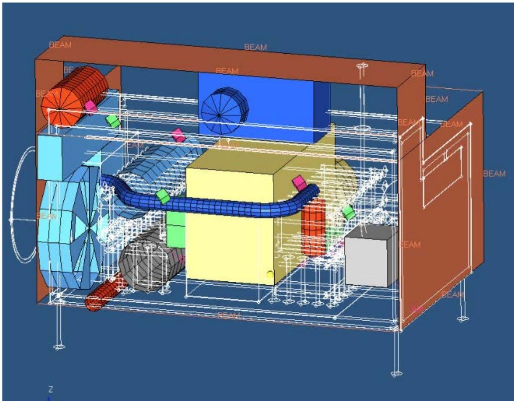
**Figure 8. 3-D Model of Motorcoach A Engine Compartment.**
