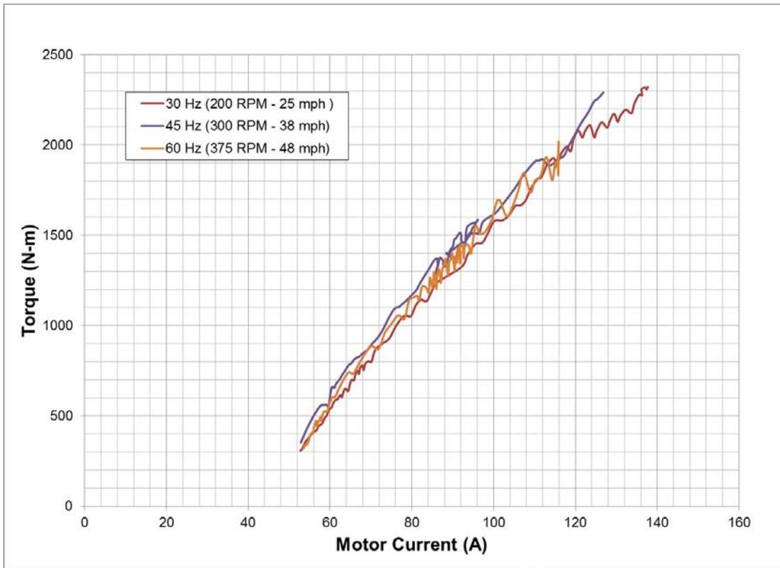
**Figure 44. Torque as a Function of Motor Current Draw.**
