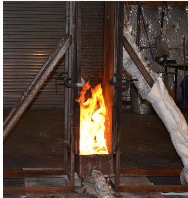
**Figure 72. Parallel Panel Test – Left: Setup, Right: Peak HRR (Uncoated Sheet Metal Material Shown).**
