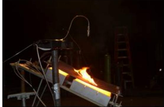
**Figure 31. Hot Surface Ignition Testing.**
