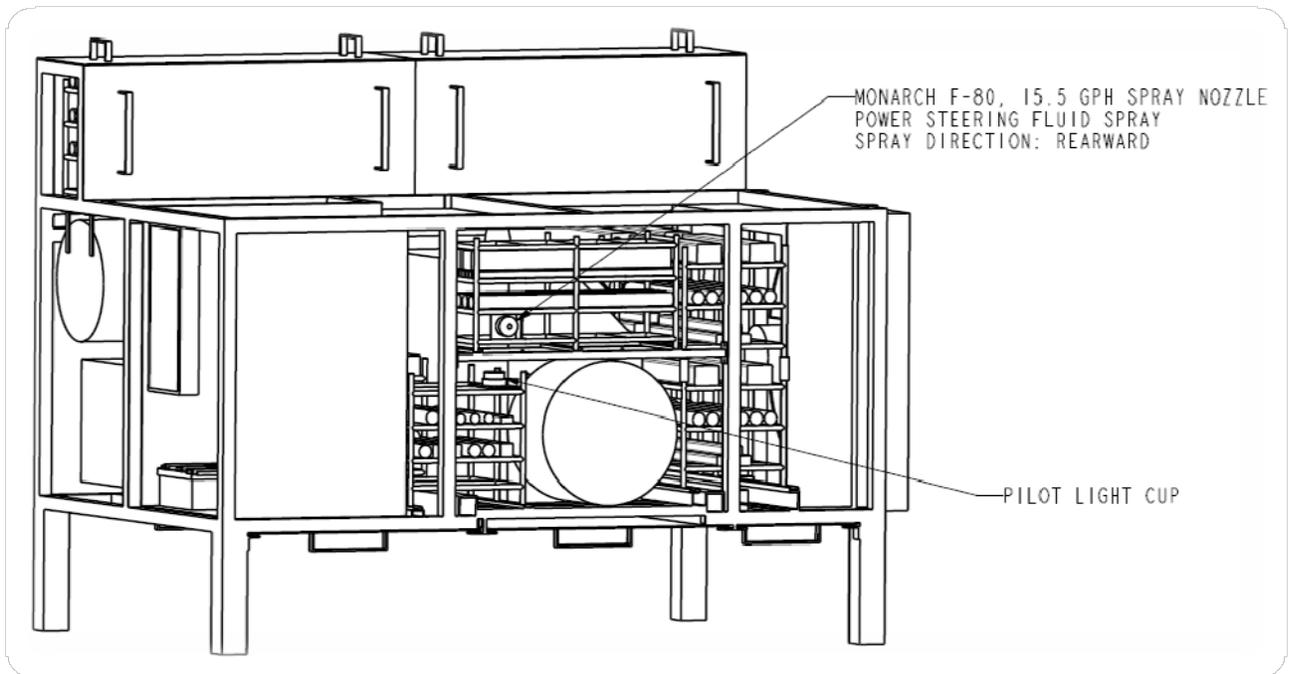
**Figure 7. PSF Spray Fire Scenario (View of Forward Side).**
