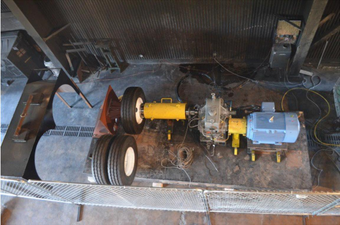
**Figure 2. Wheel Well Mockup Test Fixture (Overall Plan View).**
