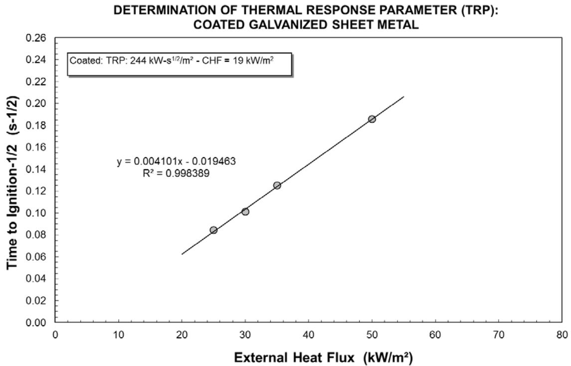
**Figure 68. TRP Plot for Coated Galvanized Sheet Metal.**
