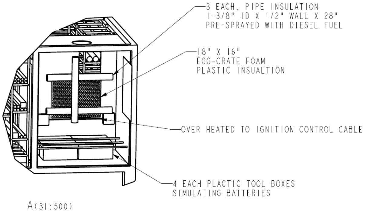
**Figure 30. Battery Compartment Fire Scenario
