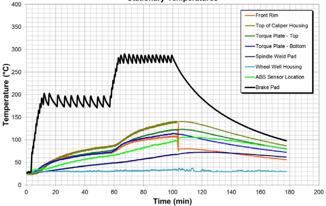
**Figure 54. Abbreviated Burnishing – Stationary Temperatures.**
