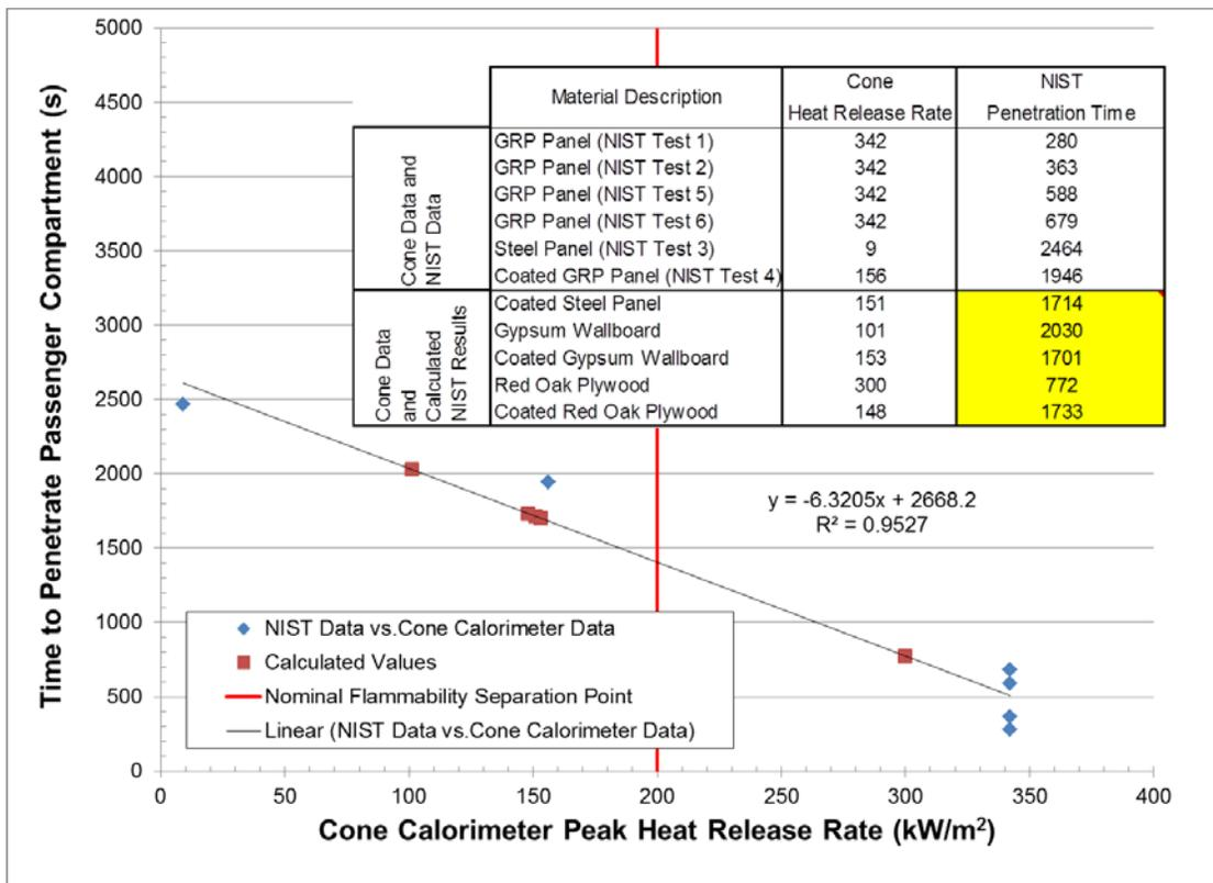
**Figure 77. Cone Calorimeter Peak Heat Release Rate versus NIST Time to Penetration.**
