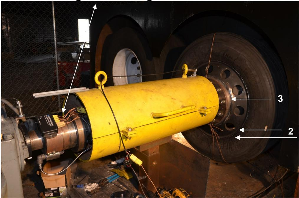
Figure 42. Rotating Temperature Measurement Locations (Front of Rim).
