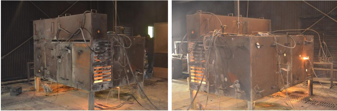
**Figure 35. Photographs of Selected Baseline Tests in Progress: Top Left: PSF Spray Fire, Top Right: Diesel Spray Fire, Bottom Left: Pool Fires (Rear View), Bottom Right: Pool Fires (Forward View).**
