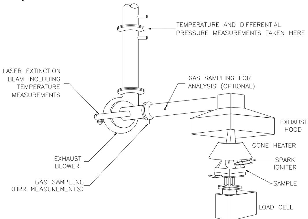
**Figure 65. Schematic of the Cone Calorimeter Apparatus.**
