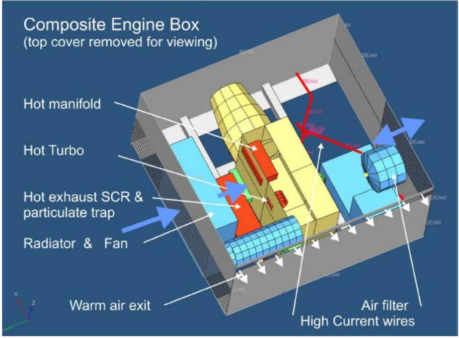
**Figure 11. 3-D Model of Representative Motorcoach Engine Compartment.**
