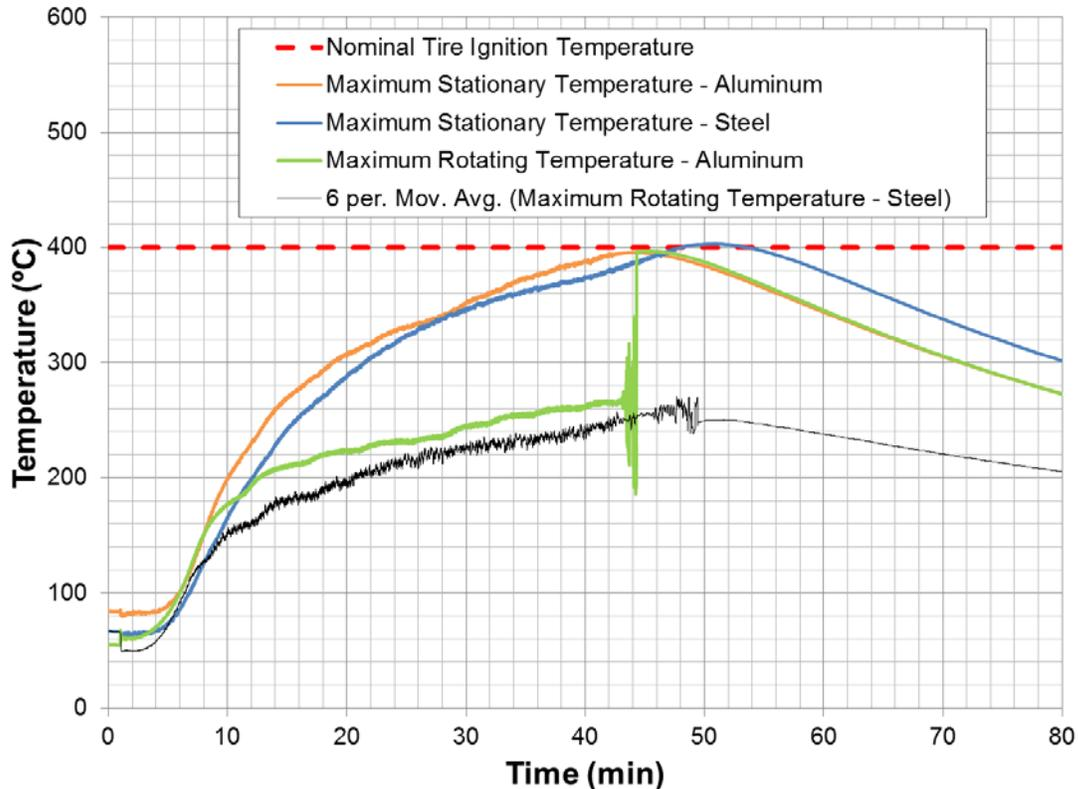
**Figure 58. Comparison of Steel and Aluminum Wheel Temperatures in Long Test.**
