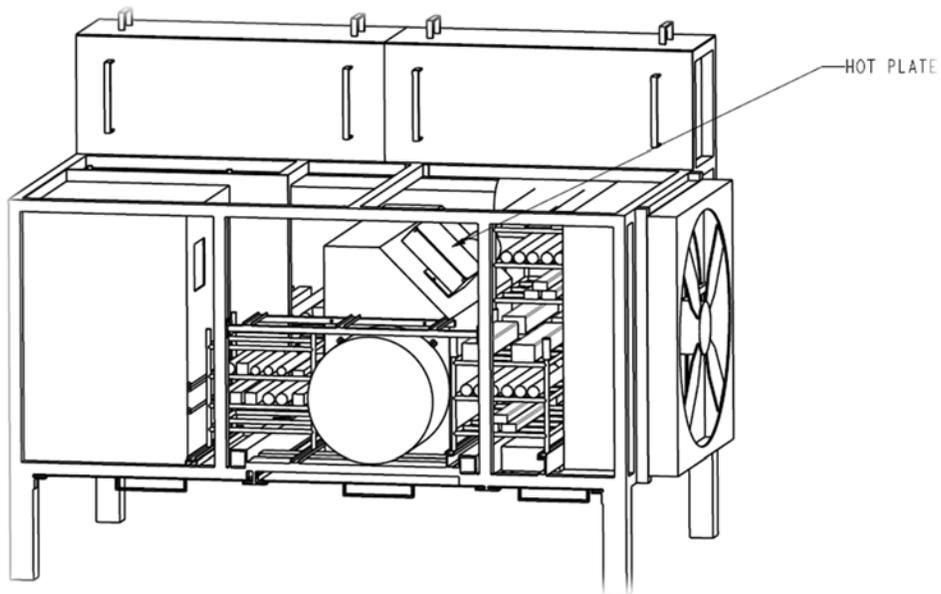
**Figure 21. Hot Surface Re-Ignition Fire Scenario
