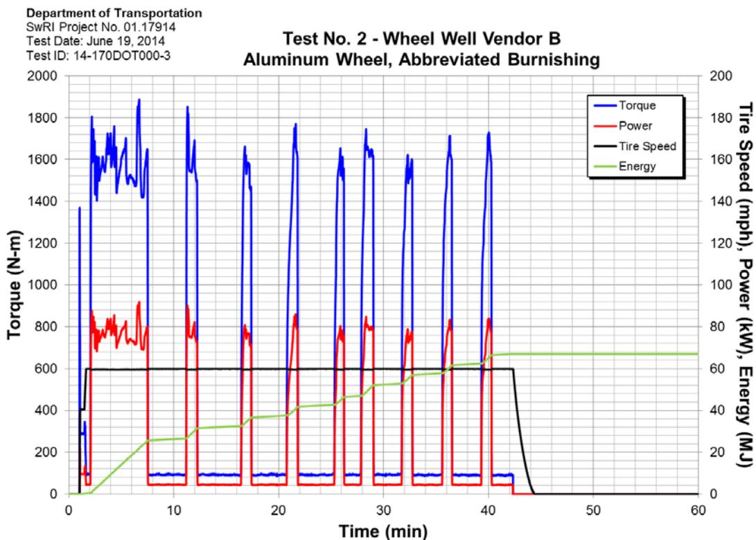
**Figure 55. Vendor B: Test 2 – Abbreviated Burnishing – Heat Input.**
