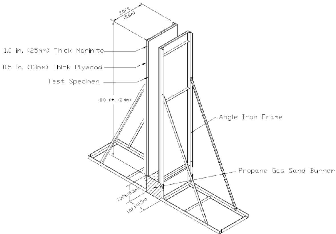
**Figure 66. Schematic of the Parallel Panel Apparatus.**
