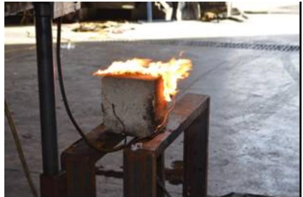
Figure 33. Plastic Fire Ignition Testing (ABS (Black) and PP (White)).
