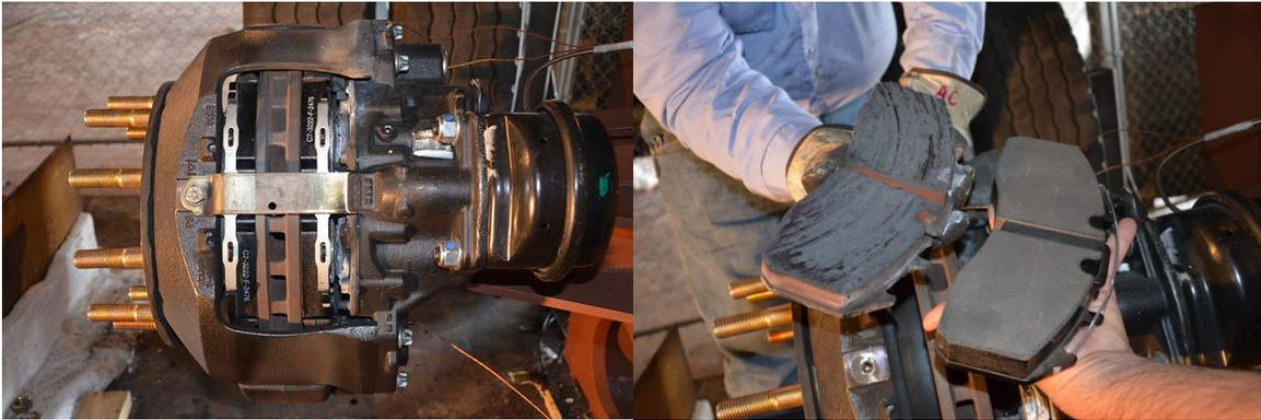
**Figure 46. Left: Brake Pad Installation, Right: Brake Pad Comparison (Left: Glazed, Right: New).**
