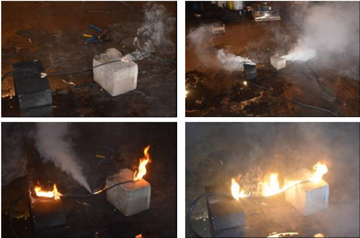
**Figure 34. Overheated Cable Ignition Testing**
