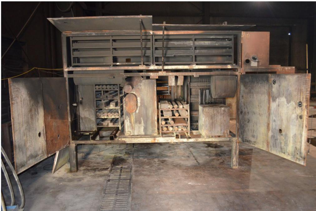
**Figure 2. Engine Compartment Test Fixture (Rear View).**
