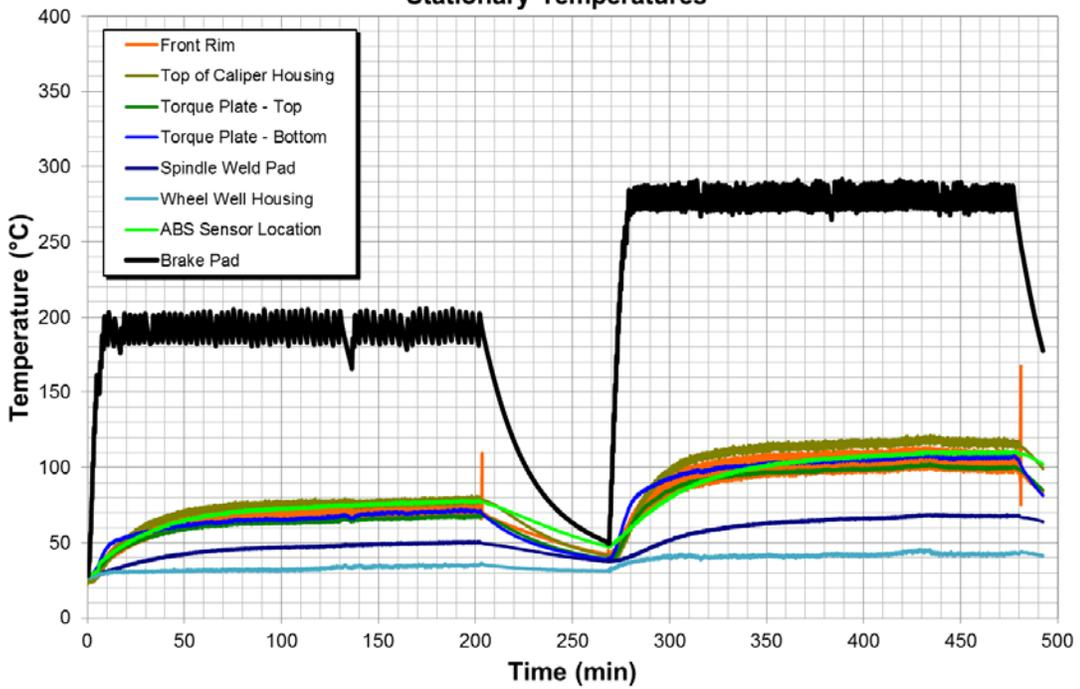
Figure 52. Full Burnishing – Stationary Temperatures.
