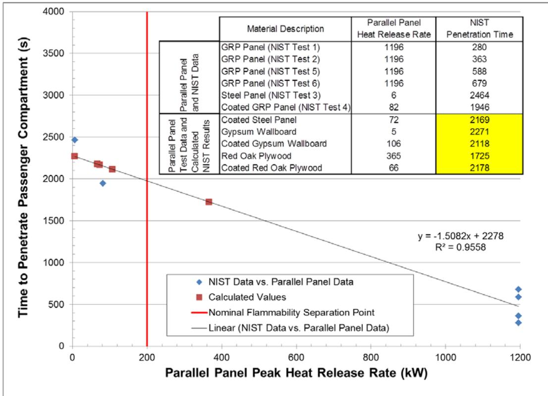
**Figure 76. Parallel Panel Peak Heat Release Rate versus NIST Time to Penetration.**
