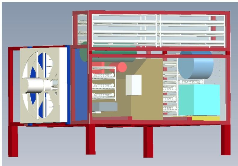
**Figure 12. Engine Compartment Mockup Test Fixture Design (View from Rear Driver's Side Corner).**
