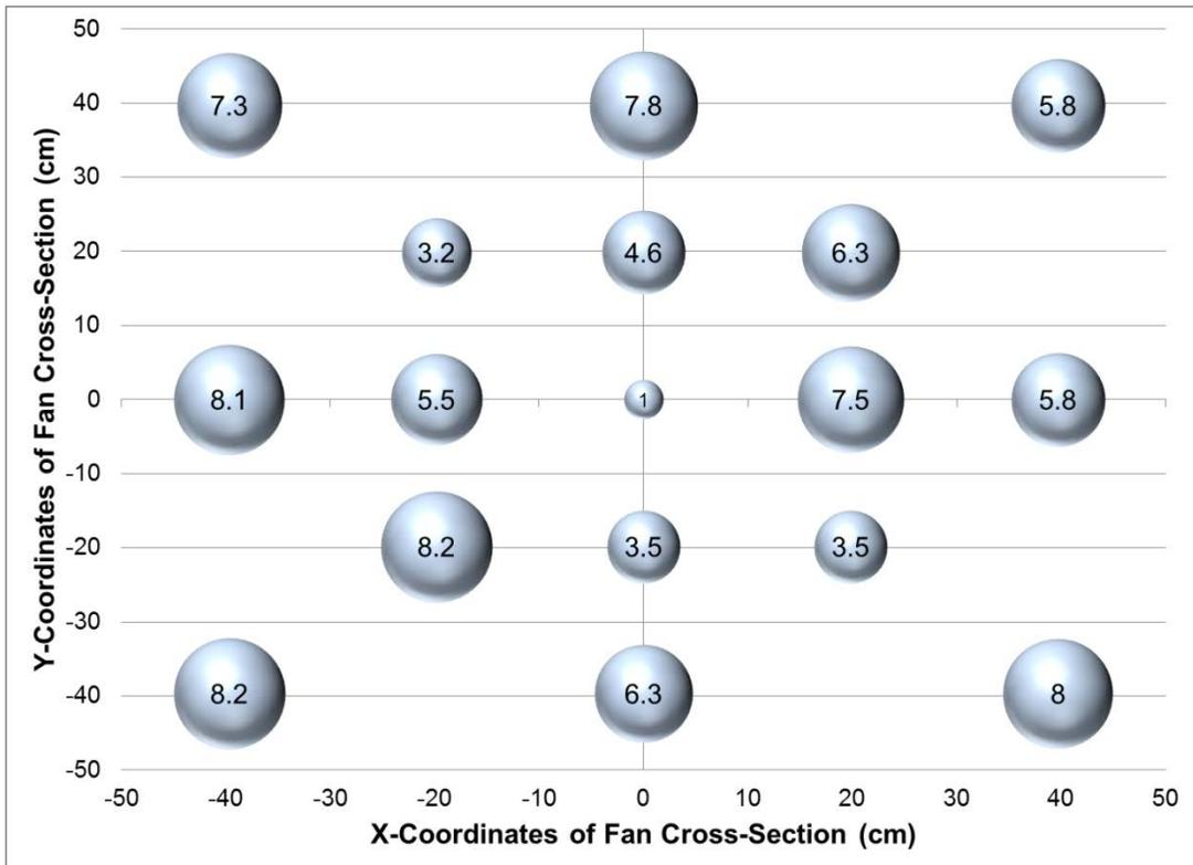
**Figure 15. Engine Compartment Ventilation (Between Louver and Hot Side Clutter).**
