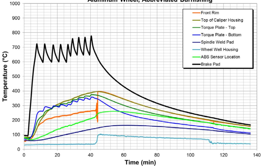
**Figure 56. Vendor B: Test 2 – Abbreviated Burnishing – Stationary Temperatures.**
