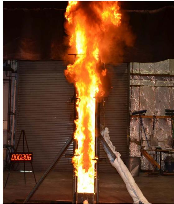
**Figure 71. Parallel Panel Test – Left: Setup, Right: Peak HRR (Uncoated GRP Material Shown).**
