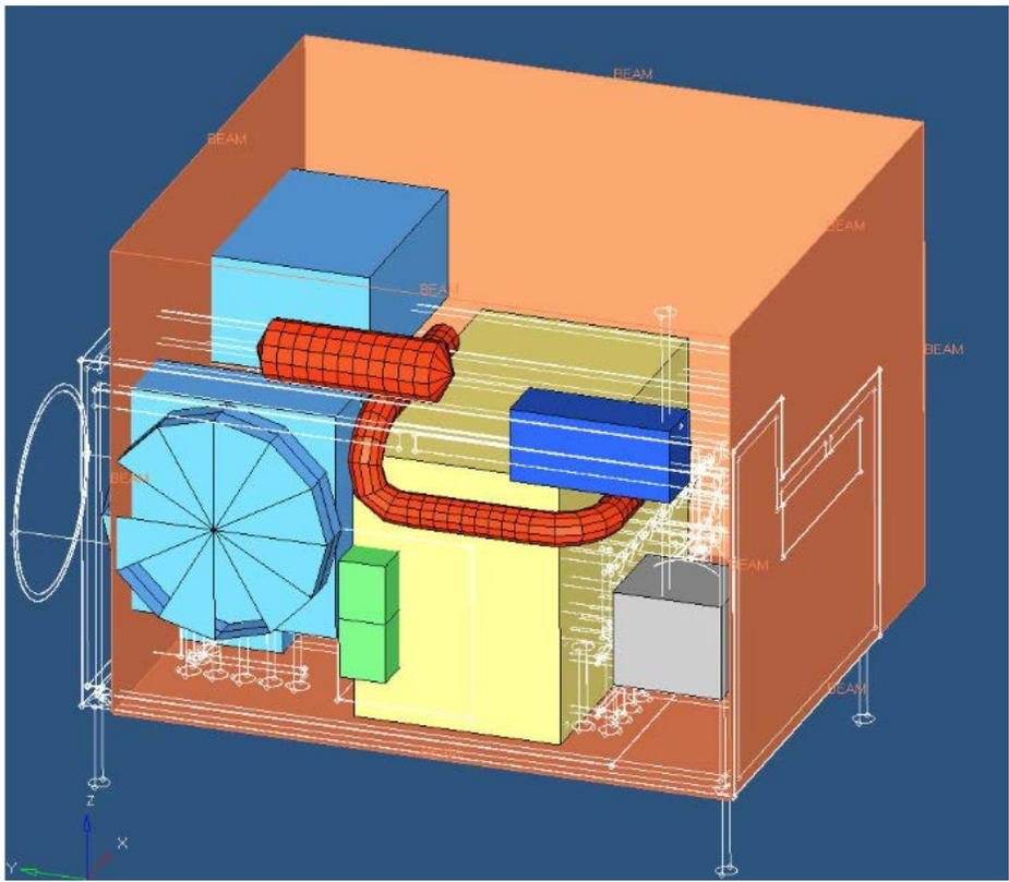
**Figure 10. 3-D Model of Motorcoach C Engine Compartment.**
