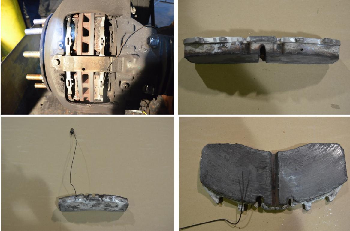
**Figure 50. Brake Pad Thermocouple Location and Construction.**
