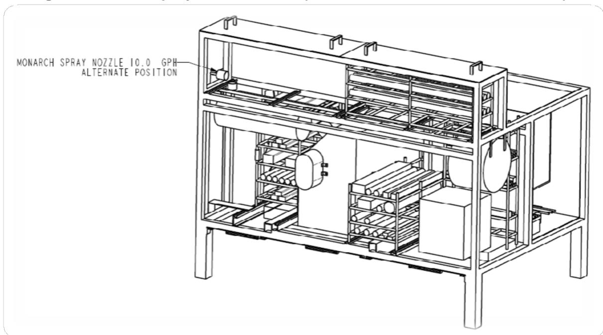
**Figure 6. Diesel Spray Fire Scenario (View of Rear Side: Upper Position).**
