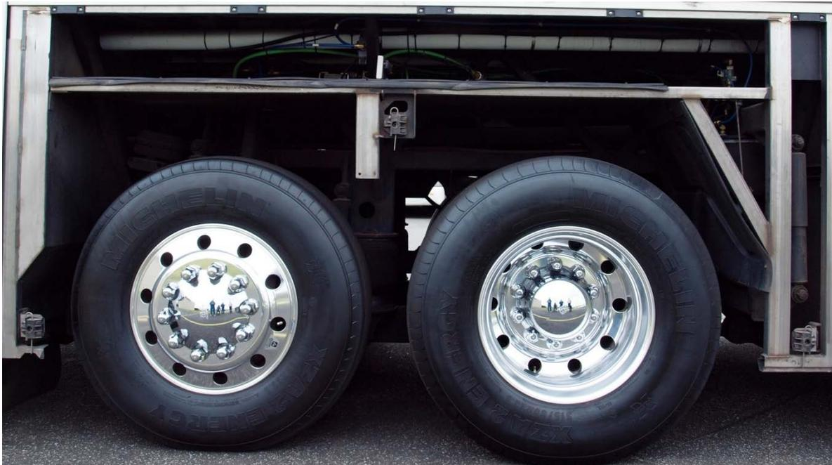
**Figure 3. Photograph of Motorcoach B Wheel Well (without fender side panel).**
