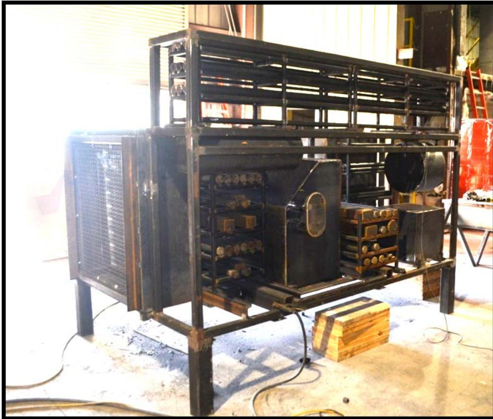
**Figure 16. Engine Compartment Mockup Test Fixture (View of Rear Driver Side – Prior to Installation of Fan).**
