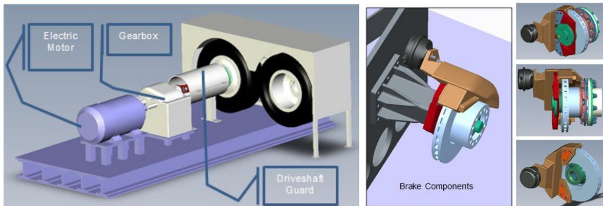
**Figure 1. Motorcoach Wheel Well Test Fixture Final Design.**
