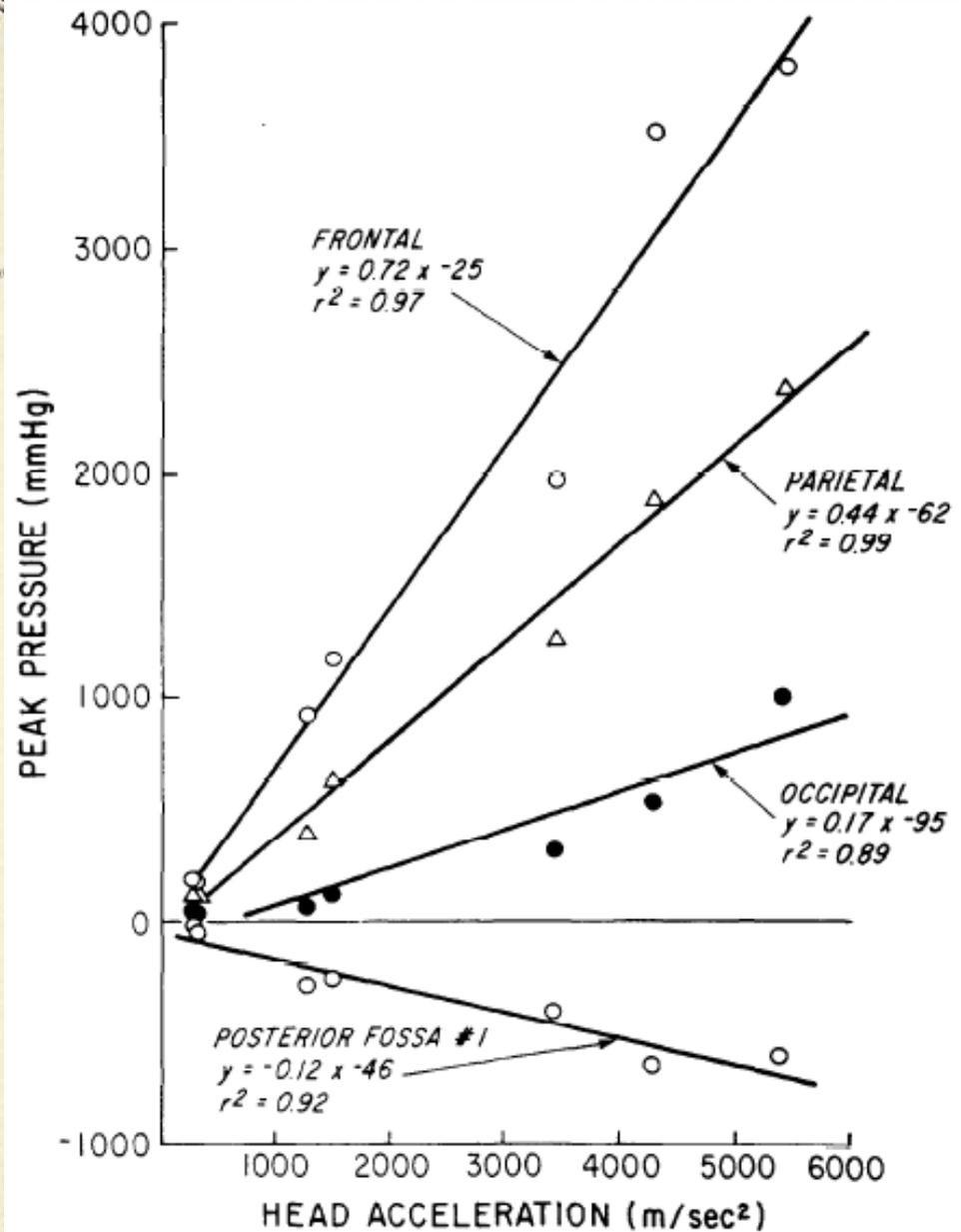
Fig. 7 - Regression analysis of peak pressure-head acceleration relationship
