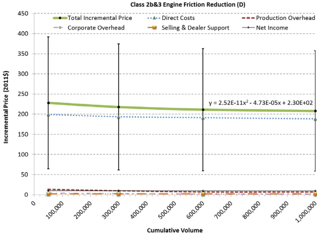
**Class 2b&3 Engine Friction Reduction (D)**
