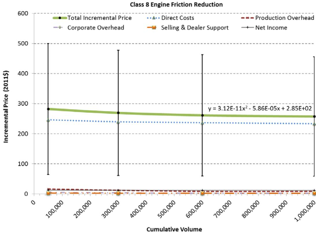
**Class 8 Engine Friction Reduction**
