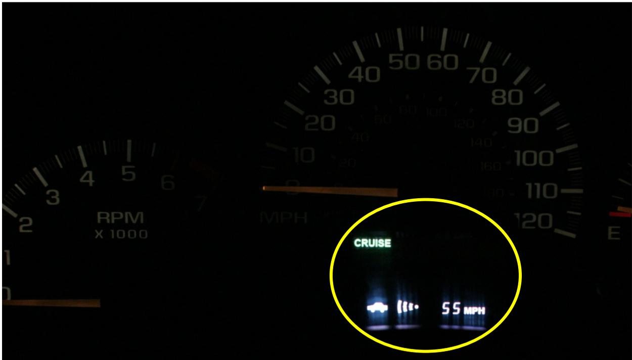
Figure 2: ACC Display in NADS-1.
