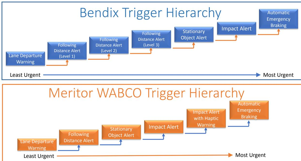
**Figure 6. Hierarchy of Activations for Bendix and Meritor WABCO**
