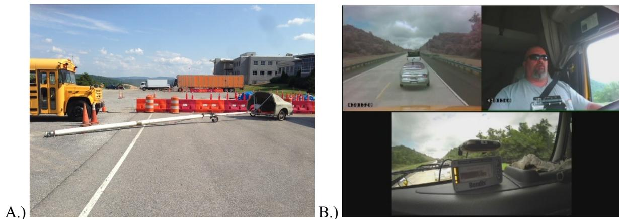
**Figure 4. (A) Crash Shell With Telescoping Boom (B) Triggering Activations With Truck Following Crash Shell**
