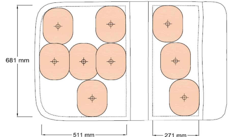
Some rear panel targets eliminated per FMVSS No. 226 procedure
