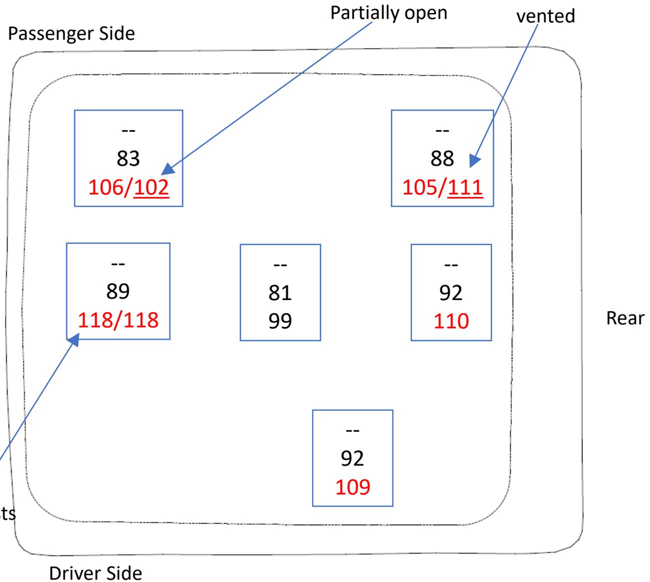
Only difference between production and countermeasure panels are holes in PET film
