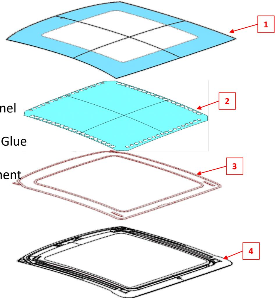
frit = a black enamel band that is baked into the edges of the windshield for better adhesive bond and protect bond from UV
