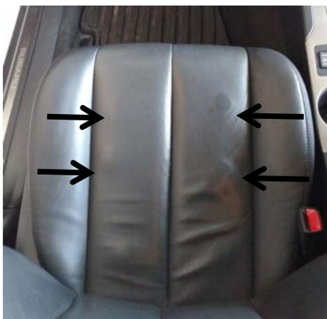
**Figure 21. Experiment vehicle driver's seat viewed from above (tactor locations indicated by arrows)**
