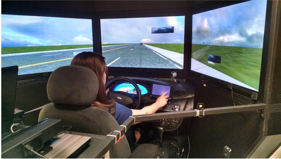
**Figure 6. Motion-base advanced driving simulator**
