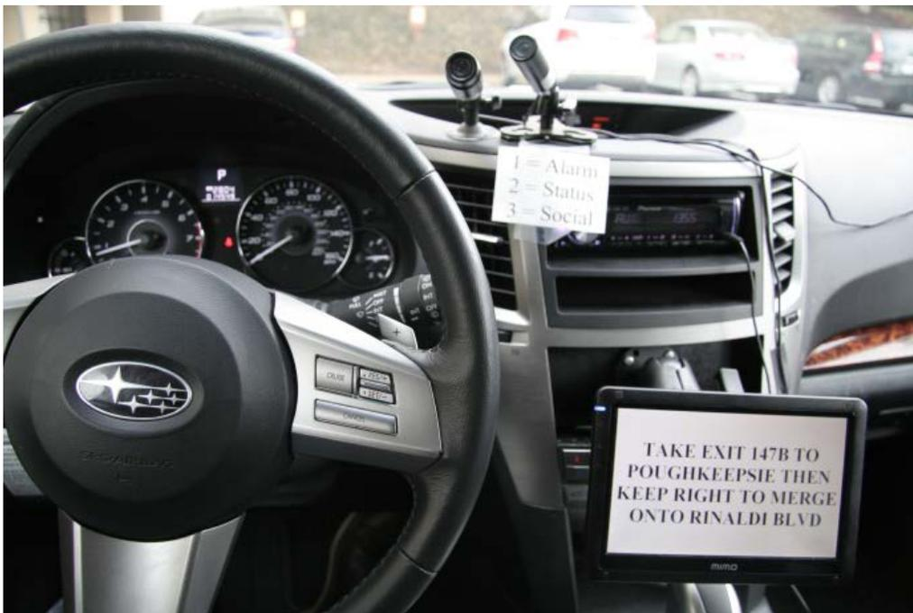
**Figure 22. Display screen with text message**
