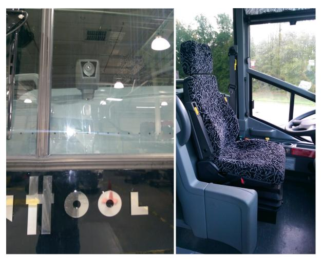
Figure 2.5 Left: Bendix AutoVue LDW System Video Camera Sensor Right: Haptic Feedback Equipped Driver's Seat
