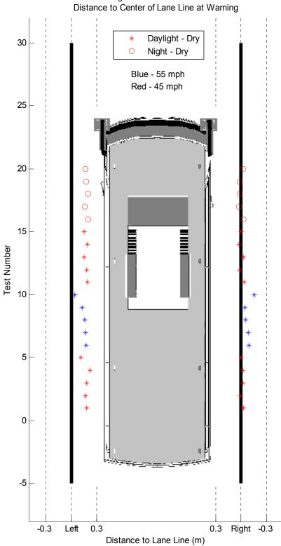
Straight Lane Solid Lane Line Distance to Center of Lane Line at Warning
