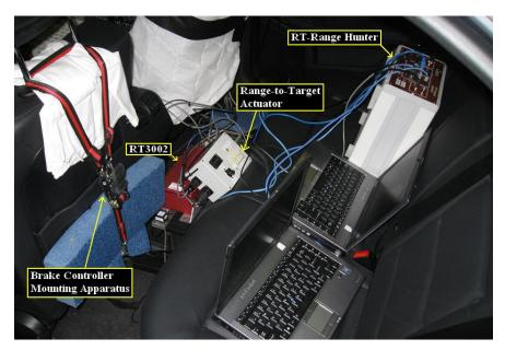
Figure B.1 RT Test Equipment in Rear Seat of Vehicle
