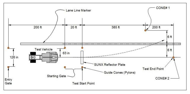
Figure 2.1 Heavy Vehicle LDW Left Lane-Change Test Procedure and Layout
