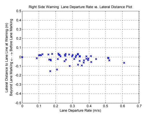
Figure 3.6 Right-Side Test – Lateral Distance to Lane Line at Warning Versus Lane Departure Rate Plot
