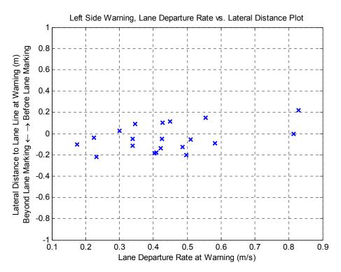
Figure 3.11 Curved Lane, Left-Side Test – Lateral Distance to Lane Line at Warning Versus Lane Departure Rate Plot
