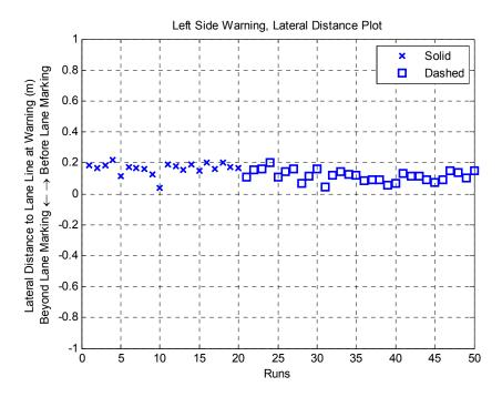
Figure C.1 Straight Lane, Left-Side Test - Lateral Distance to Lane Line at LDW Distribution
