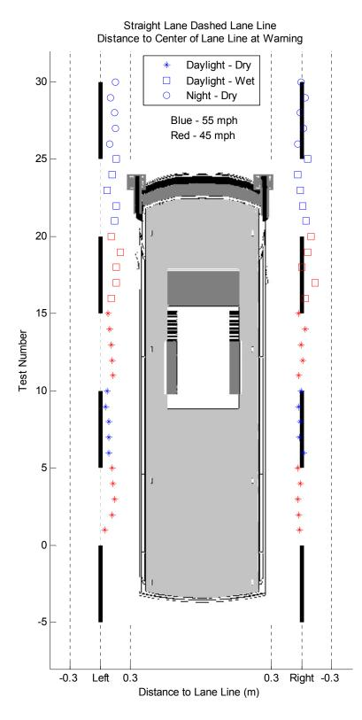
Figure 3.2 Straight Lane Dashed Lane Line – Lateral Distance to Lane Line Distribution at LDW
