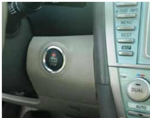
**Figure 19 - Pushbutton Ignition Option in 2007 Toyota Camry**
