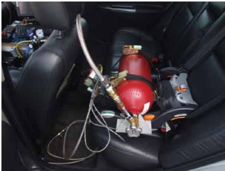
**Figure 4 - Nitrogen Supply Tank and Solenoid Valves Used for Pneumatic Brake Ram Actuation**
