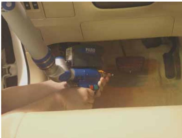
**Figure 8 - FARO Laser Scan Arm Operating in Vehicle**
