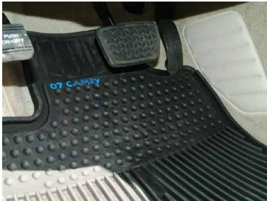
**Figure 34 – Pedal Entrapment with Incorrectly Installed Mat**
