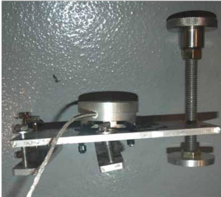
**Figure 9 - Critical Vertical Offset Device with Brake Pedal Force Load Cell Attached**
