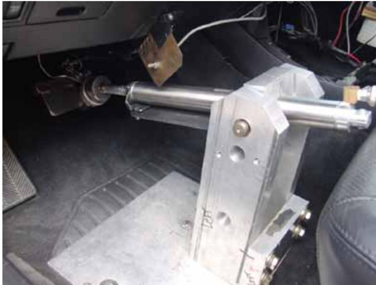
**Figure 3 - Pneumatic Brake Ram Used in Testing**
