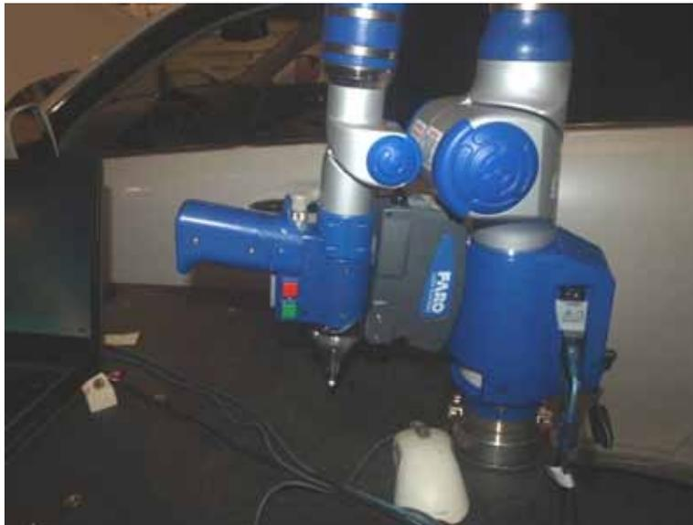
**Figure 7 - FARO Laser Scan Arm - Close-up**
