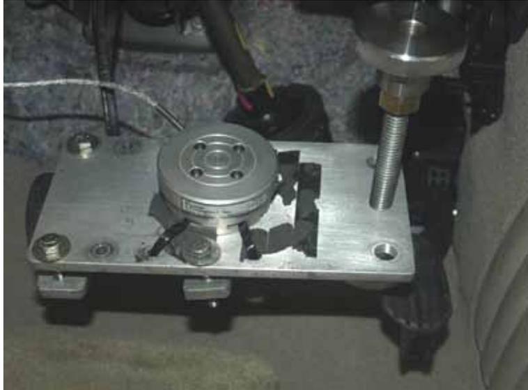
**Figure 10 - Critical Vertical Offset Device Clamped on Brake Pedal with Offset Device Contacting Accelerator Pedal - Close-up**
