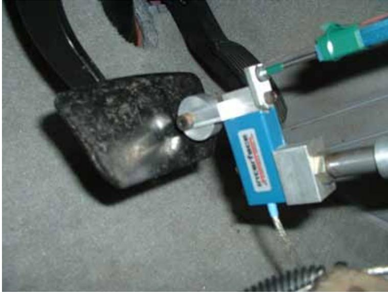
**Figure 6 - Setup of Brake Pedal Force versus Displacement Device in a Typical Test Vehicle - Close-up**
