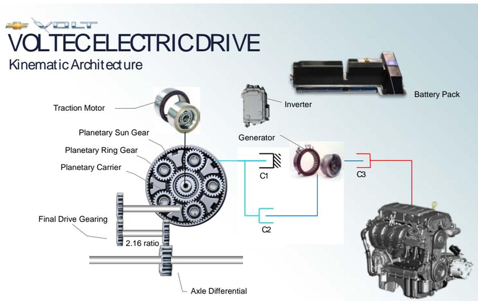
**Figure 22 – Voltec Hybrid Electric Vehicle [source: [www.gm.com](http://www.gm.com)]**
