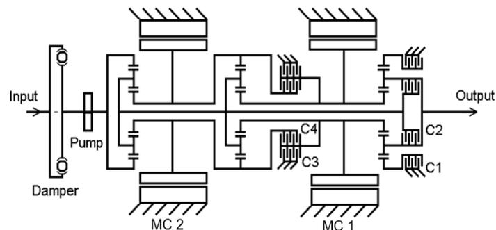
**Figure 21 – Two Mode Transmission with Four Fixed Gears**
