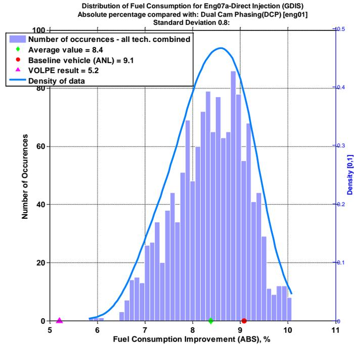
Figure 69 – Example of QA/QC distribution plot
