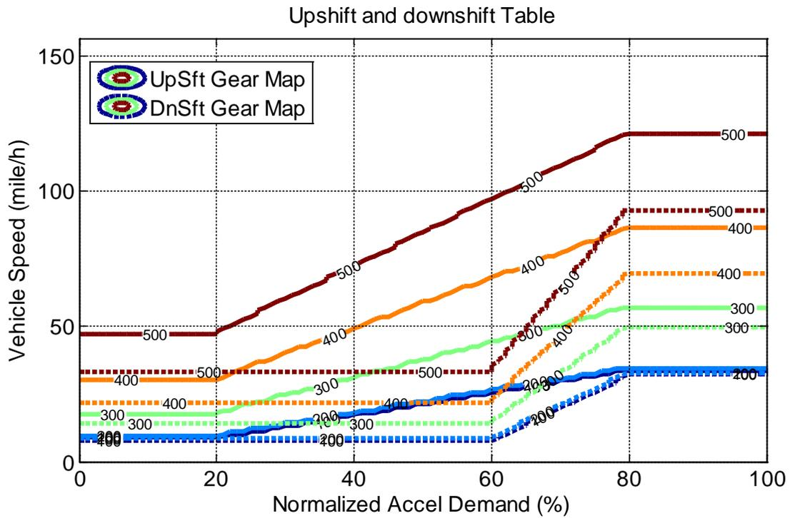
Figure 32 – 5-speed automatic up (plain lines) and down (dotted lines) shifting map
