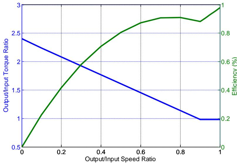
**Figure 35 – Torque Converter efficiency**
