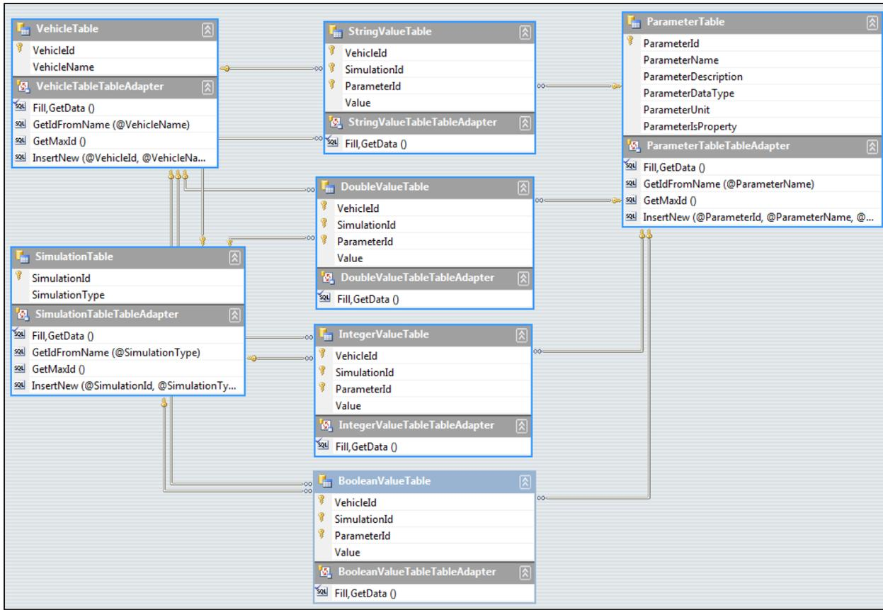
Figure 67 – Database Structure
