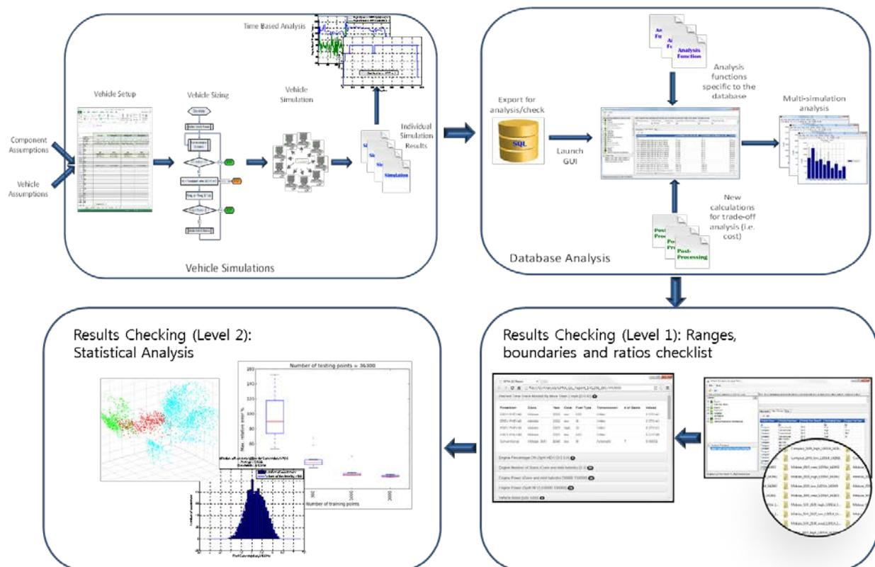
Figure 70 – Large Scale Simulation Process Summary
