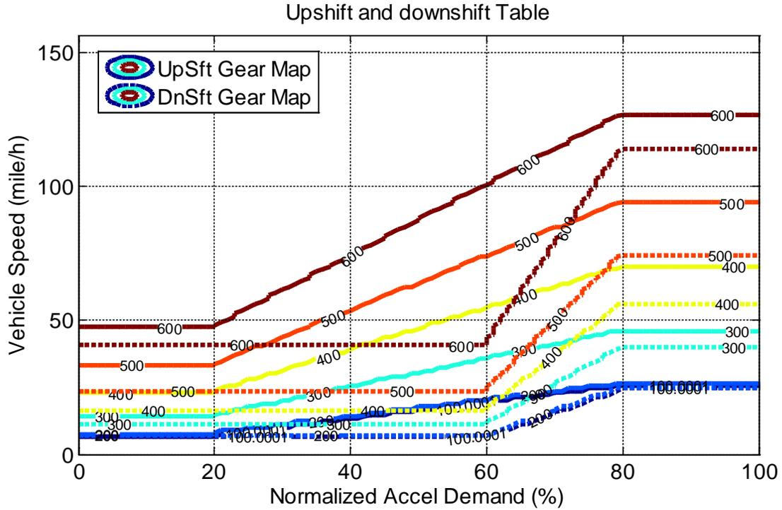
Figure 33 – 6-speed automatic up (plain lines) and down (dotted lines) shifting map
