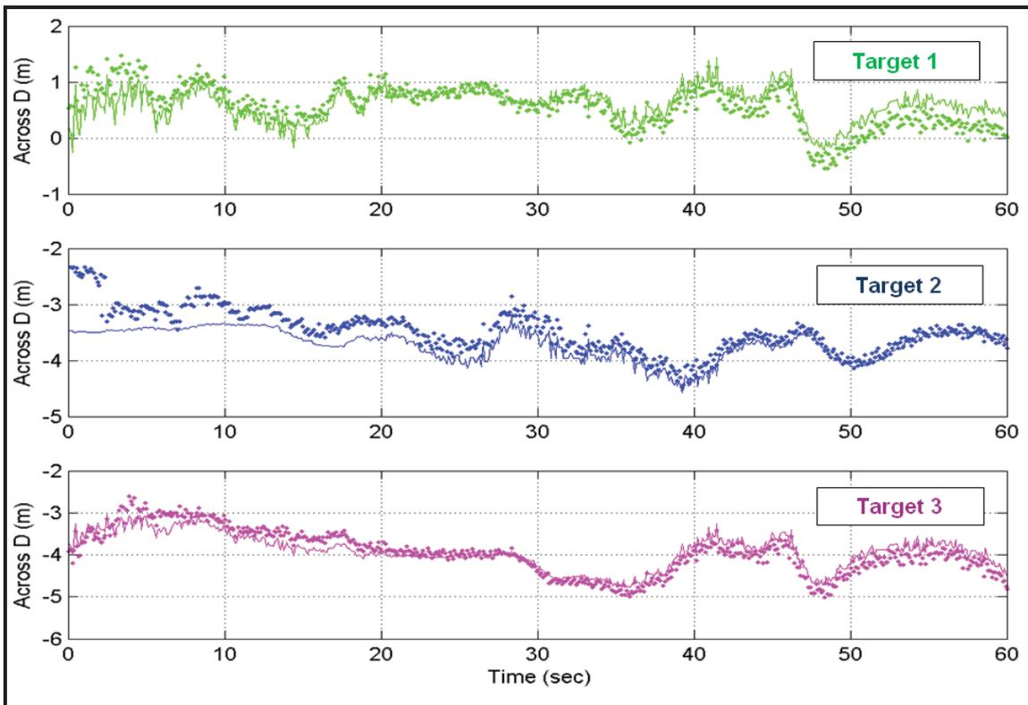
**Figure 21: Between-Vehicle across Distances in Multiple Vehicle Test Run (Solid Line: RTK Method Other: Single Point Method)**
