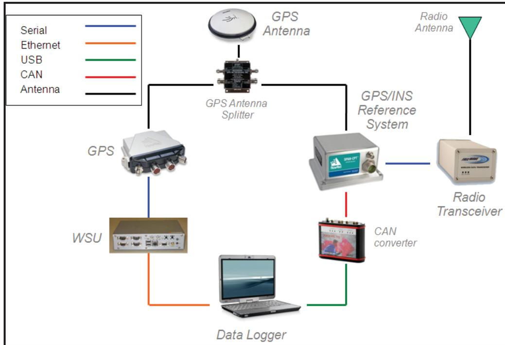
**Figure 23: Reference Positioning System Analysis Equipment Set-up**
