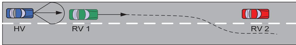
**Figure 3: Cut-out of Lead Vehicle Reveals Stopped Vehicle In-lane**
