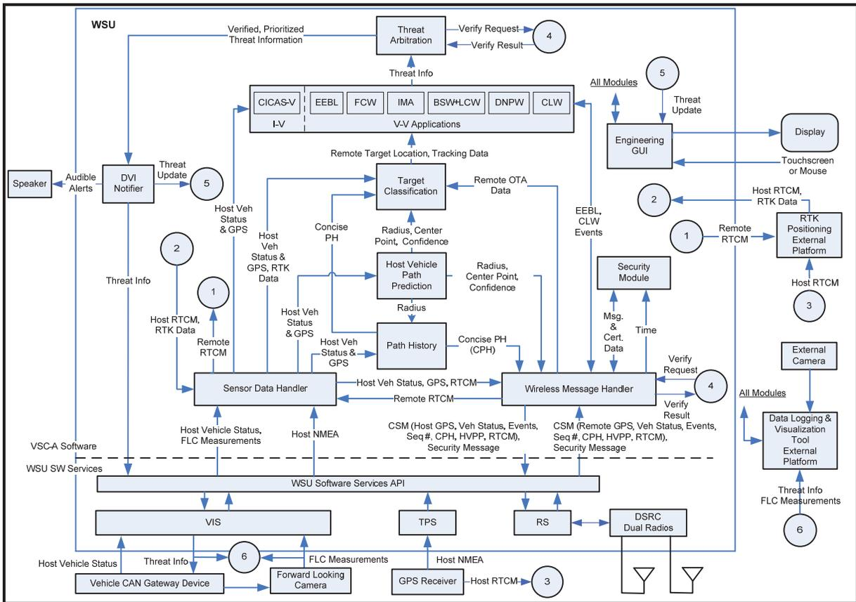
**Figure 6: VSC-A Level I OBE SW Architecture**
