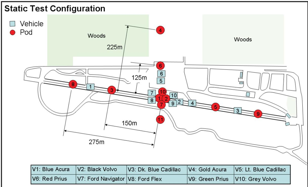
**Figure 32: Vehicle and Pod Static Deployment Configuration**
