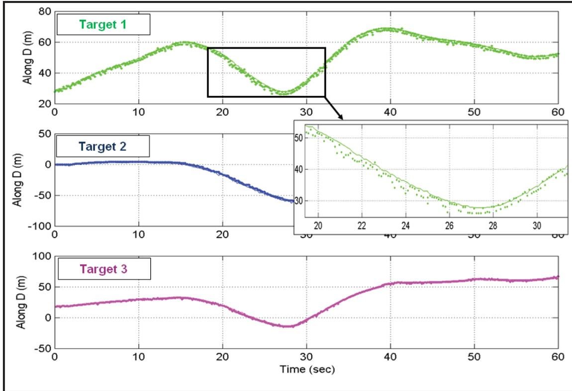
**Figure 22: Between-Vehicle along Distances in Multiple Vehicle Test Run (Solid Line: RTK Method Other: Single Point Method)**
