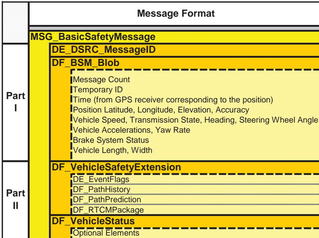
**Figure 15: SAE J2735 Rev 35 Basic Safety Message Format**
