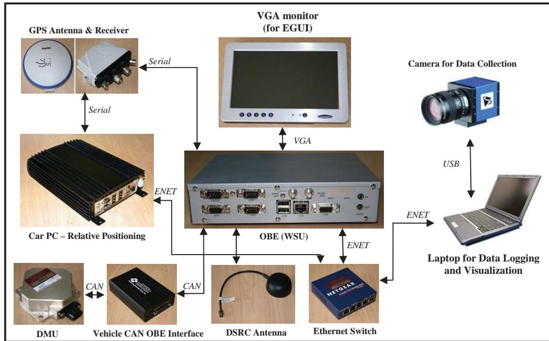
Figure 12: VSC-A System Test Bed HW Layout
