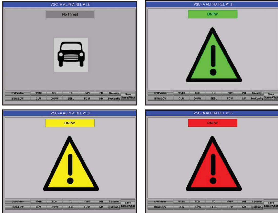
**Figure 9: DVIN Stages: (left → right, top → bottom) No Threat, Threat Detected, Inform Driver, Warn Driver**
