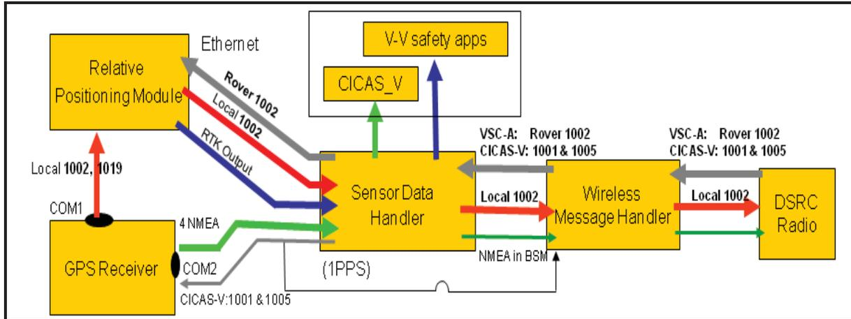
**Figure 18: VSC-A Test Bed Relative Positioning System Core Modules**
