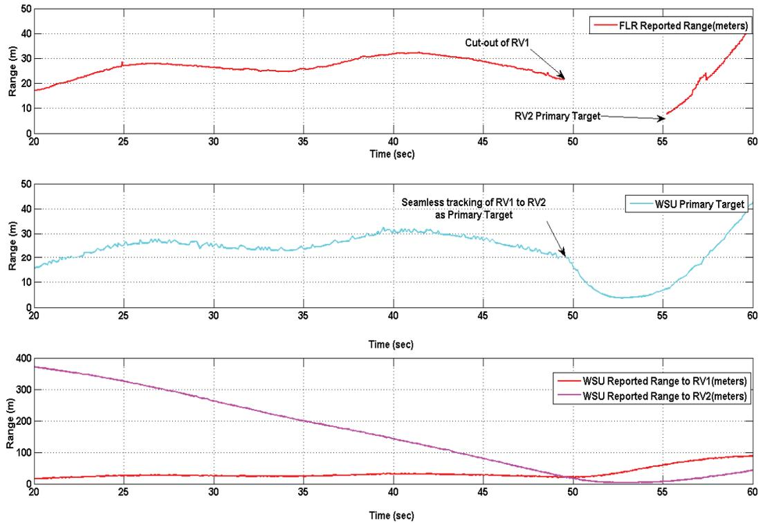
**Figure 4: Sensor Performance during Vehicle Cut-Outs**
