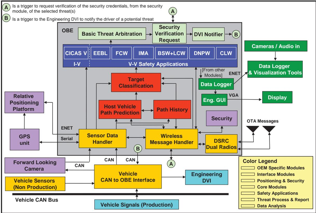
**Figure 5: VSC-A System Block Diagram**
