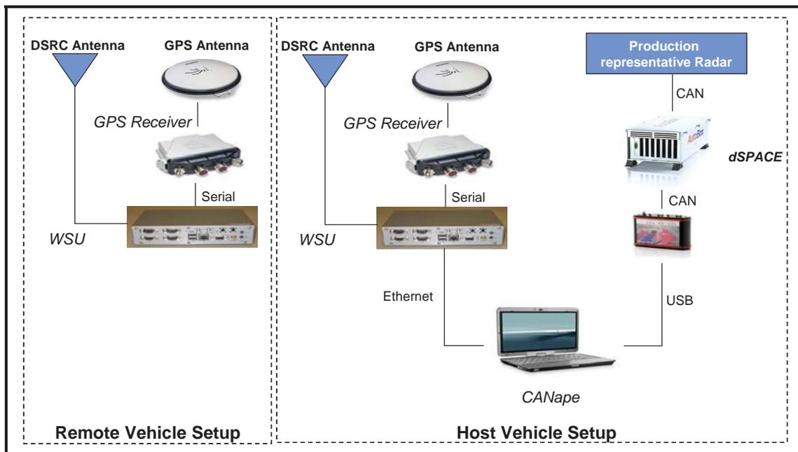
Figure 1: DSRC and Autonomous Sensing Safety System Analysis Setup
