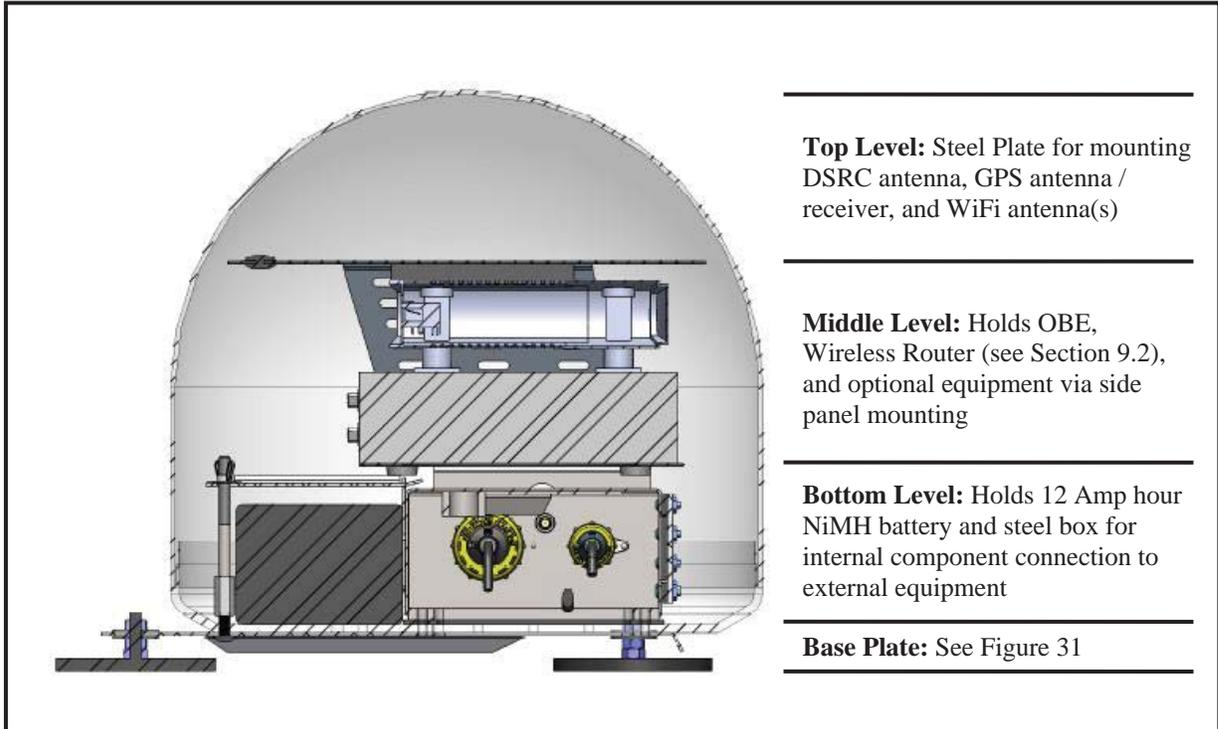
Figure 30: DSRC Pod Internal Structure Diagram
