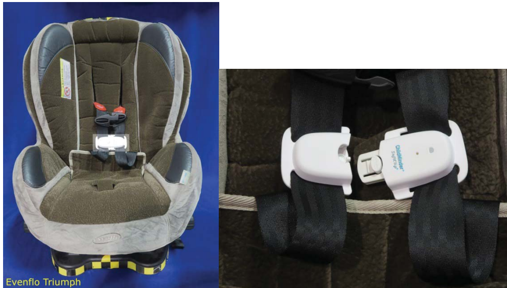
Figure 6: ChildMinder SoftClip installed on harness straps of an Evenflo Triumph convertible CRS. Note that the OEM chest clip was not removed for this assessment.
