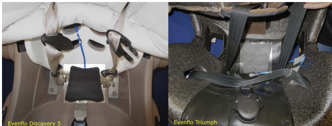
Figure 5: ChildMinder Elite Pad installed in Evenflo Discovery 5 infant carrier (left) and Evenflo Triumph convertible (right) CRS. Note that the pad position shown for the Evenflo Discovery 5 was a trial position, which demonstrated intermittent results, and was not the final position used in the evaluation. The sensor pad has been highlighted in the seat bight region.
