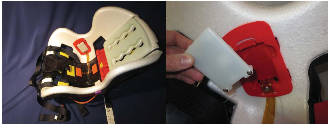
Figure 9: True Fit I-Alert C685 child restraint with cover removed (left), and the removable transmitter module (right). The two switches are the orange rectangular areas shown in the base of the CRS along the midline on either side of the seat bight.
