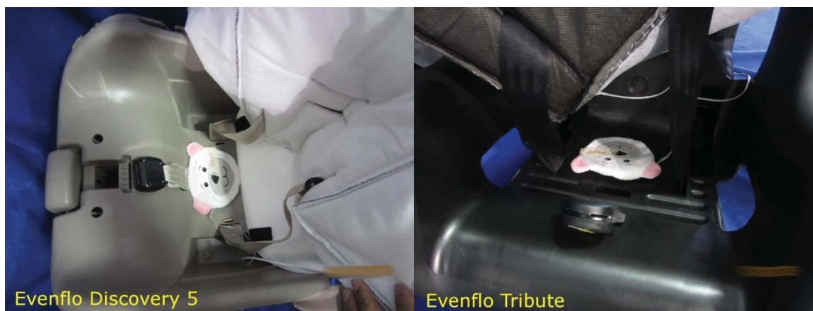
Figure 7: Forget Me Not (bear face-shaped pad) installed in Evenflo Discovery 5 infant carrier (left) and Evenflo Tribute convertible (right) CRS.
