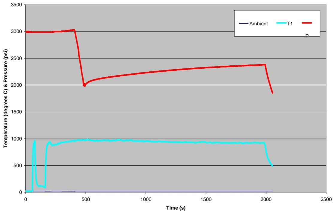
Figure 11 – Temperature/Pressure vs Time profile for epoxy intumescent during 30 minute fire test.
