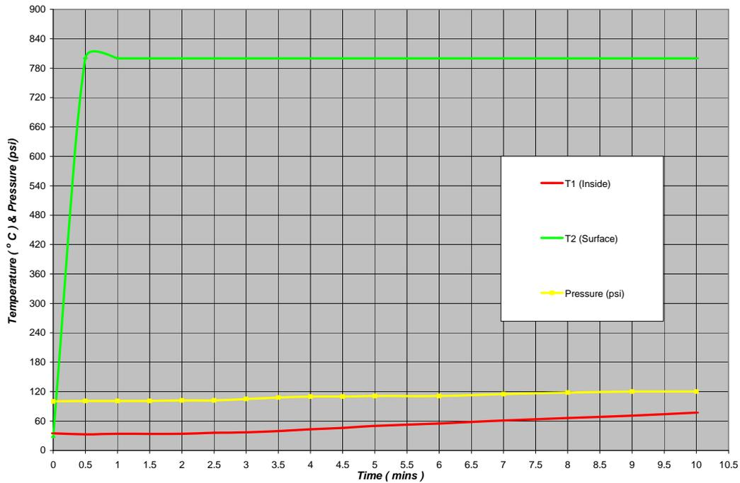
Figure 8 – Change in tank pressure and internal temperature during exposure to 800°C surface temperature
