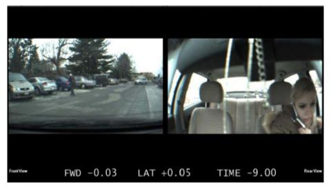
Figure 2. Exterior and Interior Video View Captured by DriveCam Cameras
