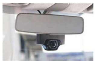
Figure 1. DriveCam Event-Triggered Video Data Recorder
